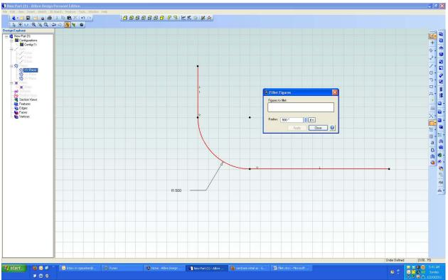
The tool extends the lines as needed to connect to my arc.
