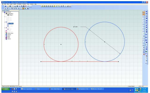
Using the tangent constraint tool, I first click on the horizontal line. This tells the program what I want to *not* move. Next I click on my new circle. The new circle is drawn down to the line and locked to it.
