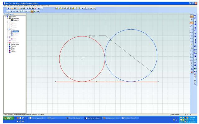
Still using the tangent constraint tool, I click on the original circle to say I want this **not** to move, and then click on my new circle. This causes the new circle to move to the original circle and be locked to it while remaining locked to the line.
