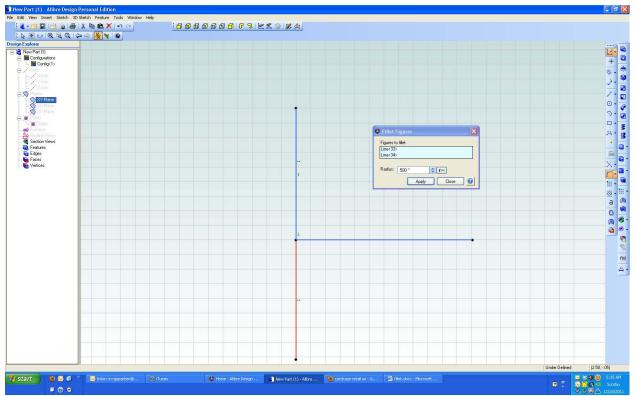
I again select my horizontal and vertical lines from within the fillet tool. But note that the separate vertical line below the horizontal line is red. This means that it has not been selected.
