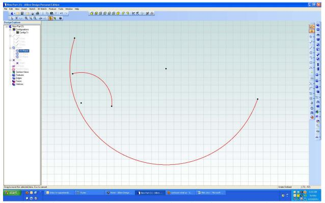
The fillet tool draws an arc between *lines*. Lines don't have to be straight; they must just have two end points and be one dimensional.
