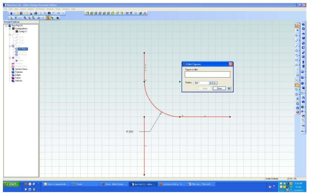
This time my fillet tool does not delete the vertical line below the arc. It is a separate line so is not involved.
