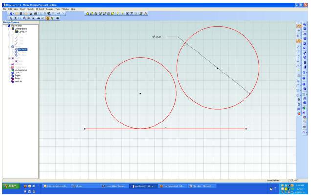
One work-around is to draw a new circle with the desired radius. I must dimension it to lock its size.
