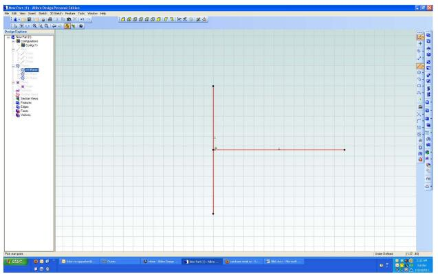
This time I have drawn a T. I want a fillet between the top half of the vertical line and the horizontal line. Alibre assumes that I no longer want the bottom half of the vertical line.
