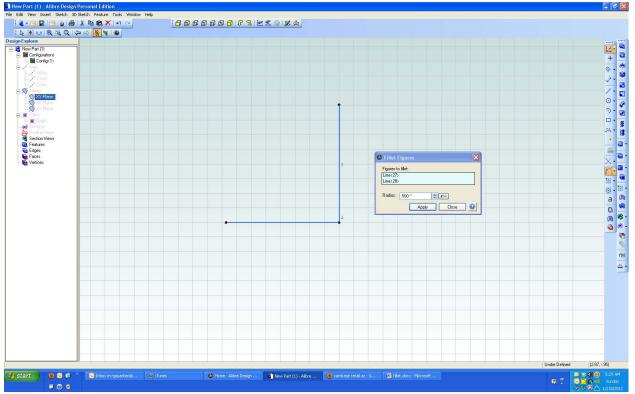
I then brought up the fillet tool and clicked on each line. I'll use the default radius of 0.500". As each line is clicked, it turns from red to blue and its ID is put in the "Figures to fillet" dialog box.
