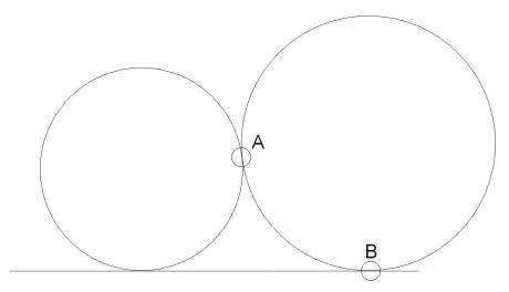
Our larger circle contacts the smaller circle at only one point which is marked A. Our larger circle contacts our line also at only one point which is marked B. The program automatically breaks up our large circle
