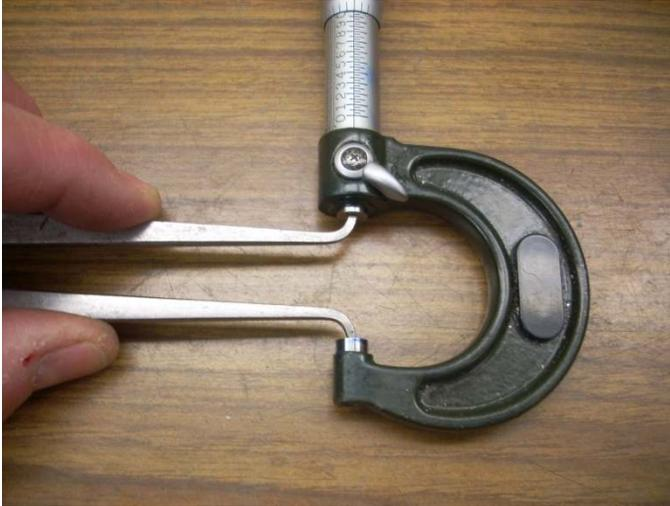
Set your mic to read exactly 0.9000" according to the thimble. Then adjust the inside caliper until it easily slides into the mic with no side play. Be sure to have the caliper on the same plane as the body of the mic. Open the mic to 0.9010" and get a feel for this extra 0.001". Close the mic down to 0.8990" and again get used to how this feels. Repeat the exercise for
