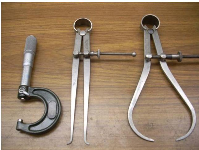
Looking at the three instruments, I would say that it is likely that what is dialed in on the mic will not be effected by setting the inside caliper. Furthermore, the inside caliper error will always be reading large because it
