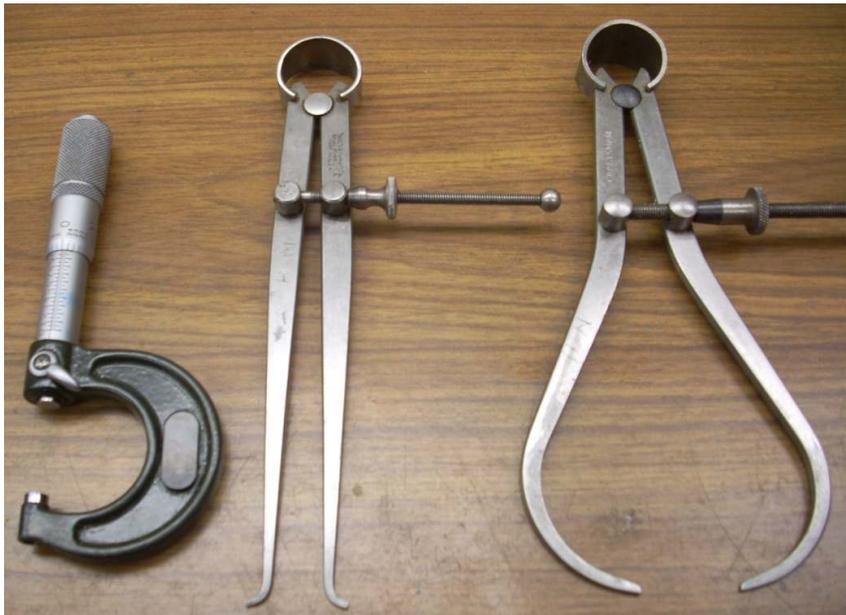
Here we have three measurement instruments that can drive you crazy. On the left is a 1” micrometer. In the middle is an inside caliper. On the right is an outside caliper. In the hands of a machinist with the proper feel, they can do
