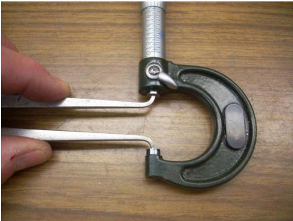
We again start by setting our mic to 0.9000" and then adjust the inside caliper for a sliding fit with no deflection.
