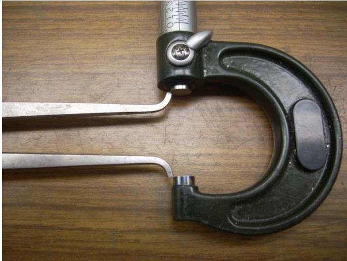
You should be able to start with the inside caliper just off of the mic. Then slide it in and feel a slight drag but no compression of the caliper<sup>3</sup>.
