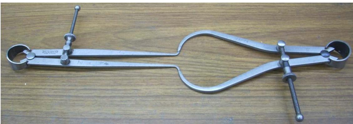
Adjust the outside caliper until it is a nice sliding fit on the inside caliper. If you get confused and adjust the inside caliper, return to the mic to set it again.
