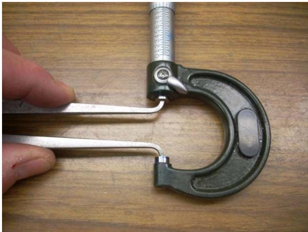
The reading you get on the mic reflects the sum of a number of errors. There was error transferring the mic's opening to the inside caliper. Then we have the error transferring the inside caliper's opening to the outside caliper. This was followed by the error of using the inside caliper to read the outside caliper. And finally, we have the error associated with using the mic to read the inside
