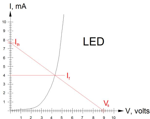
Then draw a line at the level of your desired  $I_f$  extending from the current axis and crossing the LED curve.
