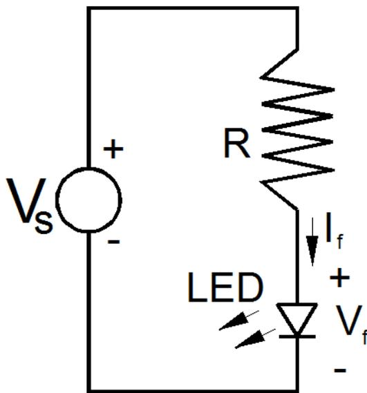
Finding the best limiting resistor to drive a Light Emitting Diode (LED) is a common circuit design task. In many cases, it is good enough to assume a fixed forward voltage,  $V_f$ , and pick a forward current,  $I_f$ . Then use the equation
