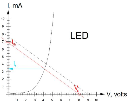
Say  $V_s$  drifted 10% lower. It would move from 9 volts 8.1 volts and the graph would look like this. My new load line (red) has the same slope but is shifted over. It was drawn to cross the volts axis at 8.1 volts and cross the current axis at  $\frac{V_s}{R} = \frac{8.1\text{ volts}}{1.18\text{ K}} = 6.86\text{ mA}$ .
