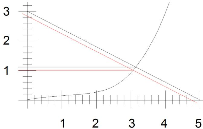
When the supply drifts down to  $5V - 5\% = 5 - 0.25 = 4.75$  volts, our load line move in towards the origin. The new forward current is about 1 mA (red line), a change of 0.15 mA or 15%. So now the forward current error is 3 times that of the supply.
