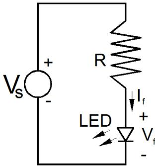
Let's see if this makes sense. We chose a  $V_s$  of 9 volts, an  $I_f$  of 4 mA and got an  $R$  of 1.18K. The voltage drop across the resistor will be  $4\text{ mA} \times 1.18\text{K} = 4.72\text{ volts}$ . This means that the voltage across the LED,  $V_f$ , should be  $9 - 4.72 = 4.28$  volts.
