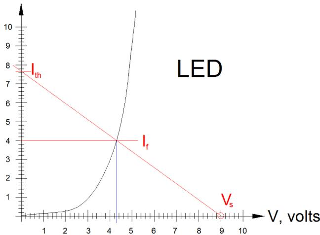
Going back to the graph, I drew a blue line down from the  $I_f$  equal to 4 mA intercept point. You can see that it hits about 4.3 volts on the volts axis.
