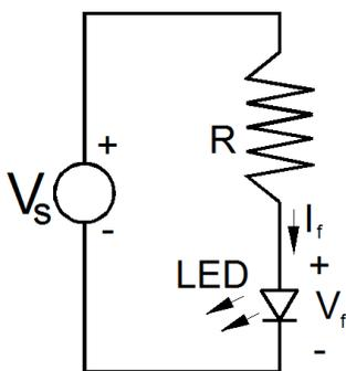
You must choose  $V_s$ , the supply voltage, and  $I_f$ , the forward current in order to find the limiting resistor's value.
