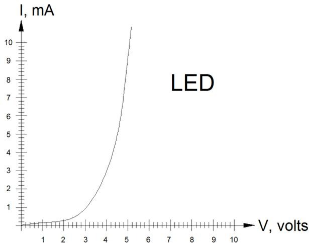
Here is a typical graph showing how the voltage and current vary for a given LED. The shape and values of the curve varies as a function of LED color, ambient temperature, and process used to make it. You can find this graph in your chosen LED's spec sheet.
