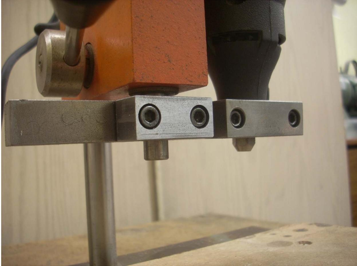
Here is a close up of the two clamping blocks. On the right is my Dremel firmly clamped in place and ready to receive a circuit board type drill. On the left is the rod that moves up and down under the control of the lever. I slide the clamp up the rod to set the maximum height of the drill.
