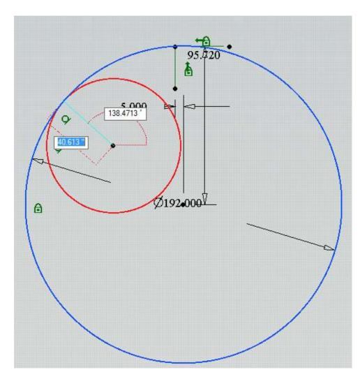
I next drew a reference line from the center of the smaller circle to near the tangent point. When I am close enough to this tangent point, an "X" appears. Then I left clicked the mouse to lock the line in.
