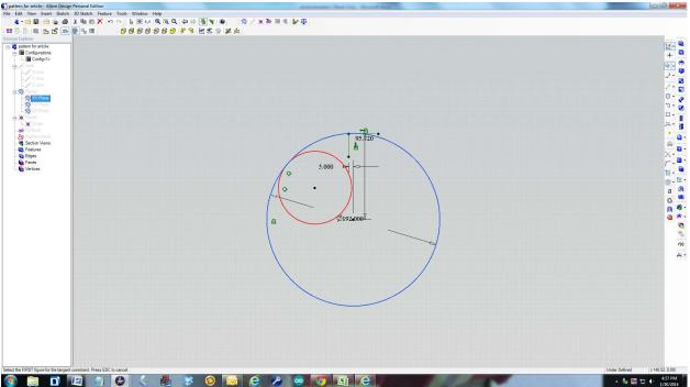
A Tangent Constraint is applied between the two circle. Notice that the larger circle did not move but the smaller circle increased in diameter. The two circles are now tangent. However, this tangent point is not in the correct position.
