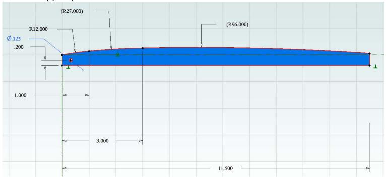
I recently needed to draw a profile that contained three radii. The transition point between radii was specified along with each radius. All tangents at these transition points had to match. Not much to go on but it turned out to be enough information to get the job done.
