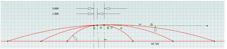
Using the Trim Figure tool, I removed the parts of the circles below the line. Then I removed the arcs that were not need in the final profile. Be very careful when doing this trimming. It is easy to remove the wrong arc and can be tricky to get it back.
