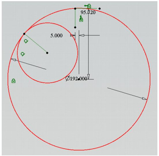
I now have a point on the two circles that marks the tangent. Using the cursor, I am able to slide this point around. The diameter of the second circled is defined. This could have been done at any time after the circle was drawn.
