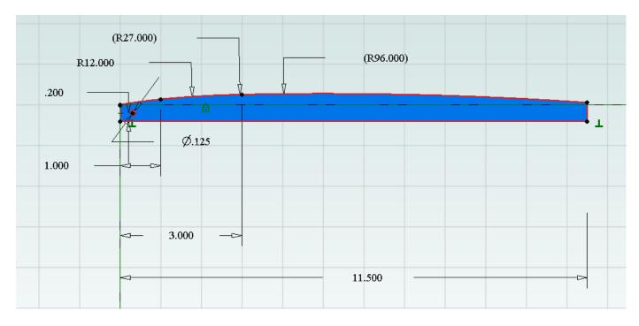
The ends have been trimmed and a small hole added near the origin to assist with installation.
