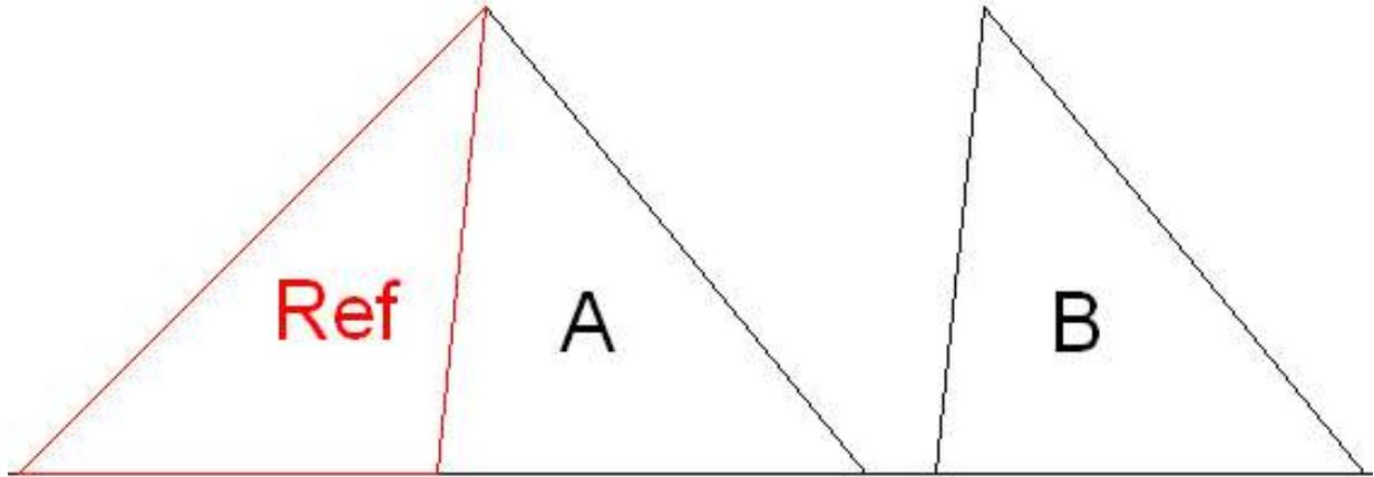
With Ref placed on a straight edge, I will adjust triangle A until it perfectly matches the almost vertical side of Ref. Then I will take triangle B and do the same thing. So now triangle A matches triangle B on its almost vertical side.
