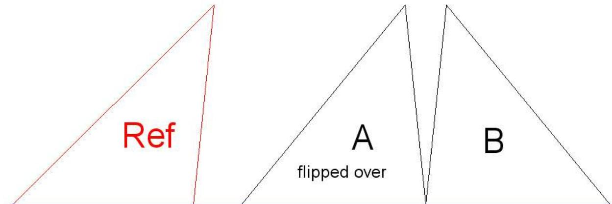
See that gap between A and B? It wouldn't be there if Ref was a perfect right triangle. So although we don't have a right triangle, we can tell when we get one. As with the challenge of making a precision straight edge, the gap at any point equals twice the error in Ref.
