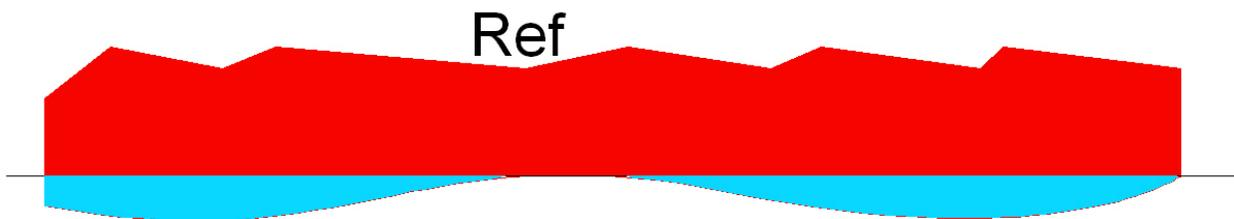
But how much do I remove? It turns out the separation between flipped A and B at any point along this edge equal twice the amount the Reference edge is over the line.
