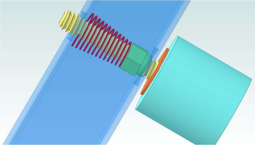
I was contacted by Bill Libecap on an idea that employed a spring to retract the fastener plus keep it from flopping around when disengaged. After a bit of discussion, we came up with this modification to the design. A conical spring has been added.
