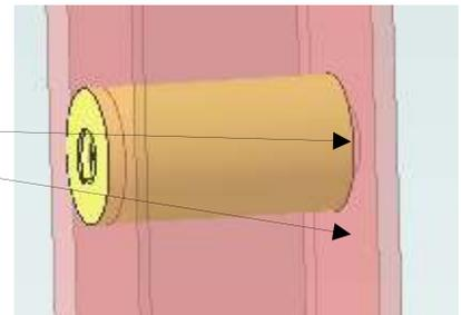
This arrangement solves two problems. The threaded material is ample compared to just trying to thread the wall of the tubing.
