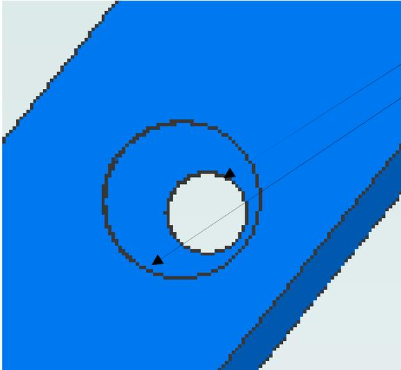
The tubing that will accept the CRS cylinder was first drilled through with an F drill and then one face was opened out with a 1/2" drill. Deburring of the smaller hole was essential.
