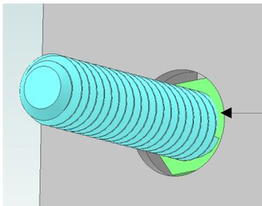
The  $\frac{1}{4}$ " diameter threaded rod passes through the  $\frac{3}{8}$ " hole to give  $\pm \frac{1}{16}$ " of free movement.
