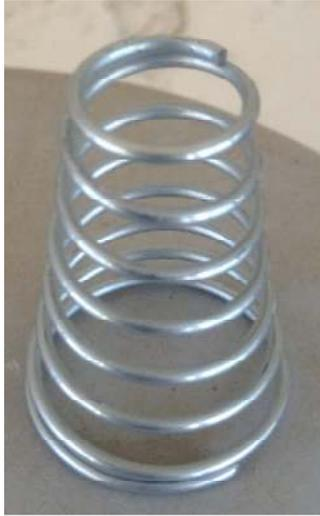
I bought this spring at Ace Hardware. The small end has an ID of about 3/8" and the large end has an OD of about 3/4". The overall length is about 1" uncompressed.
