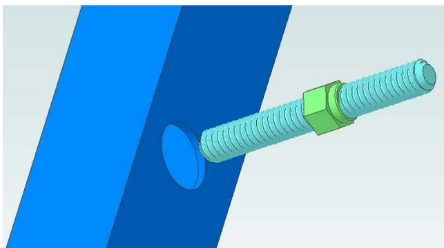
The rod/nut assembly is then fed into the tubing through the 1/2" hole. Note that the bottom of the nut is towards the tubing.
