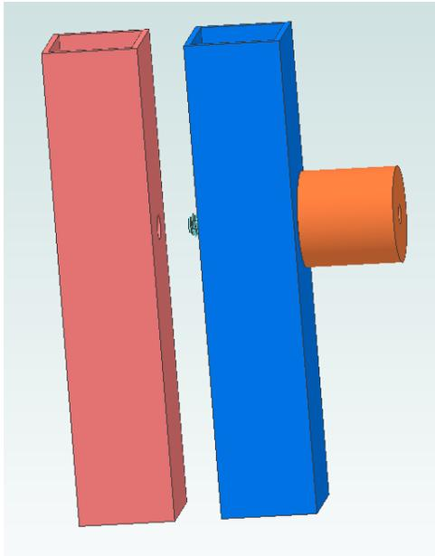
I needed to be able to fasten two pieces of 16 gage 1" steel tubing together. There shall be no loose parts and no tools required. A misalignment of  $\pm 1/16$ " shall be tolerated. The fastener thread is  $1/4$ -20 and 4 to 5 threads shall engage.
