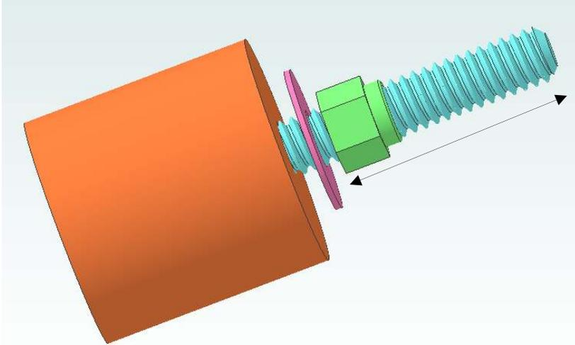
The male part of the fastener consists of the knob, a washer, a self locking nut, and the threaded rod. The ends of the rod are generously beveled.
