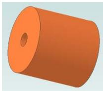
The 1" diameter 1" long knob is made of 6061 aluminum and is drilled and tapped 1/4-20 almost all the way through. See <http://rick.sparber.org/tfs.pdf> for details.
