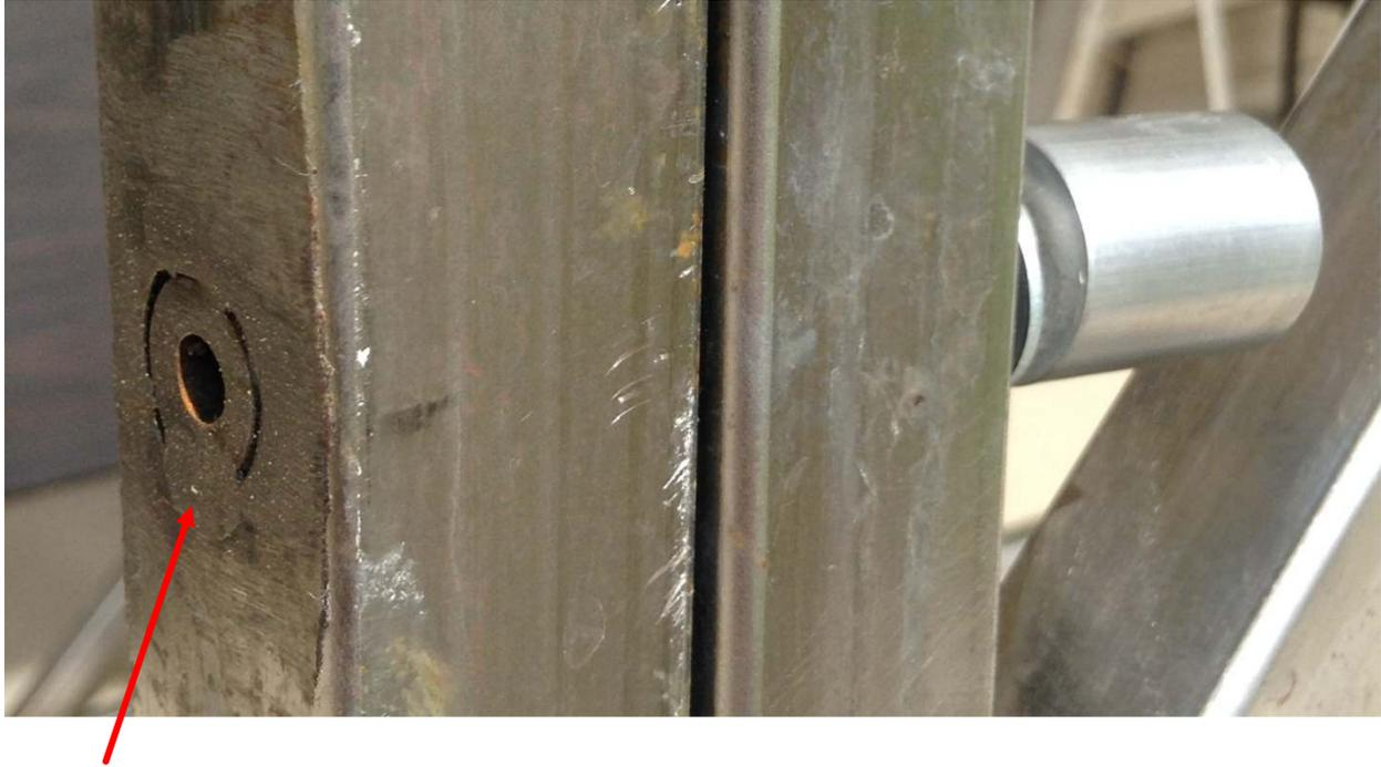
The threaded CRS cylinder was tacked in place and then the weldment ground flat. We only need to insure that the cylinder does not rotate or fall out during threading and when not in use.
