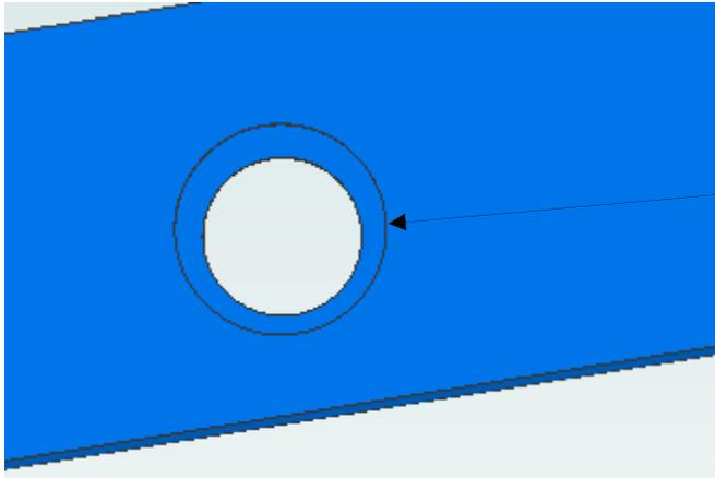
The tube that will accept the male part of the fastener is first drilled  $\frac{3}{8}$ " through. Then the outer face is drilled  $\frac{1}{2}$ ".
