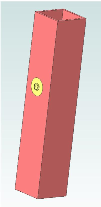
I did a lot of MIG welding on this tubing so it was a simple matter to also tack weld the CRS cylinders to the faces of the tubing.
