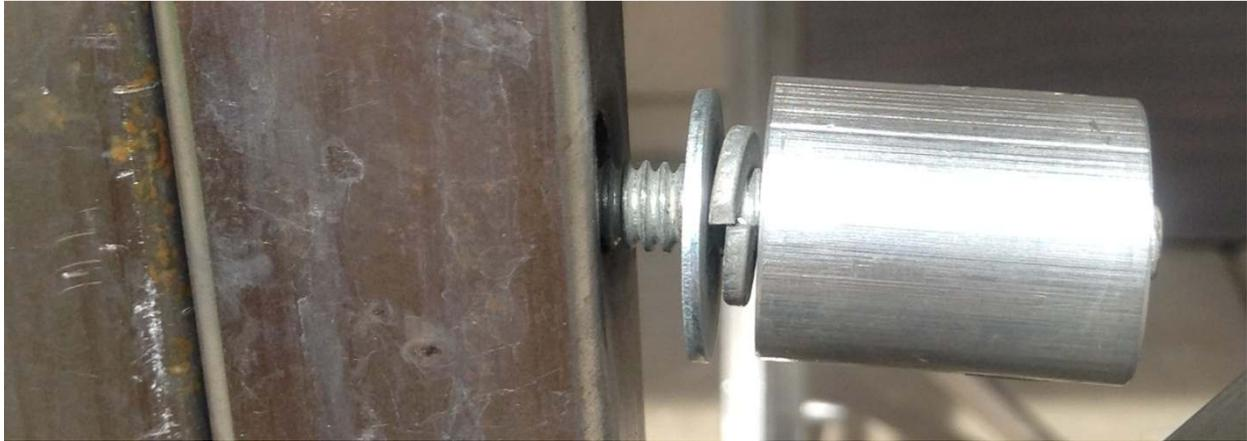
I have added a spring washer between the knob and the regular washer for this application. The knob was intentionally left smooth because very little force is required. Compression of the spring washer is all we need.
