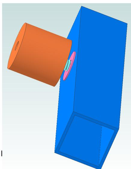
The aluminum knob goes on next but this is a thermal fit. The hole in the knob is first heated with a MAPP<sup>®</sup> gas torch for 20 seconds before being tightly screwed into place.
