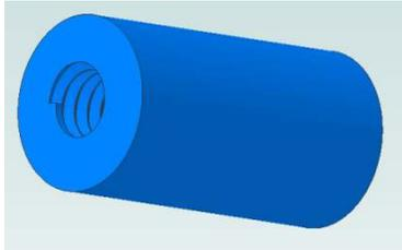
The female side of the fastener is a piece of 1/2" diameter CRS drilled and tapped 1/4-20. Its length equals the outside width of the tubing minus one wall thickness.
