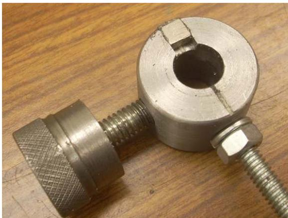
The trick is a milled slot in the side of the collar with a tiny neodymium magnet glued in place. This magnet is 1/16" x 1/4" x 1/4" and surprisingly strong. The stop can be held in any position within about 45° of vertical. Yet the magnet is not strong enough to collect swarf.
