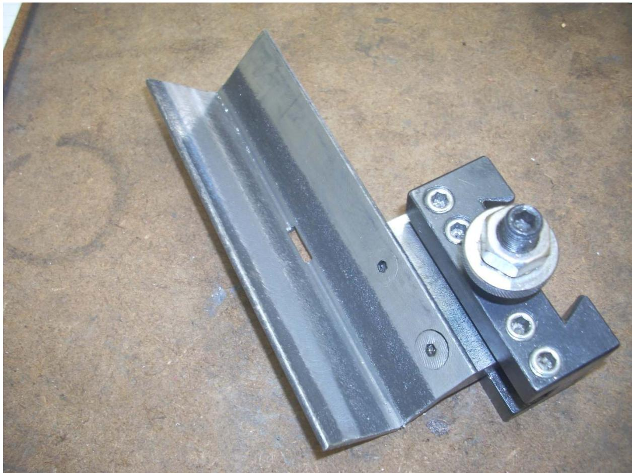
I did have to mill out the corner of the angle stock to remove the inside fillet. But otherwise, there really isn't much to the design. In hindsight, I wish I had set the support block lower because large blocks to be beveled hit the tool holder as they slide near it. Not a big problem since I just lean them towards the headstock.
