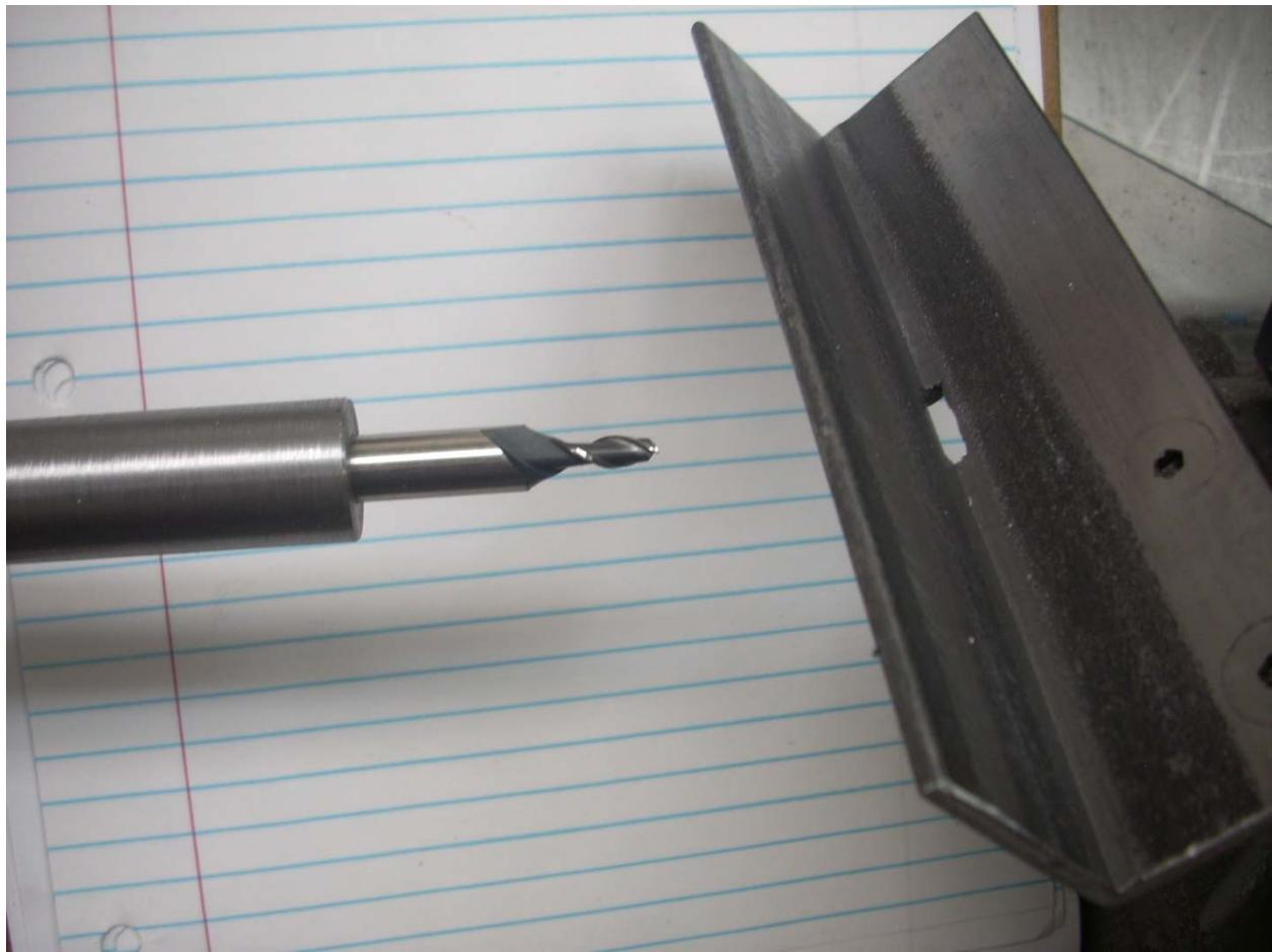
A 1/4" end mill is held in the end mill holder some distance from a Jacobs chuck on my lathe<sup>3</sup>. A piece of angle stock is supported by my quick change tool post. There is a slot in the bottom of the angle stock that permits the end mill to just slightly enter the bottom. I am shooting for about a 0.01" wide flat on the corner of the block being deburred.
