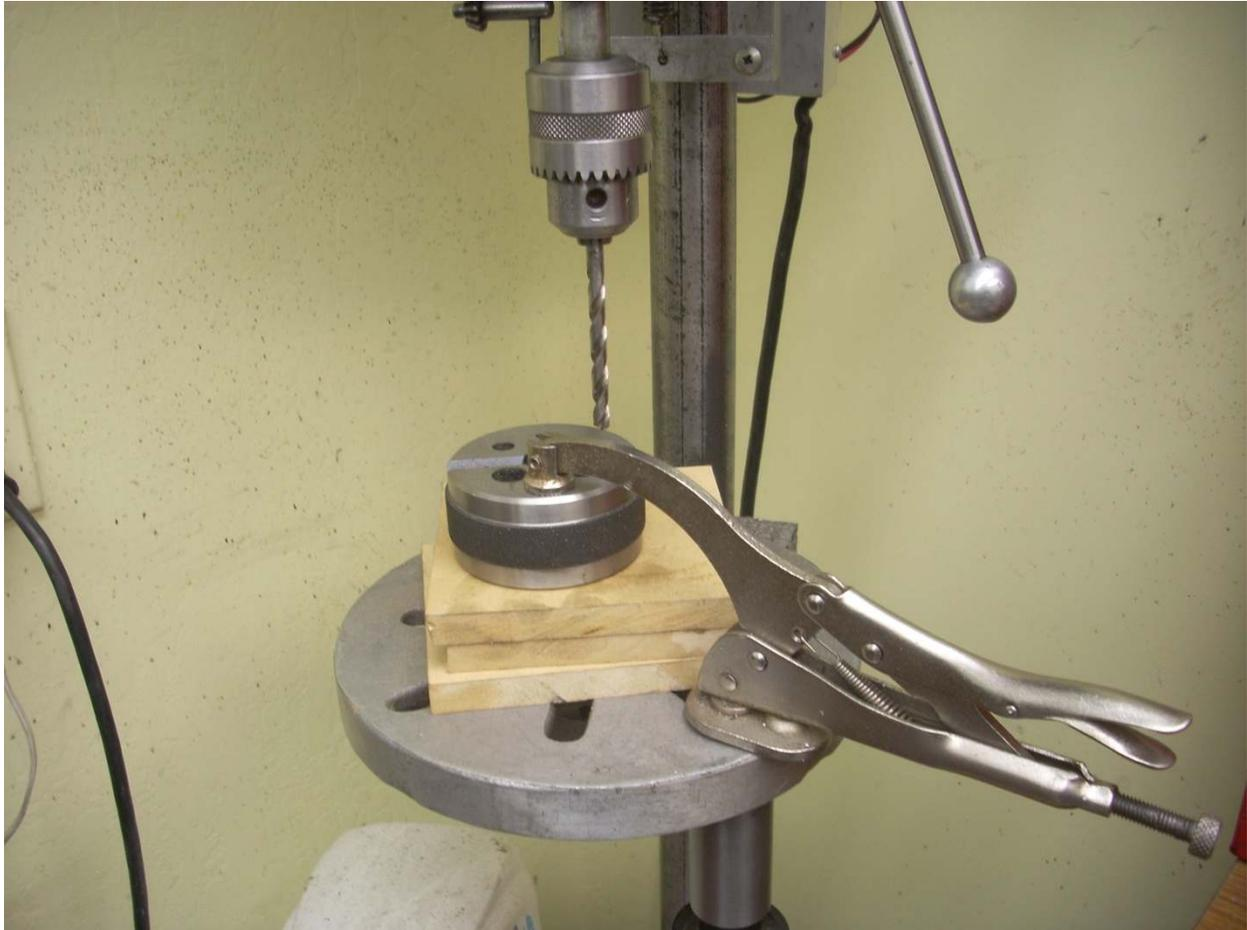
The bench block is also useful on my drill press. Here I have installed a 1/4" drill in the chuck. Then I fed down until the drill entered the 1/4" hole in the V.
