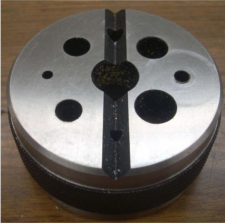
The top surface has been ground flat with respect to the bottom. Use it when you need to raise something up while keeping it parallel to the support surface.
