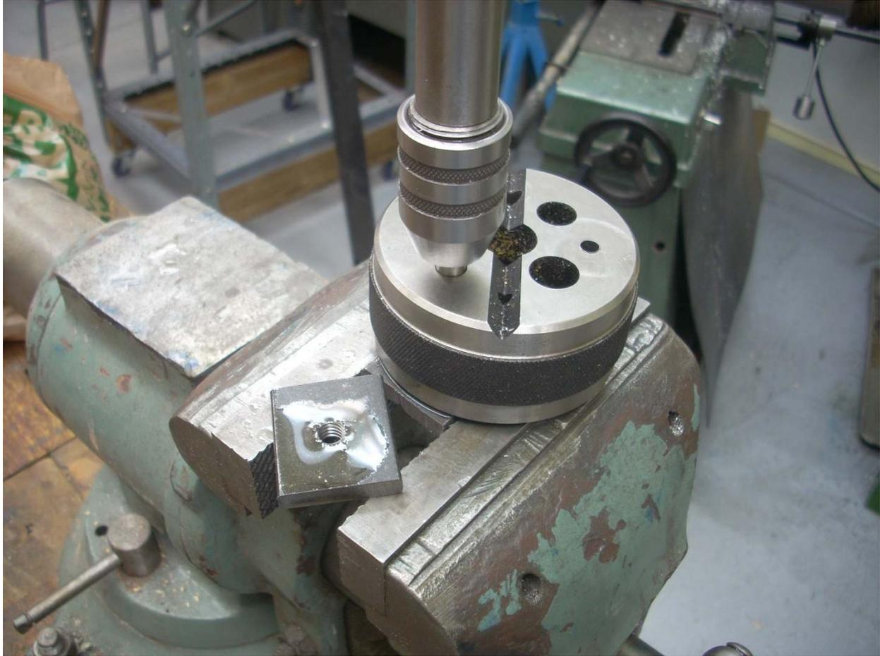
I have used my bench block to align the tap with the jaws of the vise. You see a finished part next to the set up. Using the bench block in this way is simple, quick, and gives good results. Without the bench block, it is easy to start the tap at an angle and have it bind up as you feed in.
