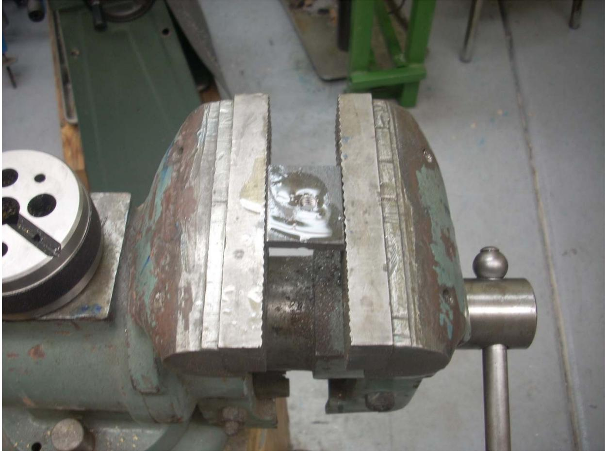
I wanted to hand tap a hole in this piece of steel. Sure I could set up my mill and install my tapping head, but it is hardly worth the trouble. The tap must go in reasonably straight but I didn't need super precision here. So I put the steel into my vise jaws so it was aligned with the top of the vise jaws.
