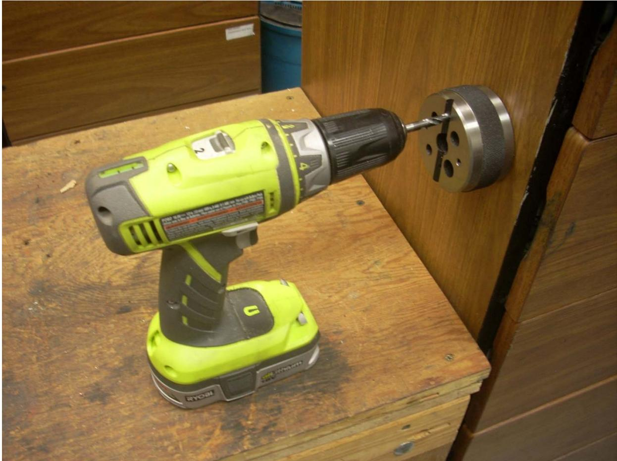
This alignment is particularly helpful when drilling through vertical surfaces or overhead. The knurled perimeter and weight of the bench block give you a solid grip and a good feel.
