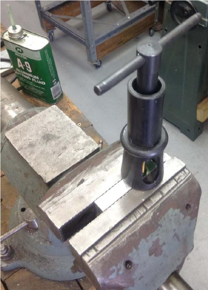
The block went into my vise with the side were flush with the top of the jaws. I then squirted a little cutting fluid into the hole to make tapping easier.
