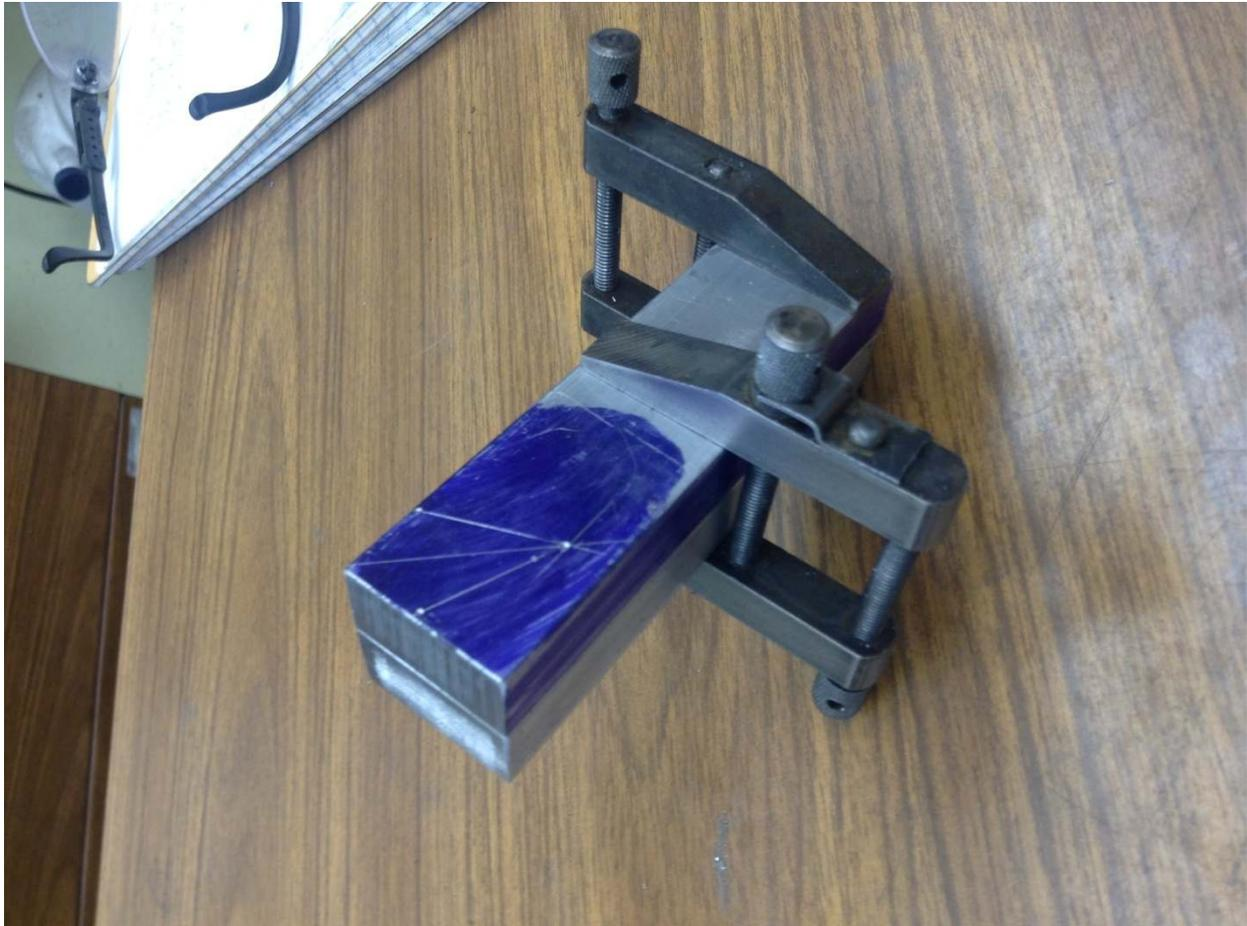
The second workpiece was clamped to the first one. By using two clamps, I could move one at a time and not lose alignment.
