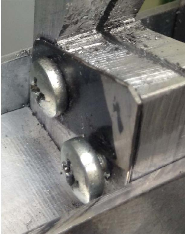
I used a tap, so ran a #36 drill in to form a hole that flanked the bottom edge of the hacksaw blade. The idea is to prevent the blade from sliding away from the bolt resting in the V. Note that this second bolt was not tightened all the way into the thread plate. When I did that, it pushed the hacksaw blade up. As shown, the hacksaw blade is solidly mounted.
