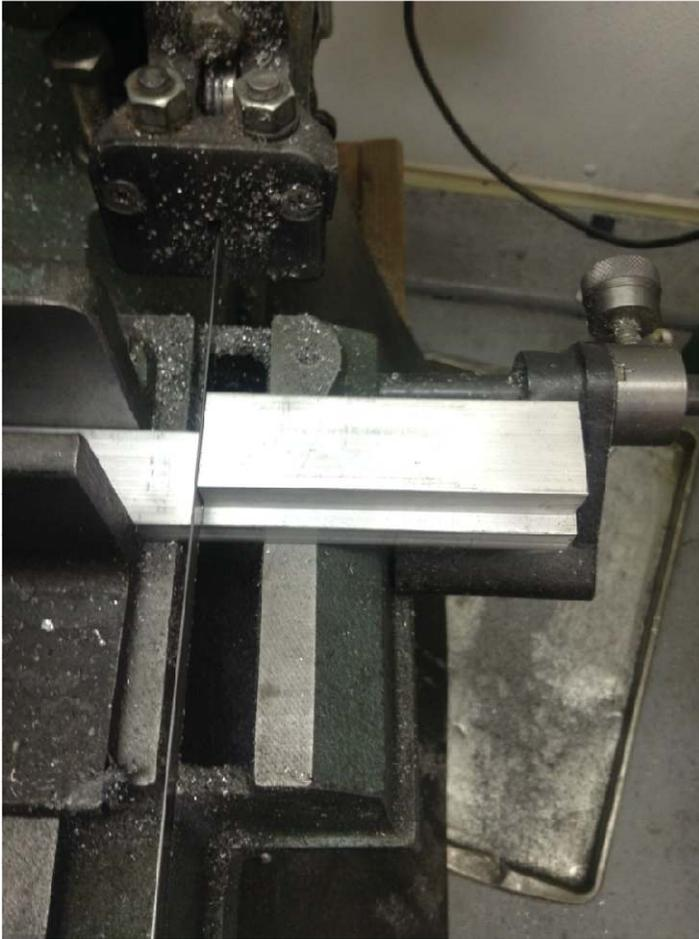
Using  $\frac{1}{2}$ " x 1" aluminum bar stock, I cut a piece 3.5" long. Then I used that piece as a measure to set the distance for a second piece. Note that the workpiece is laying flat on the vise ways. On my bandsaw, cutting it this way reduces the tendency for the blade to wander.
