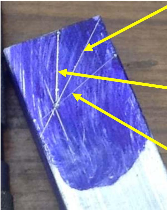
Using the square's 45° end, draw a line from a corner to the far side of the workpiece. Then scribe a line  $\frac{1}{4}$ " from that far side that intersects the diagonal line. Use the punch to mark this point. It will be the bottom of the V.
