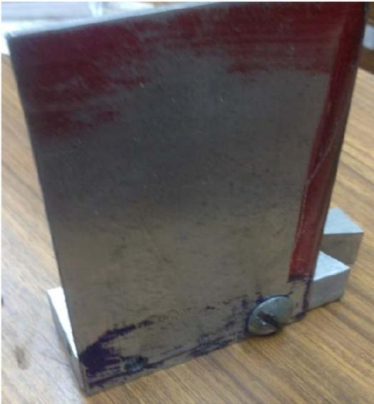
The clamp was then removed and I ran a bolt through the side plate and into the threaded hole in the block. With the end of the block resting on the table and the plate's bottom edge also resting on the table, I tightened the screw. This insures proper alignment of the plate and block on the bottom.
