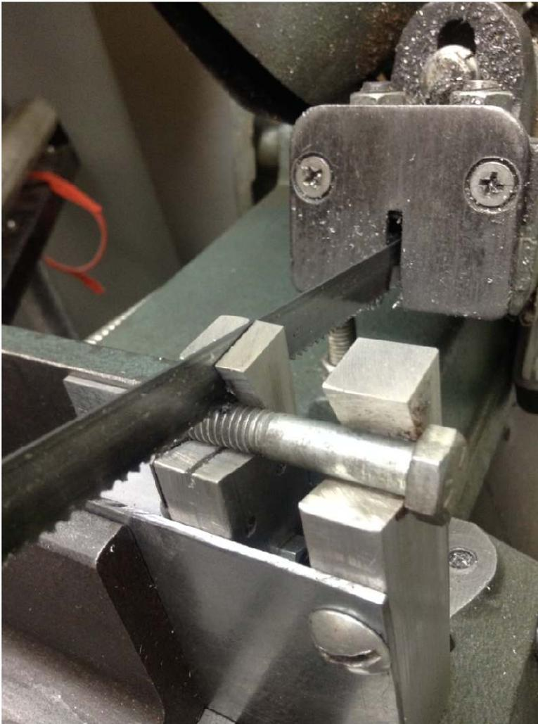
This fixture evolved from a previous design that only handled 1/4-20 bolts. It can now handle bolts 1/2" in diameter and smaller both in metric and English. It also references the underside of the head to set overall length.
