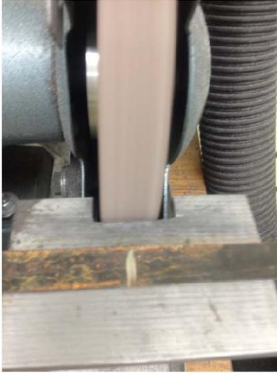
I didn't need the entire length so used my grinding wheel to score both faces about 2" from the end. I did preserve the rounded end and mounting hole. It then easily snaps off.
