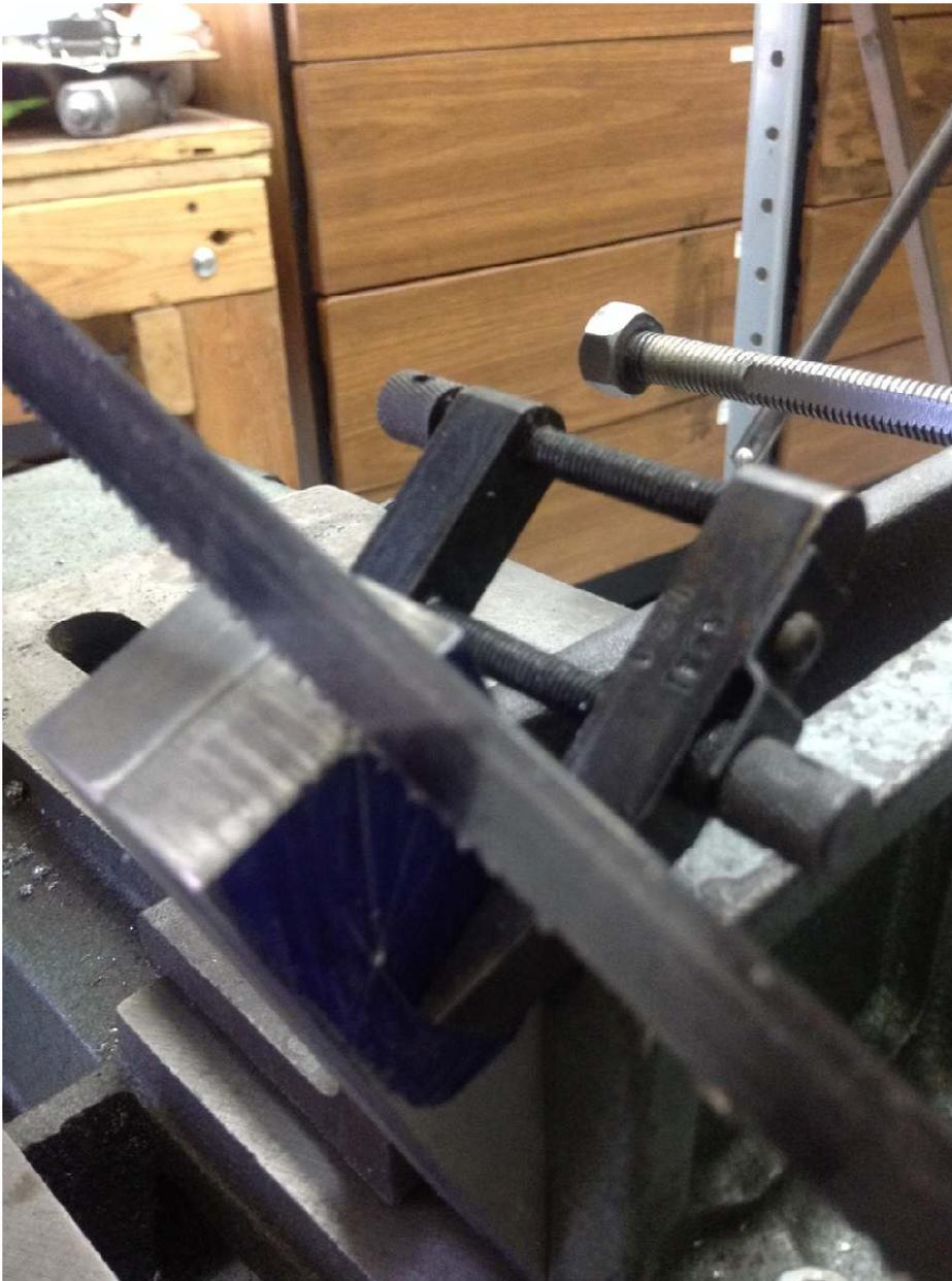
The two work pieces were placed in the band saw's vise such that the first line could be cut. The punch marks were facing the pivot of the saw.
