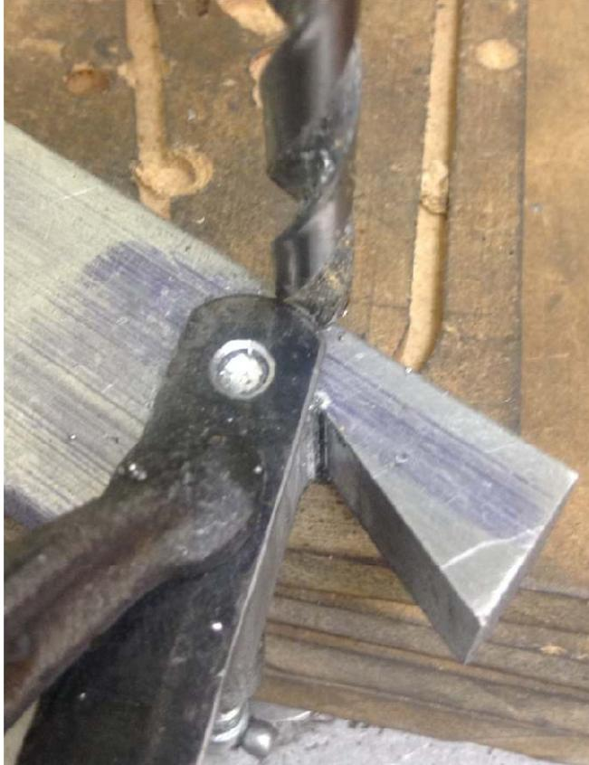
Selected a drill bit who's end snugly fits through the hole in the hacksaw blade. Drill in enough to form a small cone.
