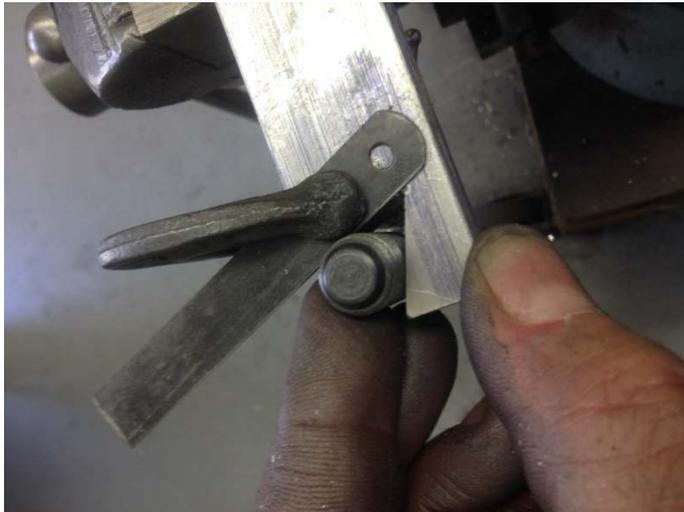
I repeated the process with a  $\frac{1}{2}$ -13 bolt or hold down stud. Rechecked the position with the  $\frac{1}{4}$ -20. When satisfied, tightened the clamp.
