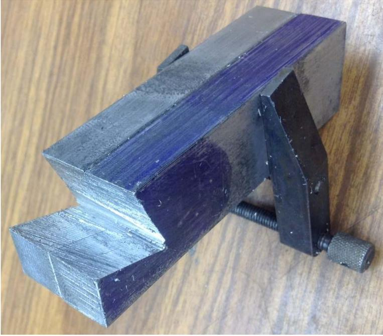
I then had two work pieces with identical V cuts in them. You could smooth the surfaces with a file if you like but take care not to open out the bottom of the V.
