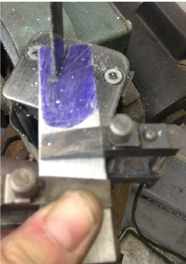
The work pieces were removed from the saw's vise and I freehand cut to the punch mark.
