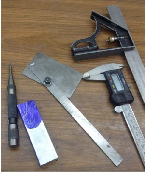
The V was cut next. I used a square, a digital caliper, a protractor, and a spring loaded punch to mark out where to cut. A steel rule could be used in place of the caliper. Accuracy is not that important here.
