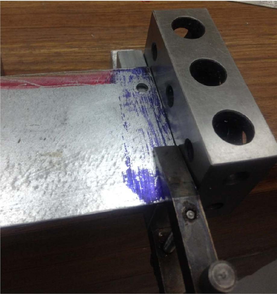
I used a block of steel to help me align the first side plate with the face of the right support block. A clamp was then applied to hold that position.
