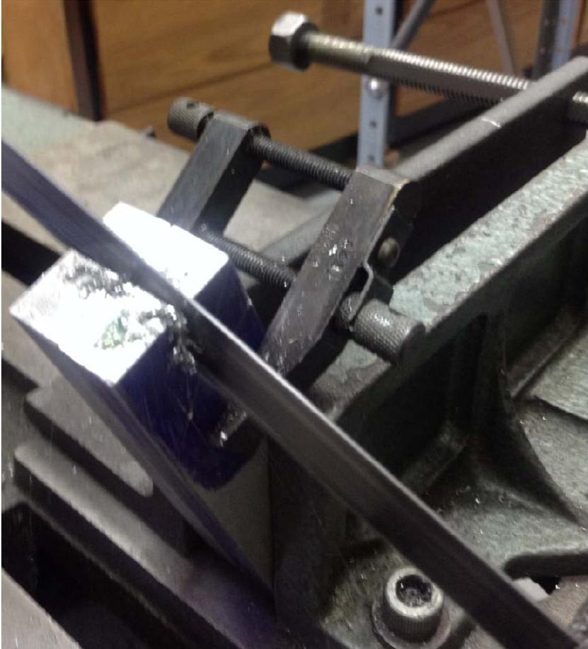
I cut through both work pieces until the blade reaches the lower punch mark.
