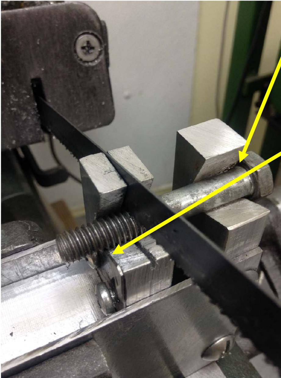
Here you can see the underside of the bolt head snug against the right face of the outer V support.
