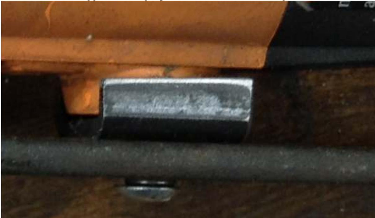
I through drilled the bar and drilled and tapped 10-24 into the channel.
