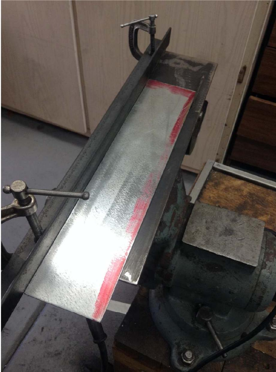
I needed to cut 10 gage steel into a strip 2.5" wide. With the help of a piece of angle stock and two small C clamps, I built a fence. Then the stock was fed into the abrasive wheel just like on my table saw.
