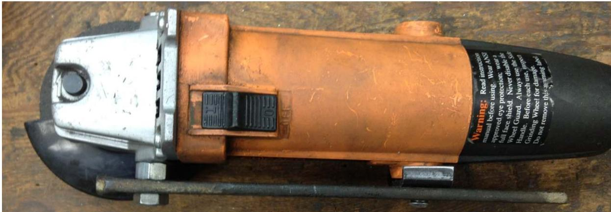
After the article was published, John Herrmann suggested that I capture the lower boss in the support bar to prevent the grinder from pivoting. The bar is too narrow but Brian Lamb suggested using a piece of channel. Worked great!
