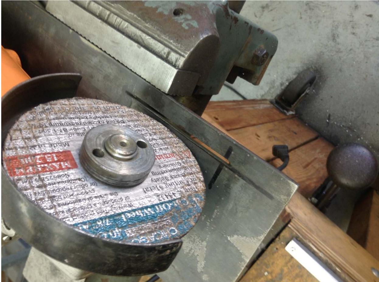
Clamp the plate into a large vise or over the edge of your work bench. Draw a line with a marker about  $\frac{1}{2}$ " from the side edge and about 1" from the end. Then, holding the abrasive wheel as close to parallel to the edge as possible, carefully plunge cut through the plate.
