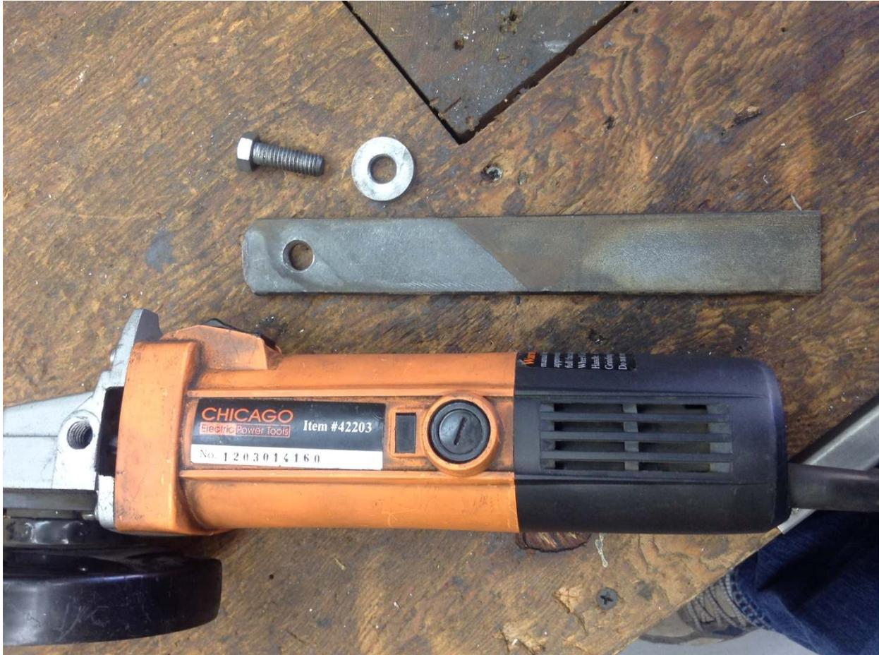
I then raided my scrap pile for a piece of steel bar  $\frac{1}{4}$ " thick, 1" wide, and about 7" long. It happened to have a hole in one end so all I needed to do was use it. I also found a  $\frac{1}{4}$ " thick homemade aluminum washer to raise the bar so it was roughly even with the top of the lower motor brush boss.
