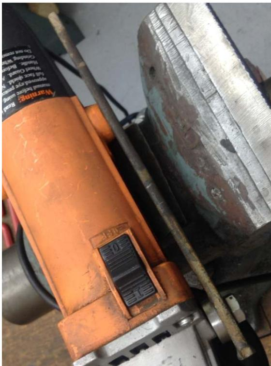
Here is a side view showing how the washer offsets the bar so it is even with the lower boss. With the bolt tight, the assemble is solid.
