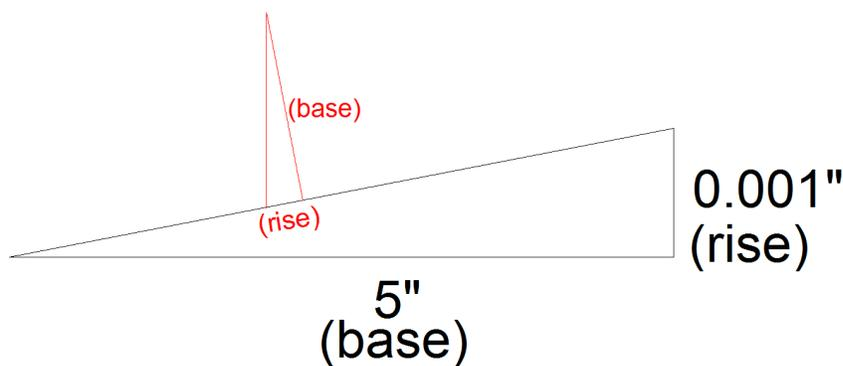
The line marked "base" on my red right triangle represents what the end mill will cut. Note that its rise and base will be proportional to what was measured during tramping.
