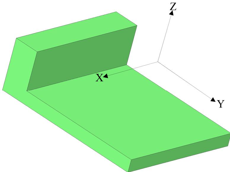
My ideal vise includes a vertical face and a horizontal face. It can be clamped to an ideal milling machine such that the vertical face is parallel to the XZ plane and the horizontal face is parallel to the XY plane.
