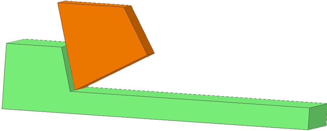
The resulting work piece looks rather sorry. I made two cuts which are both out of square. The top face forms a  $75^\circ$  angle with the face against the fixed jaw. Comparing this freshly cut face with the one nearest the vise ways, I see an angle of  $30^\circ$  rather than being parallel.
