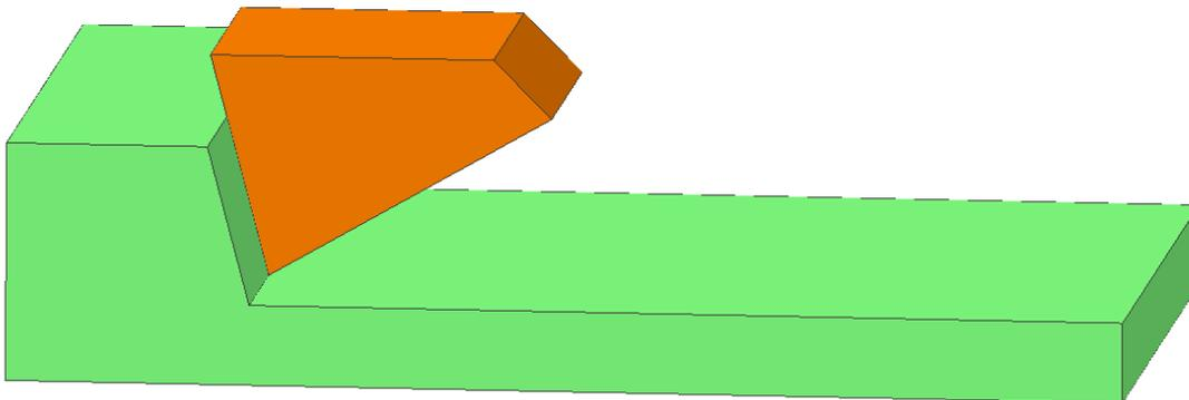
The freshly cut face is then rotated so it is against my fixed jaw. I use my end mill to cut the top true to the XY plane.
