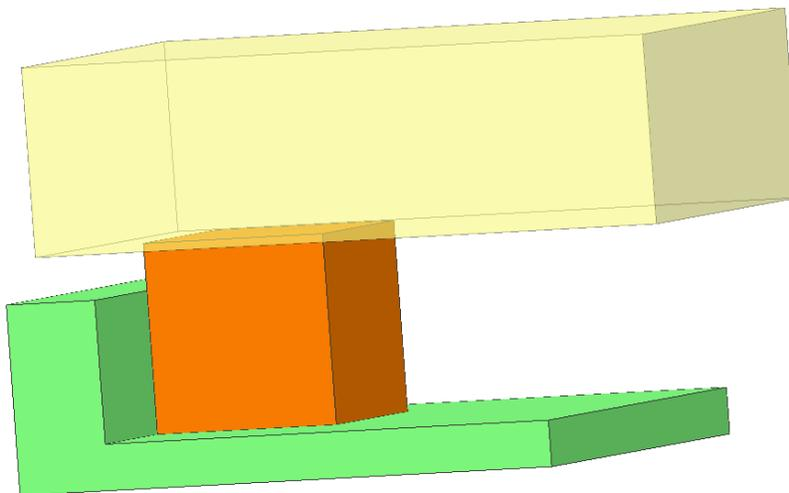
I have added a work piece that is perfectly flat and square on two sides. These sides are in contact with the fixed jaw's vertical surface and the vise way's horizontal surface. A tiny bit of this work piece is within the yellow space. When the end mill is moved over the top of the work piece, the top surface will be cut exactly perpendicular to the vertical jaw and parallel to the vise ways.
