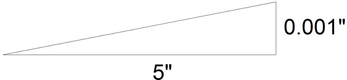
This means my cutter is tilted in the YZ plane by a slope of  $\frac{0.001''}{5''}$  which is an angle of  $\tan^{-1}\left(\frac{0.001''}{5''}\right) = 0.011^\circ$
