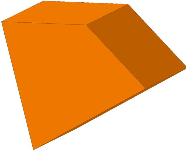
The work piece is now complete. Given an error in my fixed jaw of  $15^\circ$  over  $90^\circ$  ( $= 105^\circ$ ), adjacent faces are at either  $15^\circ$  under ( $= 75^\circ$ ) or over  $90^\circ$  ( $= 105^\circ$ ). Opposite faces are at  $30^\circ$ .
