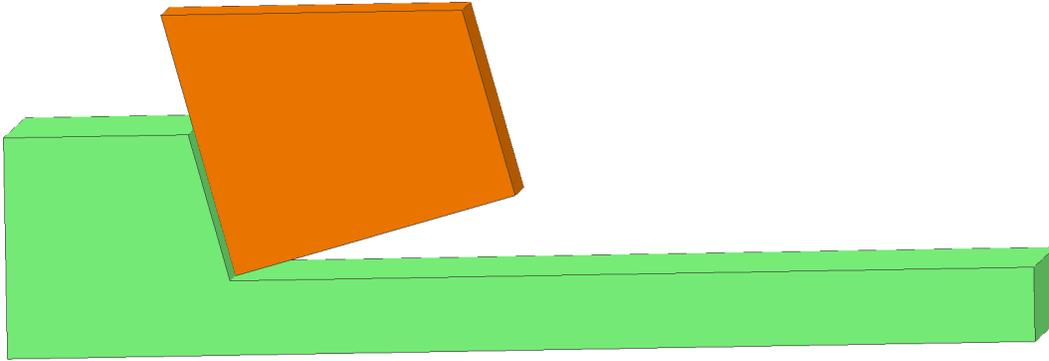
The face I just cut forms an angle with the face against the fixed jaw that is  $15^\circ$  less than  $90^\circ$  ( $= 75^\circ$ ).
