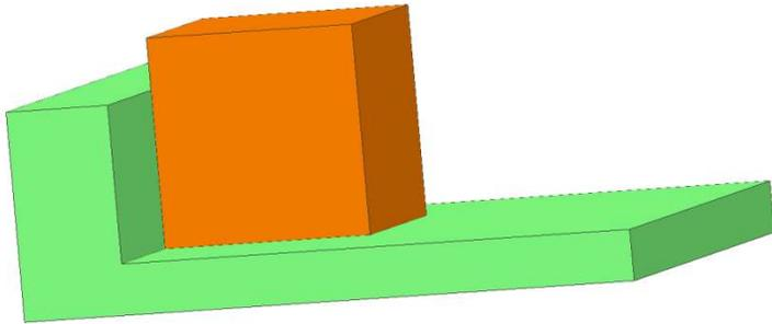
My freshly machined work piece now has three adjacent faces that are perpendicular. I rotate the block so the top face is against my fixed jaw. With another pass of the end mill, all four faces will be perpendicular to each other.
