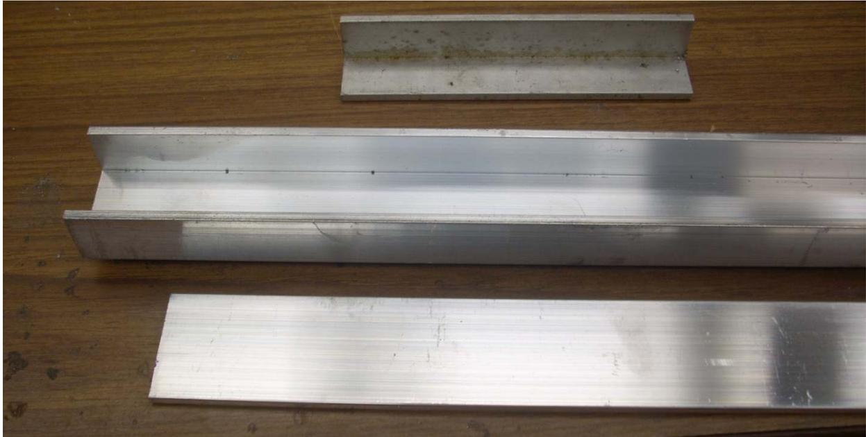
I started with some angle which was used for the ends, the channel which is the body, and the plate which is the top.
