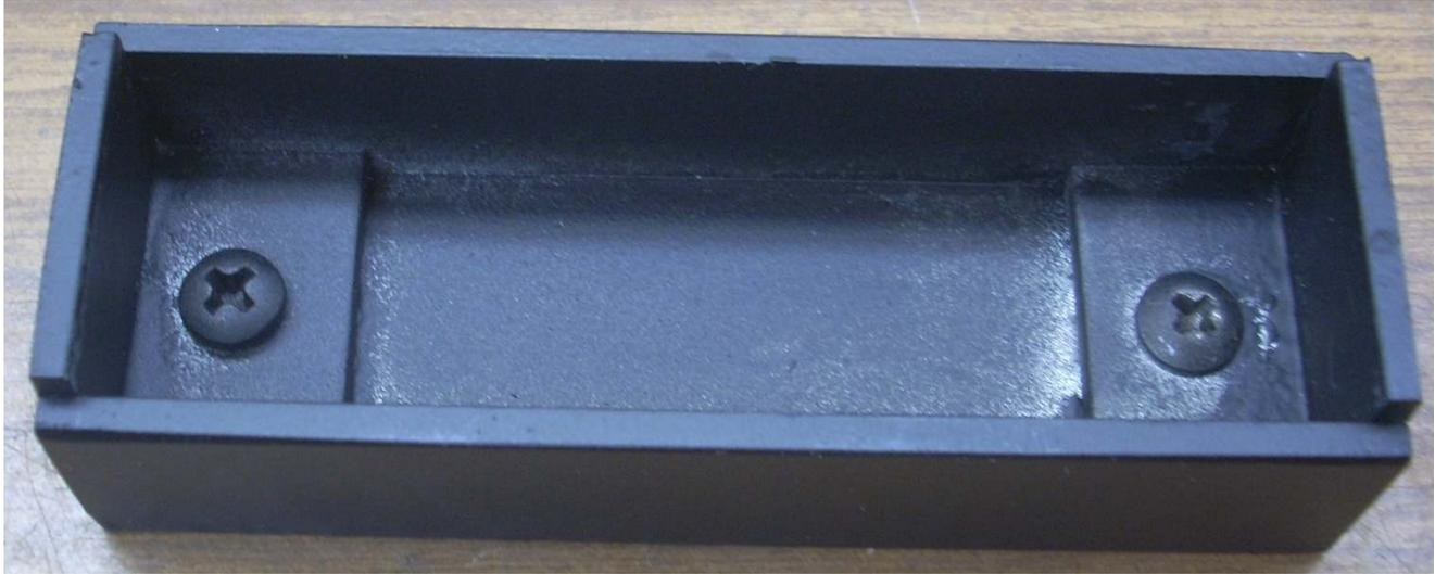
The screw on the right is 6-32. The screw on the left was supposed to be 6-32 too but I accidentally ran my clearance drill through the channel. The easiest recovery was to go up to an 8-32. After the screws were set, I placed the box on my belt sander and made them flush.
