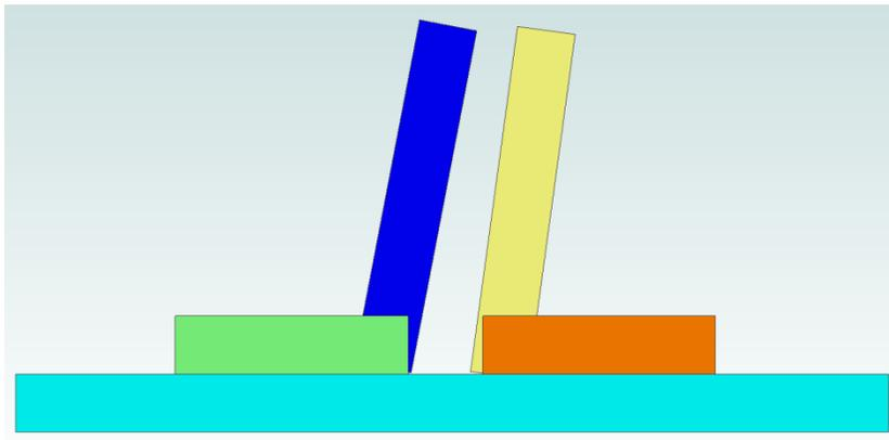
The yellow blade square we wish to set true is put up against a blue blade square of unknown accuracy. In this exaggerated view, they are both off in the same direction but neither is near true.
