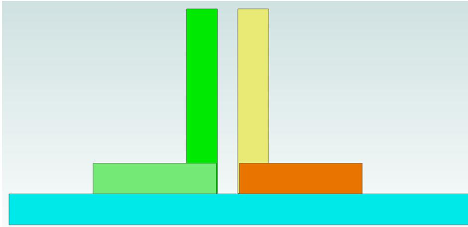
My green reference square is used to set the angle of my yellow blade. The reference square is then carefully placed back in a safe place for future testing. I never use it for
