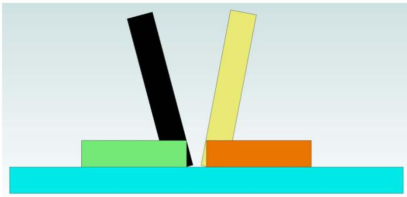
When we flip around the black blade and put it up against the yellow blade, there is a gap. The angle formed by these two blades is twice the difference between the blade angle and true vertical. We move both blades roughly the same
