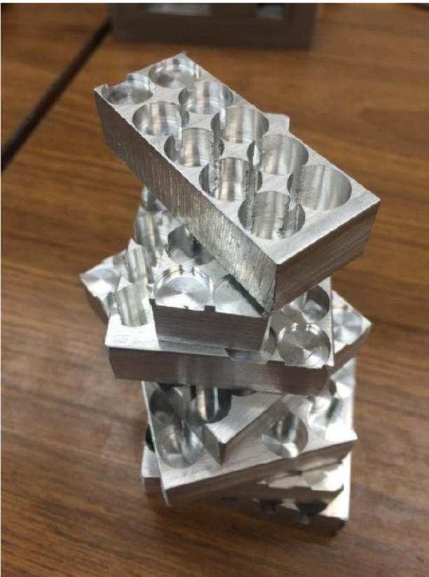
Each set of 10 holes represents one test cycle and produces one data point.
