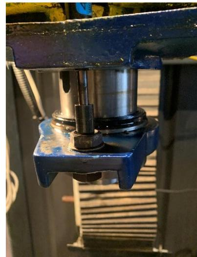
It provides about 100mm of stroke on the spindle under the cylinder pressure. Honestly I had no confidence using a slot drill/ uni mill before but with this mod it has completely changed. I have done one small job & a fairly large job last couple of days and it seems to have done the trick.
