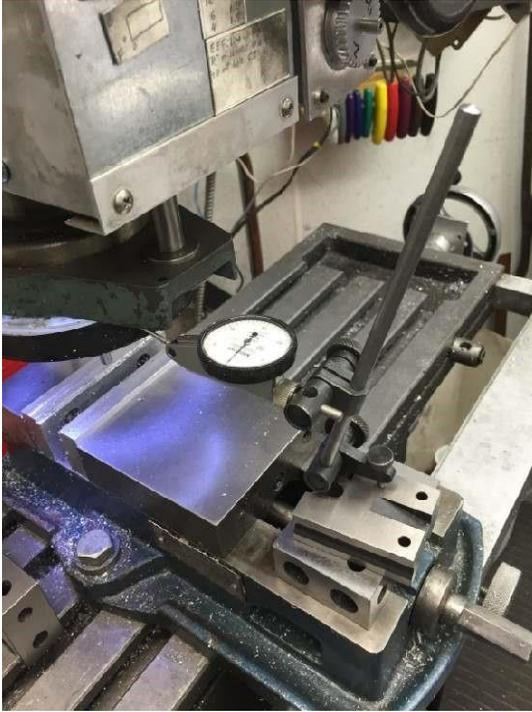
I can directly measure this backlash by using a finger Dial Test Indicator (DTI). The DTI is supported on the table and the finger is resting on the underside of the quill. Using just finger pressure, I can raise the quill a few thousandths of an inch.
