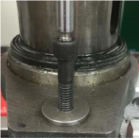
The piston's end sits in the top of a Socket Head Cap Screw 5/16-18 bolt which is threaded into a piece of cold rolled steel.
