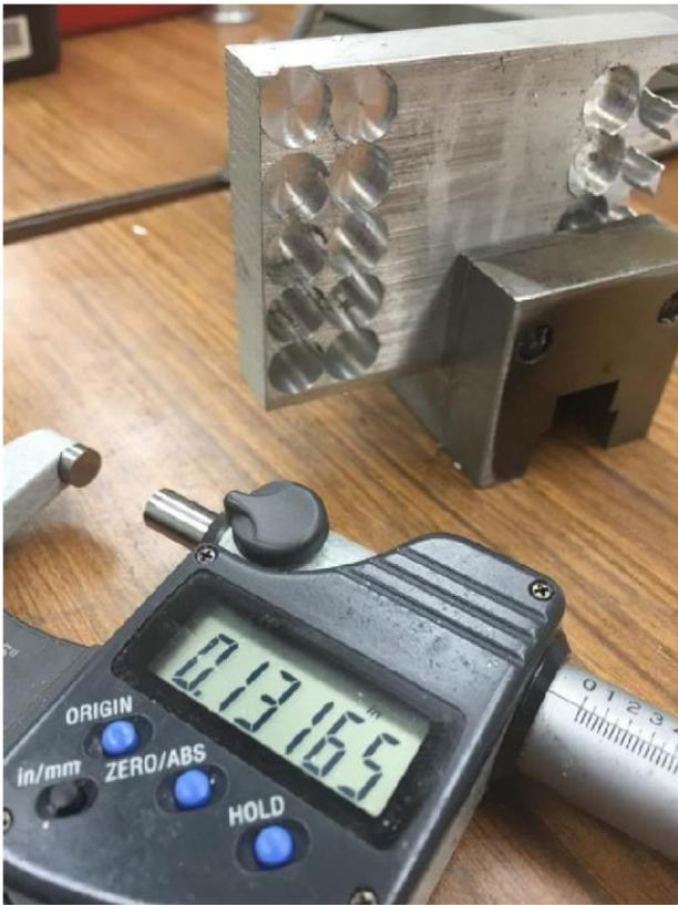
My dynamic test consisted of milling a series of progressively deeper holes in a block of 6061 aluminum. The first hole was approximately 0.01 inches deep. It was my reference depth. I zero my mic in this hole. The second hole was cut 0.1000 DRO inches deeper than my reference. The third hole was cut 0.2000 DRO inches deeper than my reference. The fourth hole was 0.3000 DRO inches deeper than my reference.
