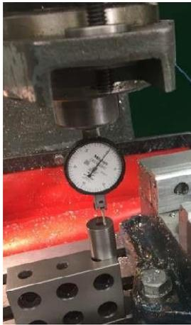
When I put down a spacer block "B" inches thick, I read a thickness of "A" DRO inches.
