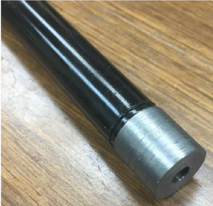
I drilled out a  $\frac{3}{4}$ " length of CRS using a #1 drill. It was then possible to screw the metric stud on securely.
