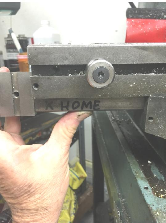
The X Home calibration bar is held against the table's ways. I'm Home when a block on the end is a snug fit to the flank of the table and the end of the bar.
