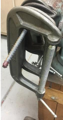
To keep the C-clamps from falling off the rod, they must first be closed all the way. Yet, to use one, it must be opened. Therefore, this storage method forces us to have all clamps in a non-ready state.
