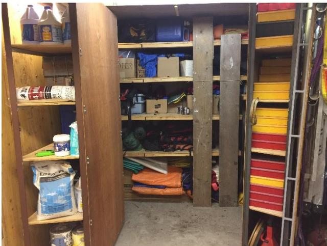
Dave calls this his layered storage area - 3 layers deep. First is the front of the hinged panels, with nominally "flat" stuff hanging (like ladders). Opening the panels reveals shelves. The shelving units are welded assemblies that are also "hinged" on wheel bearings to allow access to fixed shelves behind. The main reason for this extravagance (other than I thought it was a neat idea) is that the space was
