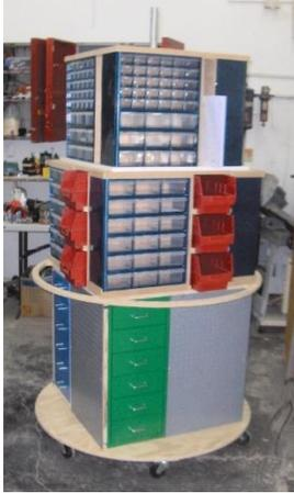
This masterful fastener storage unit was designed and built by John Herrmann. He has a large shop so this saves him steps. The fasteners have been organized so there is minimal turning of the unit during a job.
