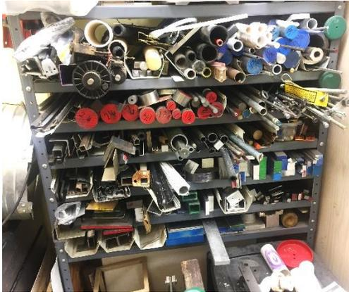
This is common metal shelving loaded with various U shaped trays. You get mostly random access and direct visibility as long as it is not overloaded. Those U shaped trays prevent sideways avalanches of metal. These trays are cut up plastic rain gutter.
