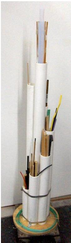
This is another contribution from John Herrmann. Various lengths of stock are supported by the 7 different lengths of PVC pipe. This is good because he gets direct visibility and random access. The assembly is secured with large hose clamps.
