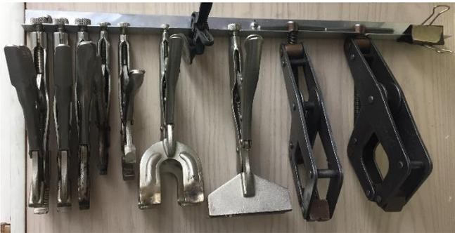
My solution was to hang them on a nearby wall. I cut a slot in a piece of light gage aluminum angle that was a close fit to each adjustment screw extending out of the back of each Vise Grip. The two Kant Twist clamps are hang from this bar.
