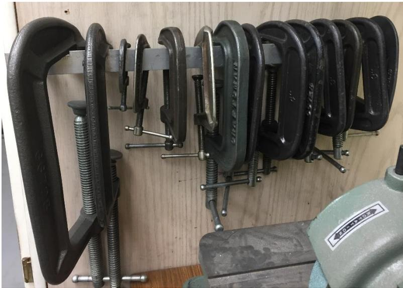
The C clamp rack is much simpler. I used another length of light weight angle and just hang the clamps on it. As long as they are open enough to get over the bar, there is no fuss.
