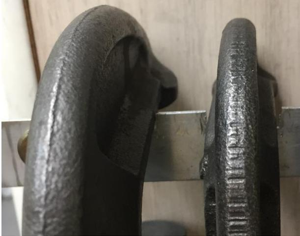
The two C clamps on the left were rather large and heavy. They tend to rotate so I cut notches for them.
