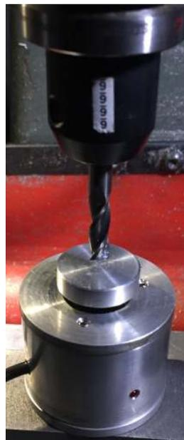
I tell CNC12 to set my reference. Push a few buttons and the height is recorded. Then I change to my first tool and assign it to Tool 1. Push a few buttons and CNC12 will record how much shorter this cutter is than my reference. If I have a second tool, it would be assigned to Tool 2.
