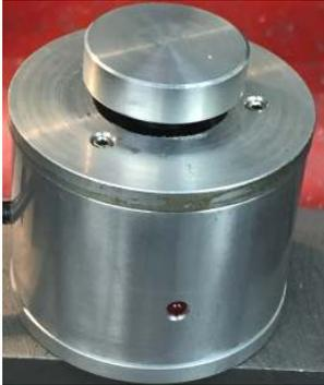
My Tool Touch Off is a precision normally closed switch. When that top disk is depressed slightly, the switch opens. A small amount of current still flows which lights the built in red LED. This is not enough to throw the Acorn's input circuit off.
