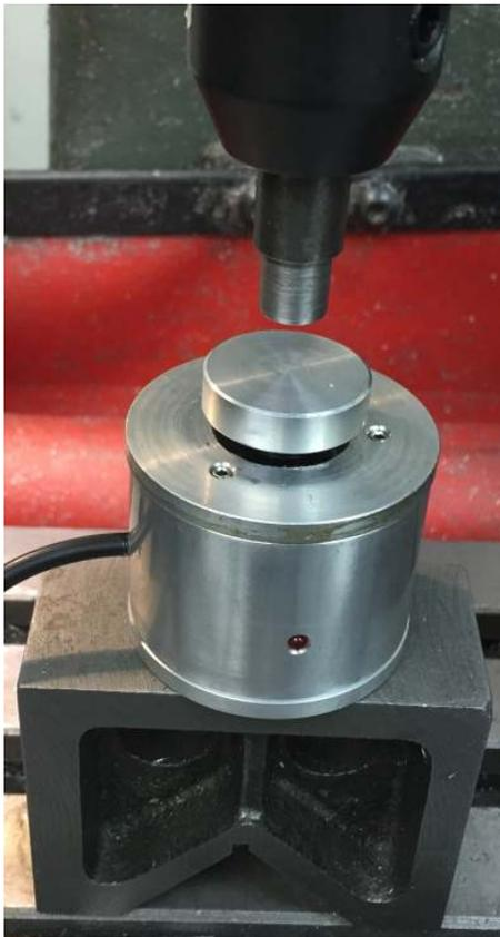
It is very handy to be able to define height differences between cutters. Once done, G code commands and Centroids CNC12 software can automatically compensate for this height. The tedious bit is measuring those differences. Owning a Tool Touch Off (TT) device makes this a semi automatic task.
