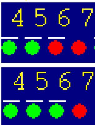
A close up reveals what the software will see at its inputs. Input 6 has a red dot. My TT is in its "normal" state. That red dot under the "6" means that IN6 is pulled low and the LED is on.
