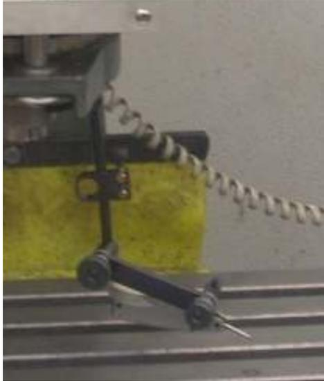
My DTI is attached to my spindle and free to move to the 4 points. Since the vertical distances are far beyond what a DTI can handle, I used the DTI in conjunction with my Digital Read-Out (DRO). The DTI is first set to be 0.002" away from zero. The spindle is then lowered until the DTI swings over to 0. In this way I have minimal force on the DTI support and an accurate way to tell when I am at touchdown.
