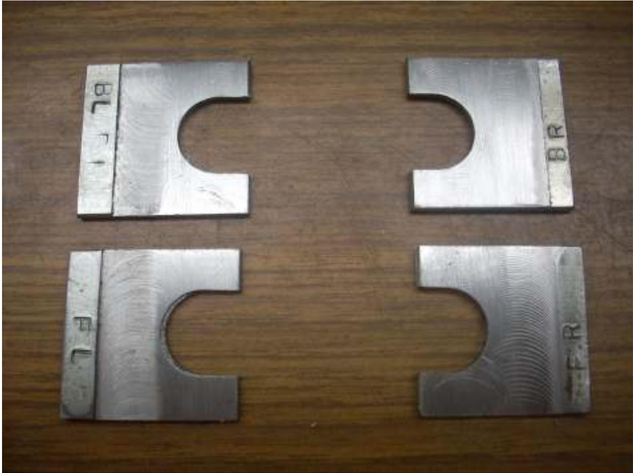
Using my 5/8" end mill I have cut slots to accept the 1/2" bolts.
