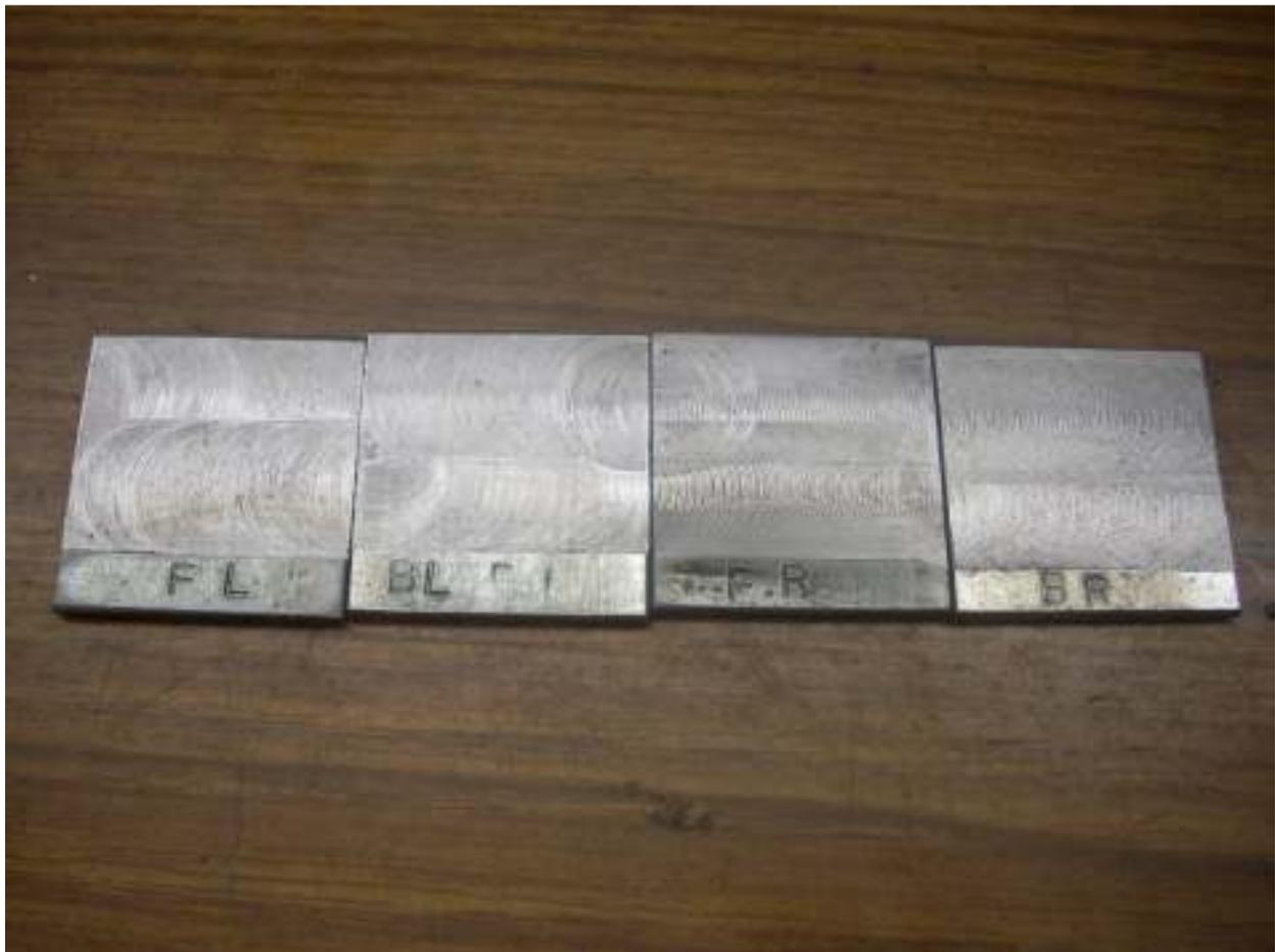
I have cut and stamped the 4 shims. The far ends were sawed off and all edges deburred.
