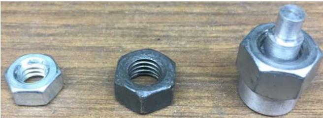
The 3/8-16 nut clears the two smallest diameters and rests on the base.
