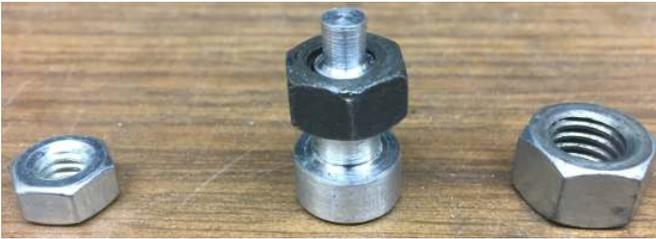
The unknown nut is dropped onto the gage and it passes through the smallest diameter but is stopped by the largest diameter. This means it must be a 5/16-18 nut.
