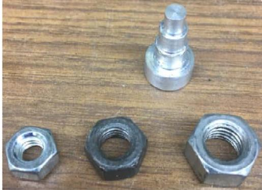
We can also make a gage to sort nuts. Here we have a 1/4-20, 5/16-18, and 3/8-16 nut. The gage has been turned on my lathe to have diameters of 0.196", 0.252", and 0.307". These are the minimum minor diameters of these inside thread sizes. Each diameter can be +0 / -0.01" and still get the job done. Note that Metric nuts can fool this gage.
