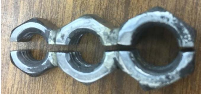
A variation on the nut idea is to braze or epoxy nuts together and then saw across them. Deburr as needed. If you are able to cut right on the centerline, you get one tool for yourself and another for a friend.
