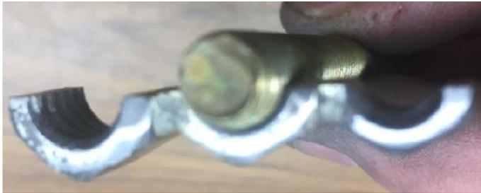
Slap the gage against the side of the bolt and if it fits snugly, you have identified the thread size.
