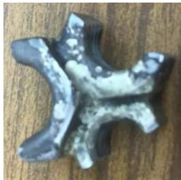
A variation on this idea is to braze or epoxy three nuts flat to flat. Then saw each one shy of the center. A bit of filing will be needed so the bolt can slide in but you get the maximum possible amount of thread engaged.
