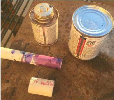
It is possible that a steel mandrel can be made with a diameter equal to the maximum diameter of ½" PVC pipe. According to one source, this pipe is  $0.840 \pm 0.01$  inches. Therefore, a mandrel 0.850 inches in diameter would pass all pipe. However, in the worst case, there could be a gap of 0.02 inches between the resulting coupler and the smallest diameter pipe (0.830 inches). My concern is that it might leak.
