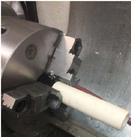
I took a 5 inch length of scrap 3/4 inch schedule 40 PVC and held it in my lathe chuck. The lathe was set to run at 26 RPMs. Next, with the lathe turning, I used my heat gun to warm about 2 inches of the end of this pipe. Since it was constantly turning, the heat was evenly distributed.
