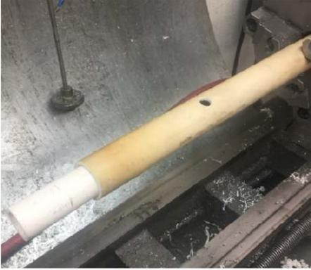
Here is a length of 1 inch schedule 40 PVC in my lathe chuck. It was heated for about 45 seconds. I forced a piece of  $\frac{3}{4}$  inch schedule 40 PVC into the bore. After waiting about a minute for it to cool, the mandrel was removed. I cut off about 2 inches of the 1 inch pipe.
