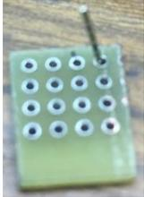
Then a scrap of circuit board is cut to include all of the holes to be drilled. With the pin in the top right hole and the circuit board on the bench top, I heated the pin and hole and add a *very small* amount of solder. Excess solder will coat the bottom of the pin and is a pain to remove without disturbing the pin alignment.
