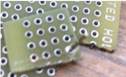
Then I placed the template over the edge of the circuit board and reheat the pin and hole. The pin drops down the proper distance. I used my finger to set the pin vertical before the solder cooled. Finally, I snipped off the excess on the top of the template. Repeat for the bottom left pin.
