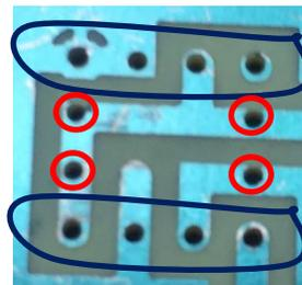
You can see the top and bottom holes are nicely aligned. But then there are four holes that should not be there.
