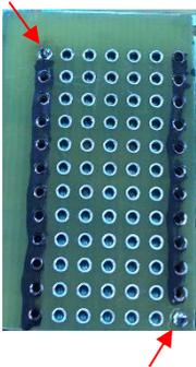
In this template, I have soldered in my two alignment pins. The black lines remind me where to drill. My drill is a close fit to the holes.
