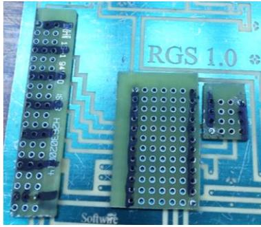
Here you see the three templates I built for this circuit board. The black lines tell me which holes to drill (duh).
