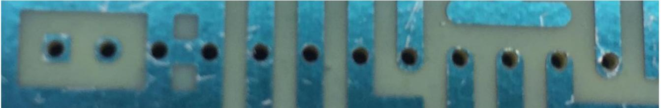
Drilling a series of holes in a circuit board so they line up with the copper traces can be tricky when the drill bit is 0.03 inches in diameter. I often need to do this just once or twice on a hand etched board and the patterns vary.
