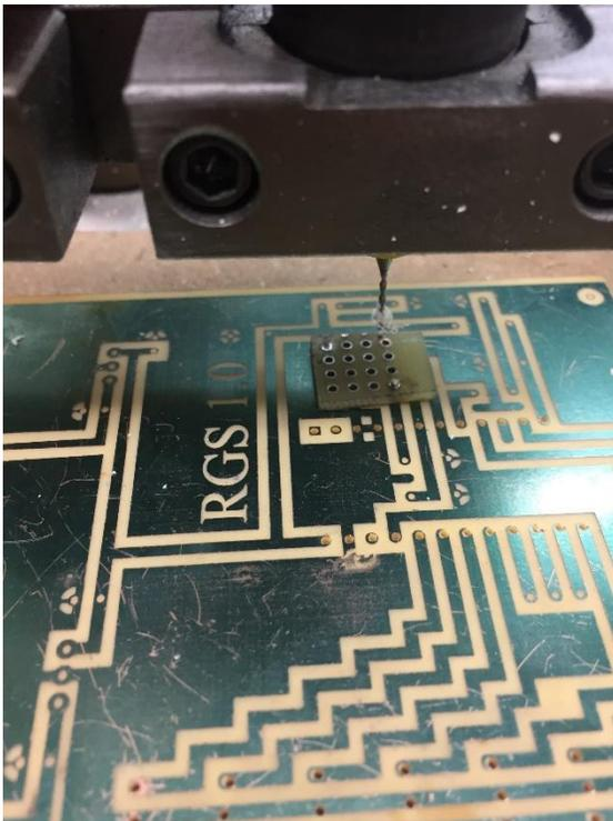
Then the template drops in. Drilling was quick and accurate.
