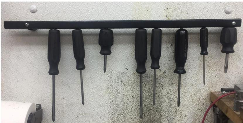
I installed a neodymium magnet<sup>2</sup> into the top of the handle of each screwdriver. A dab of 5 minute epoxy did the trick.
