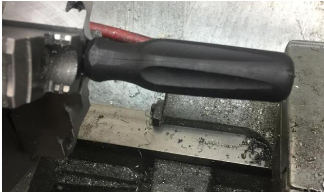
Each screwdriver went into my lathe for drilling.
