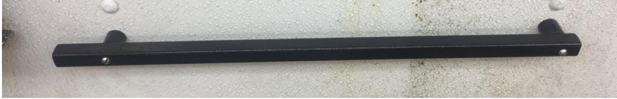
The bar is a piece of ½" square steel tubing about 18 inches long. Two holes are drilled through it 16 inches apart. This lets me run my screws through the tubing and into studs in the wall. Two spacers, made of conduit, place the tubing about ½ inch from the wall. A coat of black paint and it all looks new.
