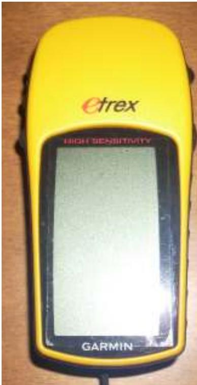
I own a hiking GPS from Garmin called an eTrex H<sup>®</sup>. The gray scale screen is 1.1" wide and 2.1" tall. I can select a screen format that show me a line that represents just my route. With the map scale set correctly<sup>1</sup>, it just takes a quick glance to see what to do next.
