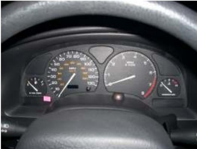
Consider the design of the standard instrument cluster in a car. It really is a masterful design of human/machine interfacing. As you throw a quick glance at the cluster, you can easily tell that no red lights are on. No need to bother you if all is well. If you want to know the speed, you have an analog dial with only numbers on it. Often you don't even need to see the numbers, just the position of the needle is enough.
