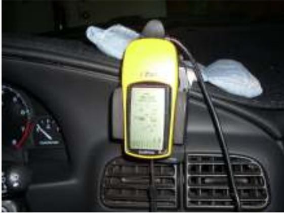
I have built a holder for my eTrex H that suspends it to the right of the instrument cluster. It is on the same viewing plane as my cluster making it easy to see without refocusing my eyes. The uncluttered and small screen of the eTrex H is consistent with the simplicity of my instrument cluster.
