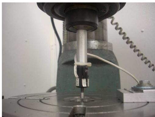
I start out with the EEF roughly centered on the RT. The tool offset is set to center.
