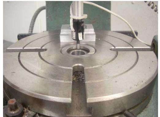
So how good was my alignment using a DRO? I put in my pin and DTI. The mill table was moved until the DTI showed I was aligned within 0.0005". I then looked at my DRO display and saw that my X axis had been moved by 0.001". My Y axis was not moved at all. I repeated the test and this time found that no movement in the X or Y axes was needed.
