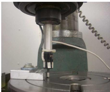
The RT was then turned 180 degrees. My EEF has just come in contact with the block. The distance traveled divided by 2 is the center of the RT along the X axis.
