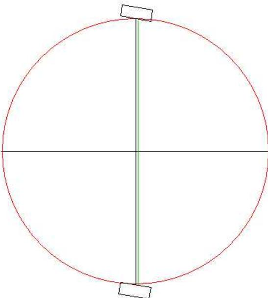
I now have a Y axis centerline very close to true. By repeating the X axis centerline again, I will get it closer. You can repeat this process as many times as needed to get to the limits of the DRO's repeatability and accuracy.
