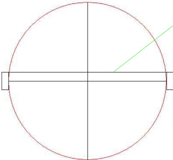
Here I am moving along a line parallel to the X axis but with a non-zero Y value. If, and this is a big if, the block face is perpendicular to the X axis, then Y misalignment of my line does not matter. In fact, if the block is 2" wide, I can be off by 1" and still find the point on the X axis which is aligned with the RT's center of rotation.
