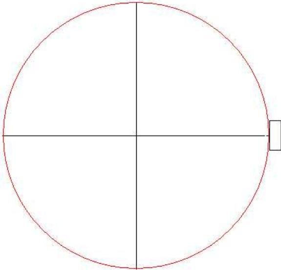
Next I crank the RT until the block is at 180 degrees. If my Y location is exactly at the center of the RT, then when I touch down on that same inner face of the block, I will be at a distance equal to the diameter of the circle inscribed by the block minus the diameter of the EEF probe. I don't care about either diameter. But if I now run the centerline function, I will see how far back to crank the X axis to end up at the center of rotation of the RT along the X axis.
