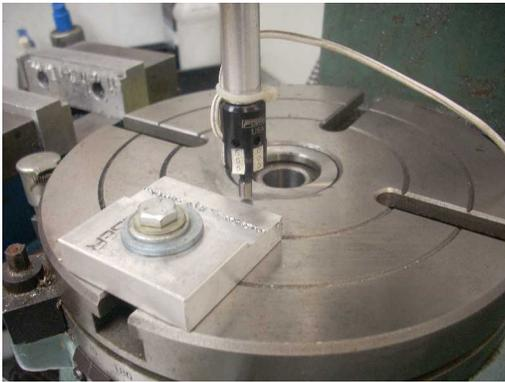
The process is repeated for the Y axis. Here you see the EEF coming in contact with the block as it has been moved to 90 degrees. At touch down, the Y axis is zeroed.
