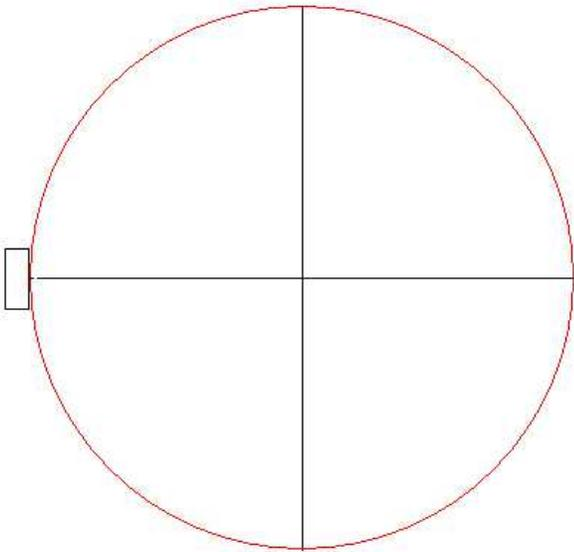
Say I attach a block to the surface of the RT<sup>2</sup> and set the angle to 0 degrees. I then define the block's inner face as  $X = 0$  with an Electronic Edge Finder connected to my DRO. I would do this by moving the EEF from near the center of the RT out to the block. When the EEF contacts that inner face of the block, I set my zero for the X axis.
