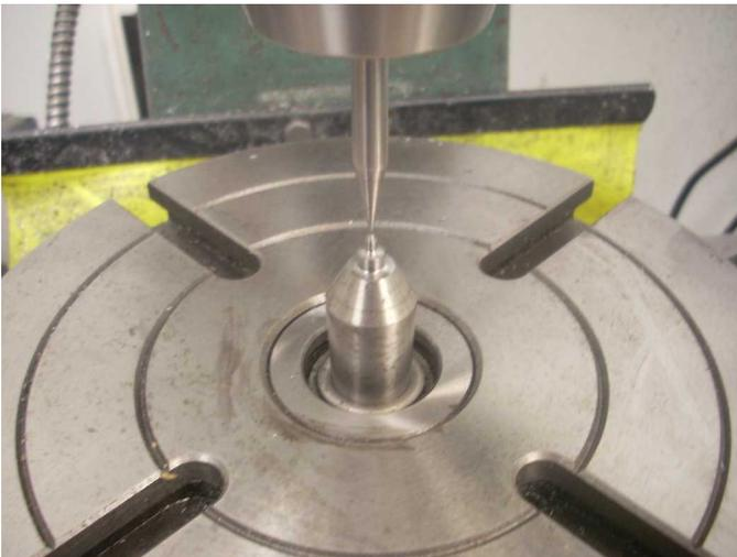
Before you can use a Rotary Table on a mill, its center of rotation must be aligned with the spindle's center of rotation. Many means exist with varying degrees of ease and accuracy. In most cases, you start with a rough alignment. My favorite method is to mount a spud in the spindle and a modified dead center in the RT's tapered hole. This can get the center of rotation of the RT to within about 0.02" of the center of rotation of the spindle. For some jobs, this is plenty good.
