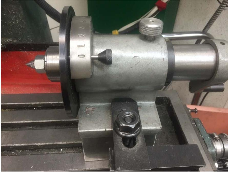
After setting up my 8 inch rotary table to be the drive for my 4th axis<sup>2</sup>, it was time to figure out the tailstock. I could buy one on eBay for around \$100 including shipping, I could make one from scratch which would take a few days, or I could adapt something I already owned. A bit of hunting turned up my 5C collet
