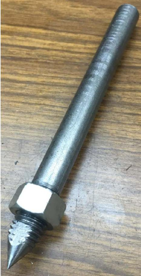
Since I wasn't sure this idea would work, I made the adjustable dead center out of  $\frac{1}{2}$  inch diameter CRS. I may later make one out of drill rod and harden the point.
