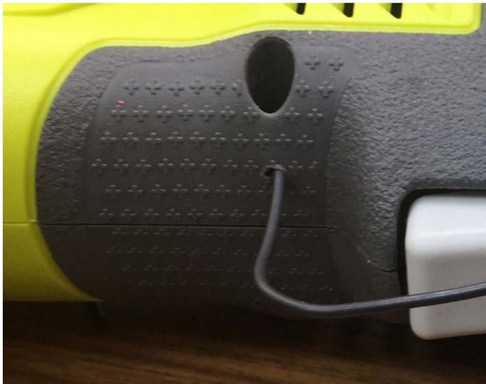
After removing the screw just below the trigger, I drilled an 1/8" hole tangent to the top of the chamber that held the screw. I then pushed the wire through the hole and formed a hook.
