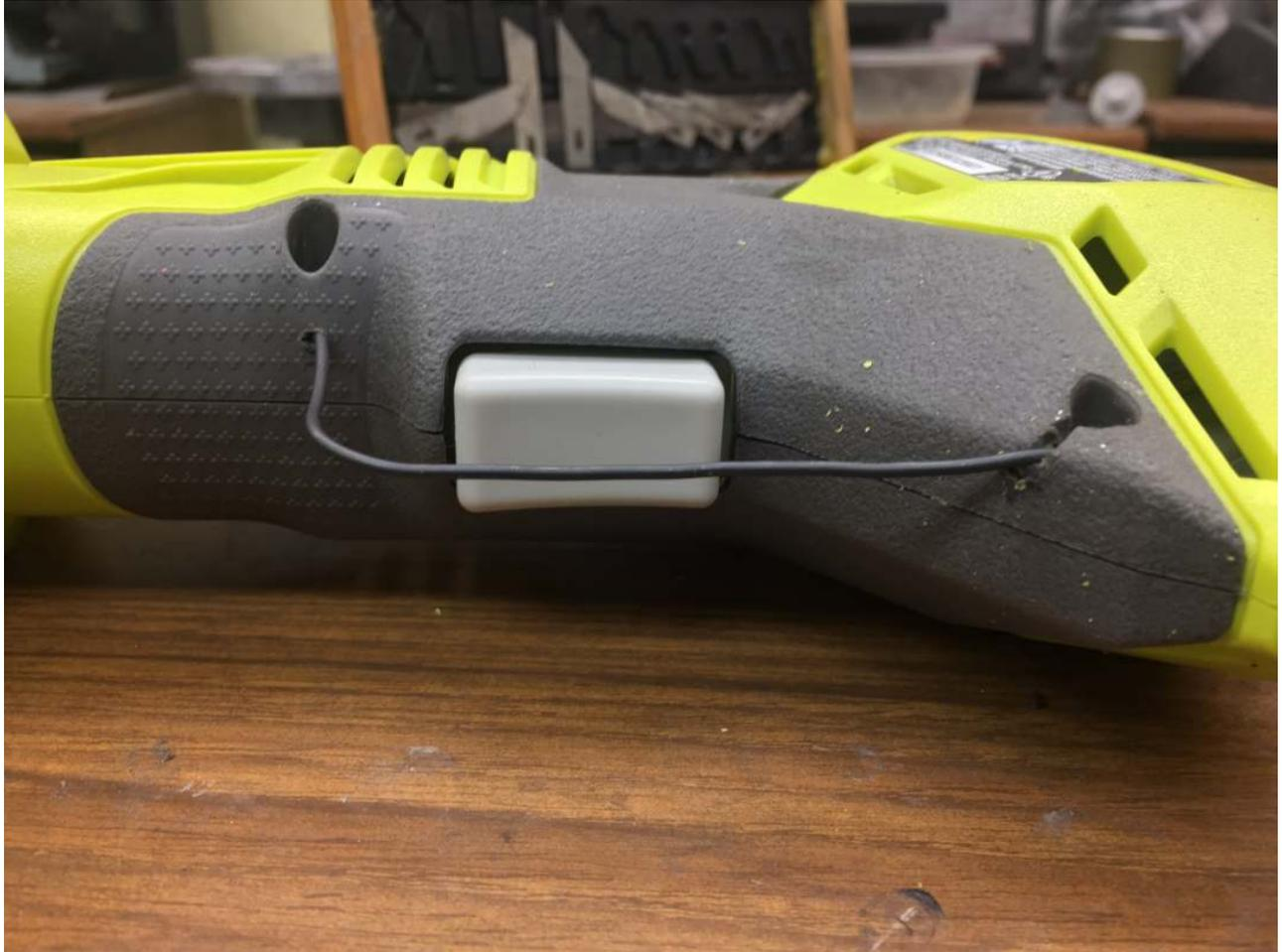
The final step was to bend the wire so it was centered over the trigger.
