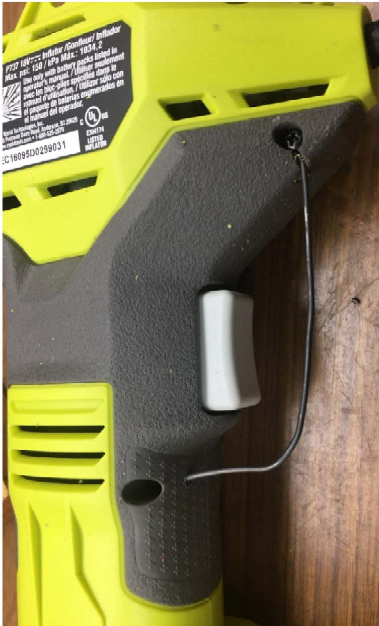
After installing the second screw, the soft wire guard was secure.
