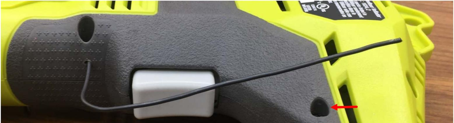
Next I notched out the rubber and plastic on the side of this hole. It was too shallow to drill a side hole plus the base of the compressor prevented me from drilling this hole at the needed angle.
