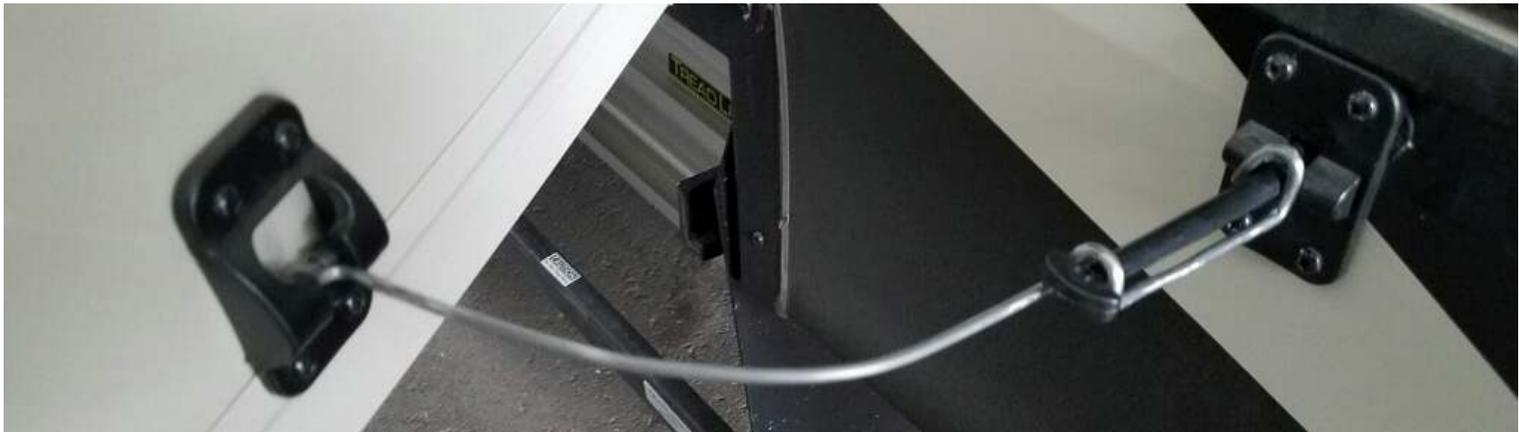
I had to slightly bend the end loop to fit over the arm attached to the trailer wall. Otherwise, it was usable on the first try.
