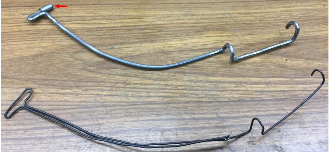
That sleeve on the end (red arrow) that fits into the receiver is a correction needed because I cut the wire about 1/8 inch too short.
