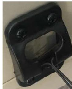
a pocket fastened to the door. This existing anchor holds the door almost flush with the trailer wall.
