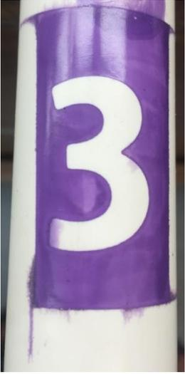
I tried Frog Tape and it was better than 3M tape for preventing bleeding. In this test I applied a rather thick coat of primer. The blob at the top was from a subsequent test.
