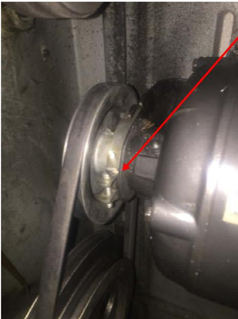
After over 25 years of service, one of the rubber support rings that holds the motor in my Atlas/Craftsman lathe failed. A search of the web found nothing that perfectly fit. The closest I could get had the correct outside diameter but the wrong inside diameter. This is how I machined two of these rings so they would fit.
