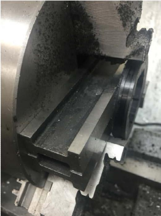
The first step was to secure the ring in the chuck so it would run true. I rested two large parallels behind the ring and then tightened the jaws until snug. Over tightening the jaws would excessively distort the ring and cause lobes on the inside after grinding.
