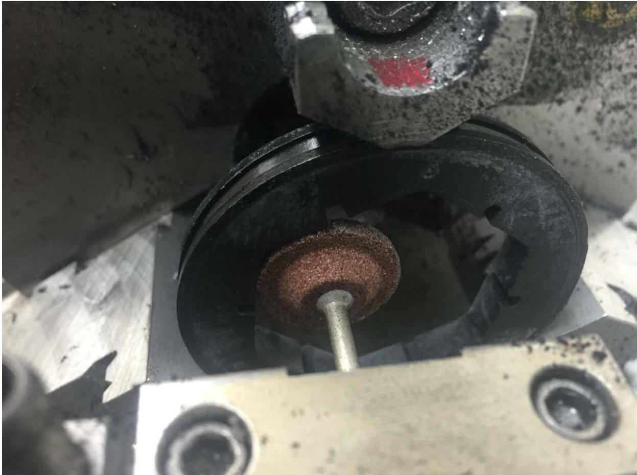
I set the cross slide to zero at the point where the grinding wheel just touched the minimum ID.
