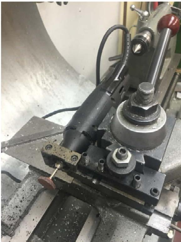
My Dremel was mounted in my toolpost using a support bar. A small grinding wheel was installed.
