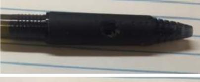
When there is still gel in the cartridge, the hole is blocked.
