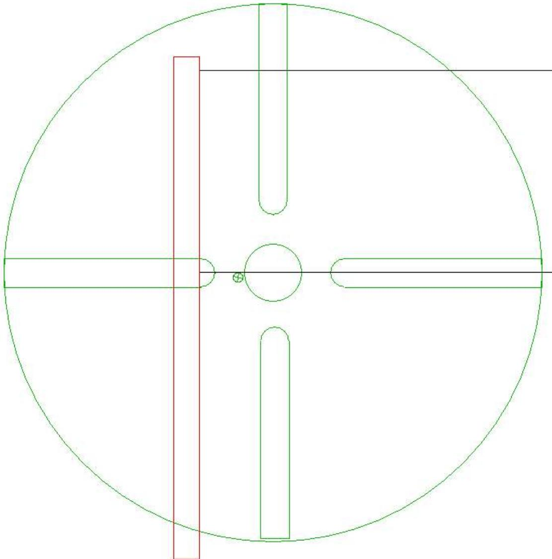
By moving the mill table in the positive Y direction, the spindle mounted rod is pushing the plate in the negative Y direction along the fence. As with the X direction, I can use the Y axis indicator to tell me how far I have moved the plate.
