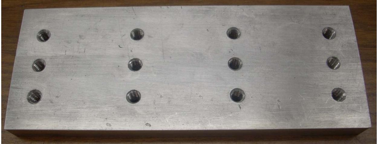
The first thing I made was the compound. It consists of a plate of 6011 aluminum with a grid of  $\frac{1}{4}$ -20 tapped holes in it. The plate has been machined square and is about  $\frac{1}{2}$ " x 3" x 6". I'm sure this will be handy in the future but I didn't use it this time.
