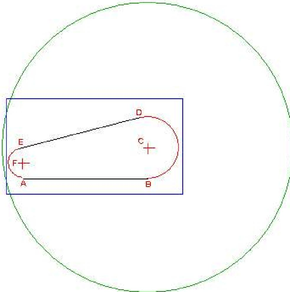
The block to be cut, shown in blue, is set up on the RT so line A-B is parallel to the mill's X axis and point C is at the center of rotation of the RT. The (0,0) point of the mill table is set up at the center of rotation of the RT.
