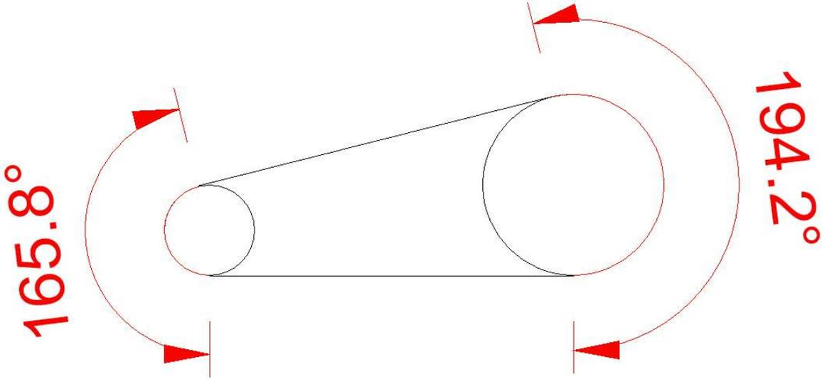
I can now delete the two circles. Using the dimension tool and the fact that the ends of the arc are easily found, I measured the length of the two straight runs.
