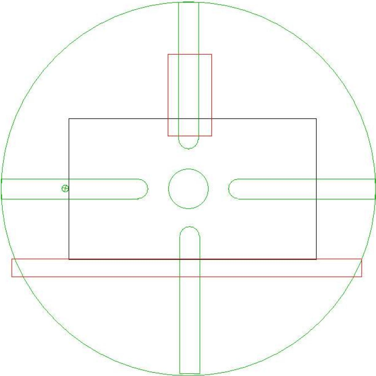
I have now moved the mill table along the X axis such that my spindle center of rotation is at the left side of the plate. Additionally, A small but rigid rod has been fitted into the spindle. The rod is in contact with the plate.
