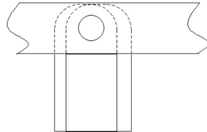
The dimensions of the various parts must come from your RT. The assembly is held together with a socket head 1/4-20 screw. No need to tighten a lot since the goal here is just to prevent the fence from moving as we reposition the plate. The rounded part with the cut out was initially supposed to give me alignment to the T slot but it is too sloppy. You may wish to just make the bar and tapped part that engages the T slot.
