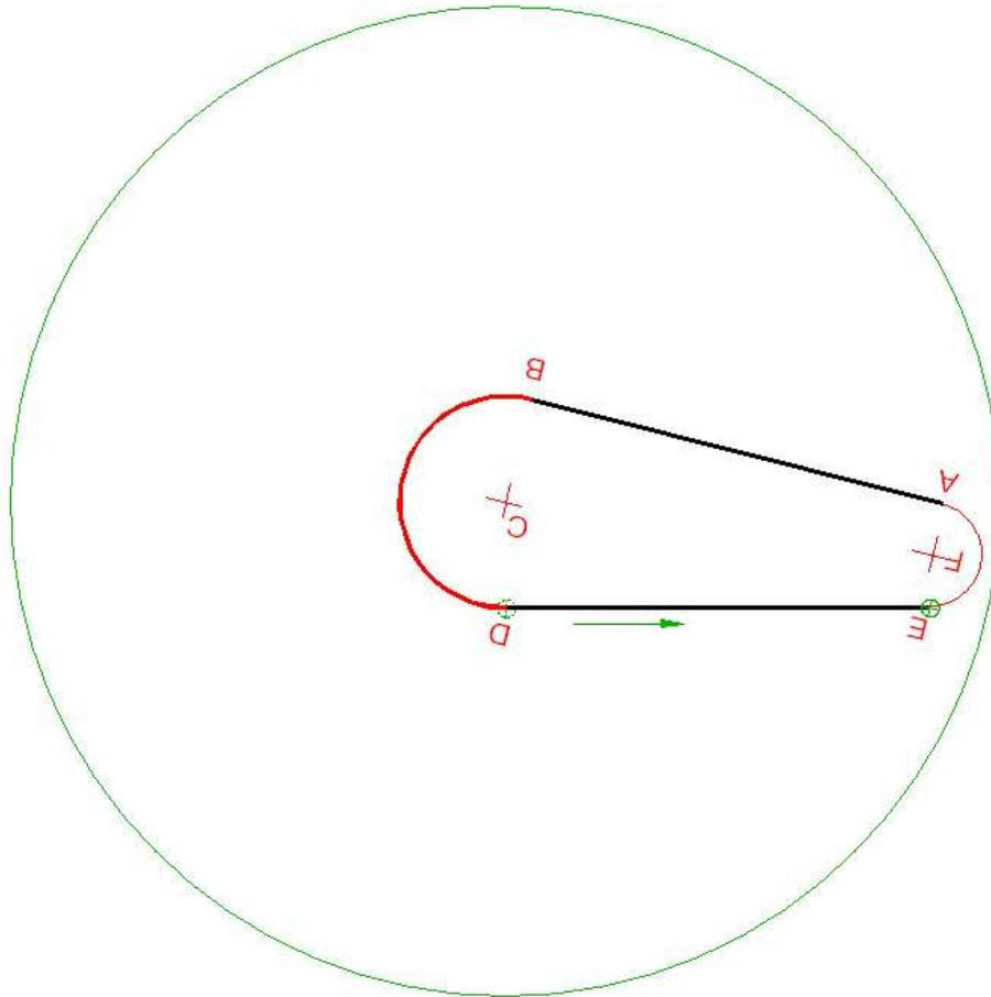
Line D-E, a tangent of the B-D arc, is parallel to the X axis as discussed on page tangents9. We just have to lock the RT, unlock the X axis, and move the cutter along line D-E to point E. At point E, the cutter is raised from the part.
