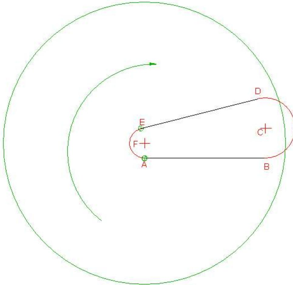
The X axis is locked and the mill started. Our part is rotated about point F clockwise. This causes the cutter to move from point E to point A and cut the 0.500" radius arc. The part is now finished.
