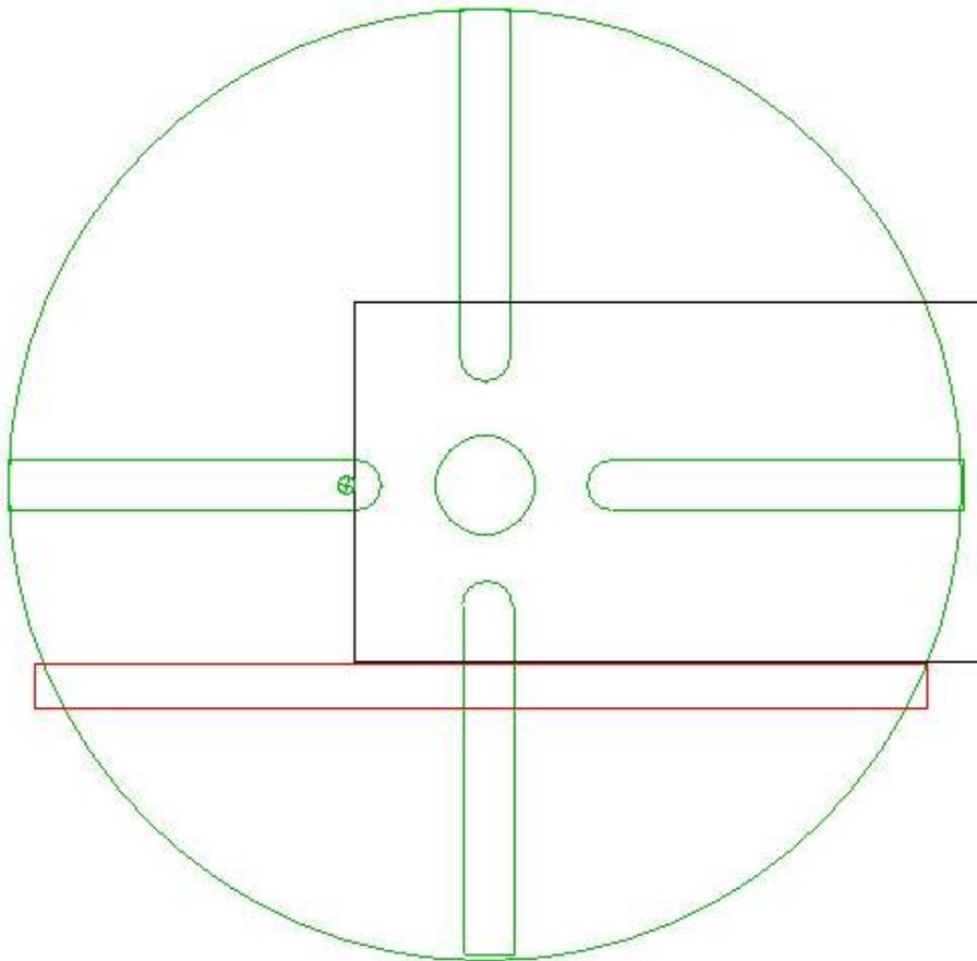
By moving the mill table to the left, my spindle mounted rod pushes the plate to the right. The fence insures that no motion along the Y axis will take place. Since no cutting is going on here, a light touch on the plate keeps it in contact with both the rod and fence. I know exactly how much the plate has moved because I can read it off of my mill table's X axis position indicator.
