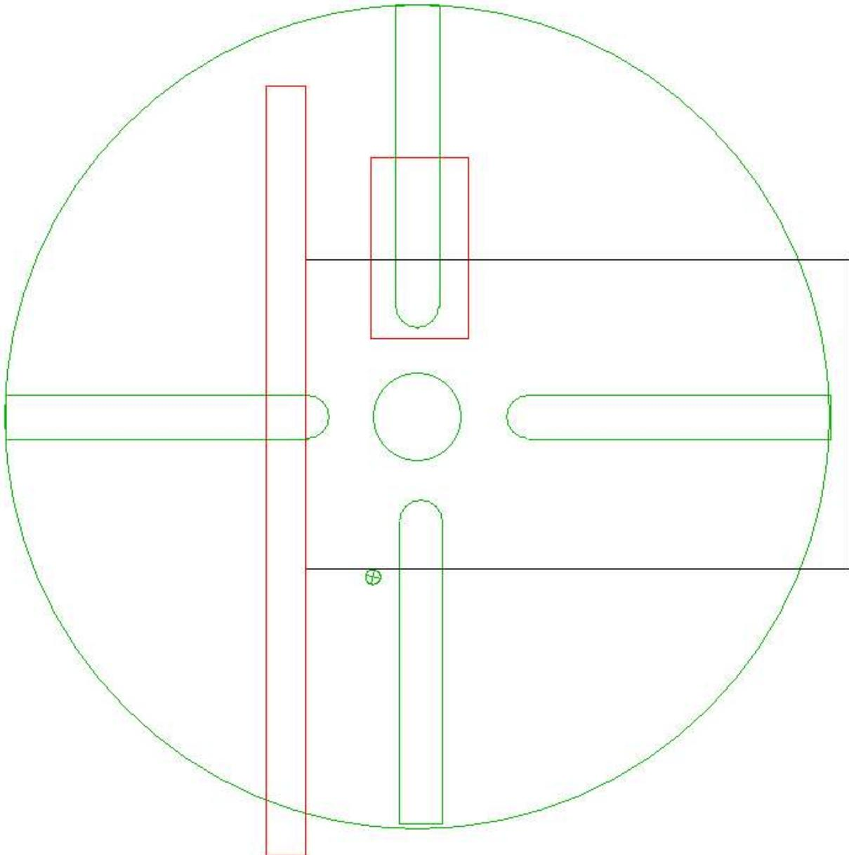
I first put back the clamp so the plate can't move. Then I move the fence so it is now contacting the left side of the plate. My rod is now touching the front side of the plate near the left corner.
