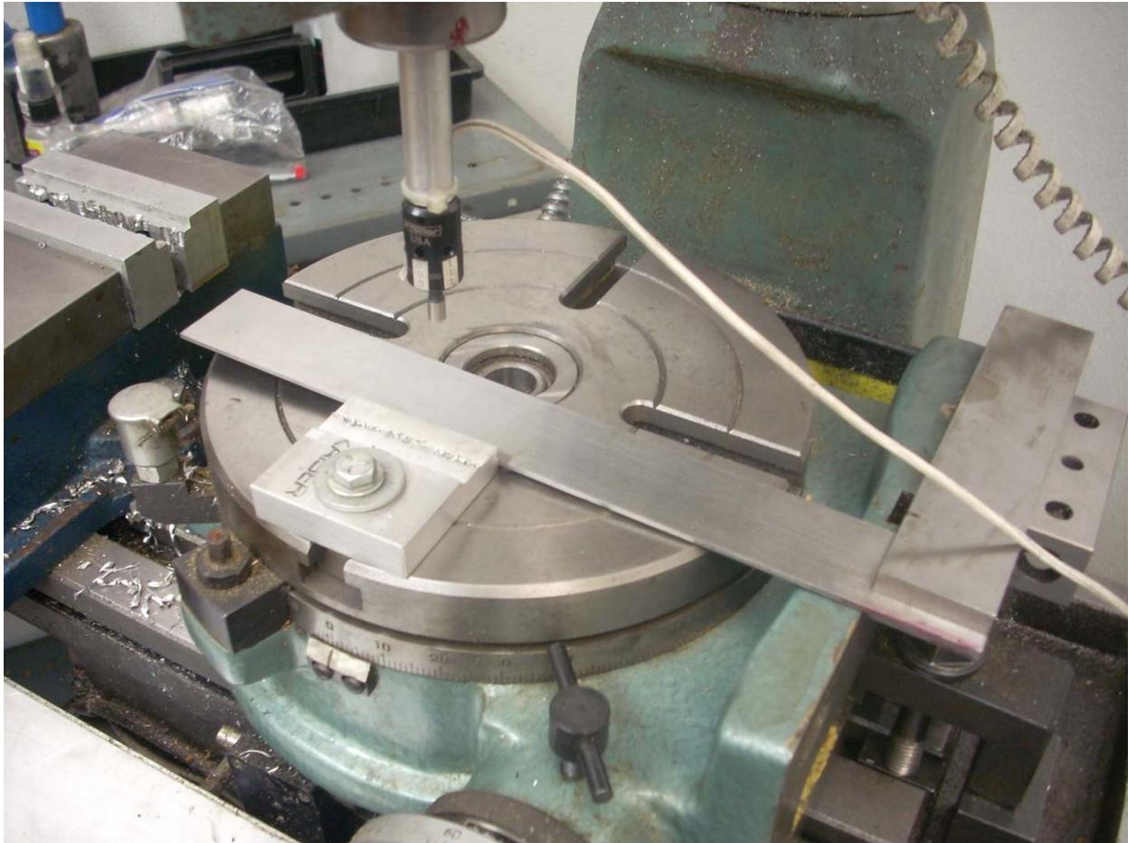
I will use an Electronic Edge Finder (EEF) and a block of metal clamped to the RT. The RT is set to  $0^\circ$  and the crank gear has been disengaged for now. I'm using my machinist square to get the block parallel to the X axis.
