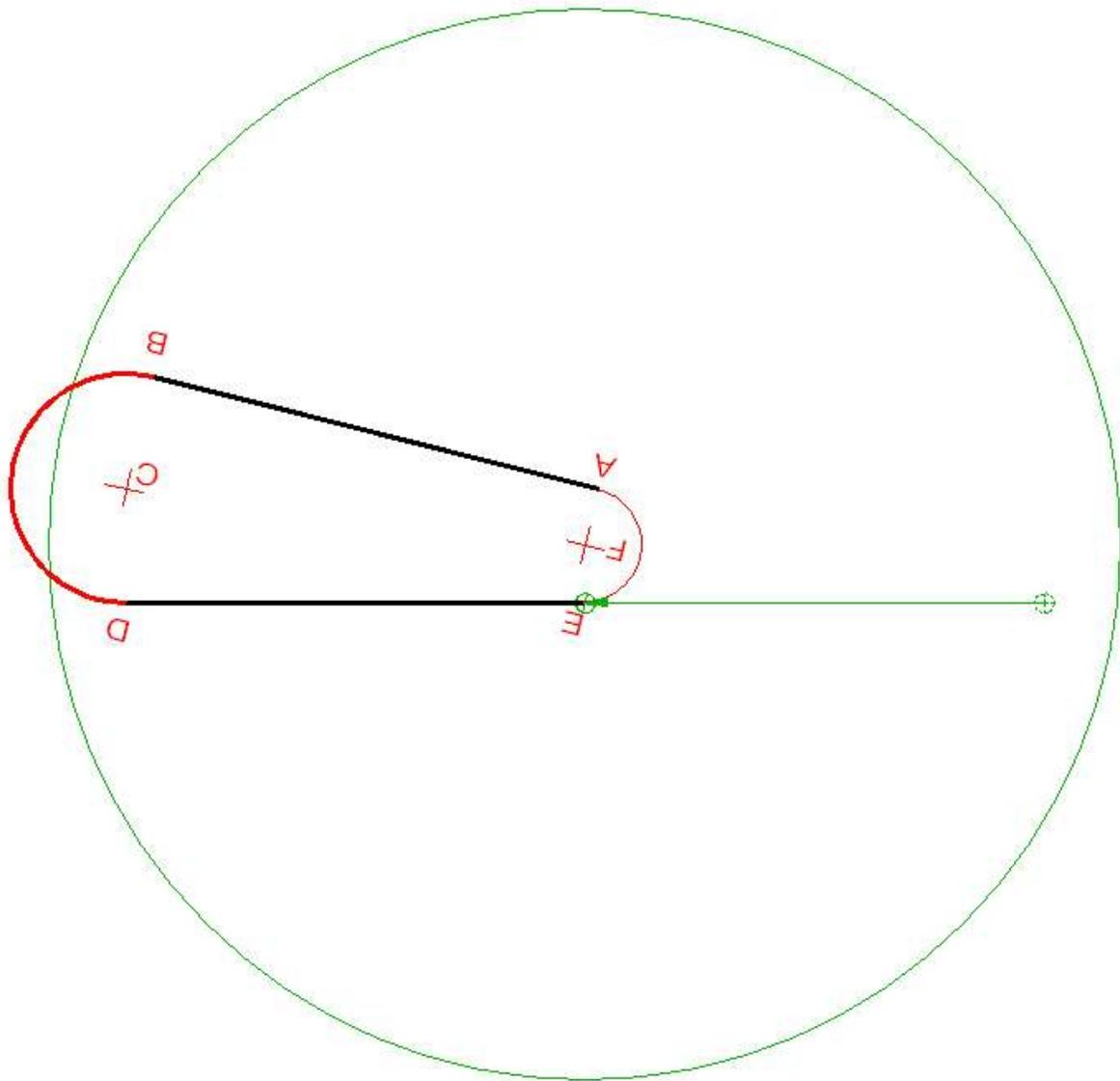
We know that point F is at (0,0) because that is how we initially set up the RT. Point E is directly below point F at a distance equal to the radius of the E-A arc, 0.500". By moving the mill's XY table, we put the cutter at point E. It is now lowered back into the part in preparation for cutting arc E-A.
