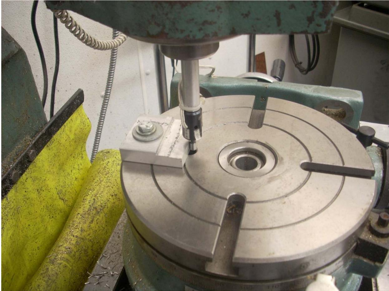
The RT is spun  $180^\circ$ . Then I move the Y axis until my EEF again contacts the block. Half the distance traveled is my  $Y = 0$ . The procedure is repeated for the X axis. I now have  $(0,0)$  set at the center of rotation of the RT. The crank drive is re-engaged.
