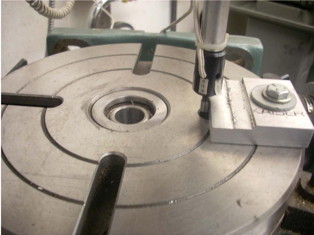
First I will align the center of rotation along the Y axis. I run the EEF, set with no tool offset, up to the block and set zero.
