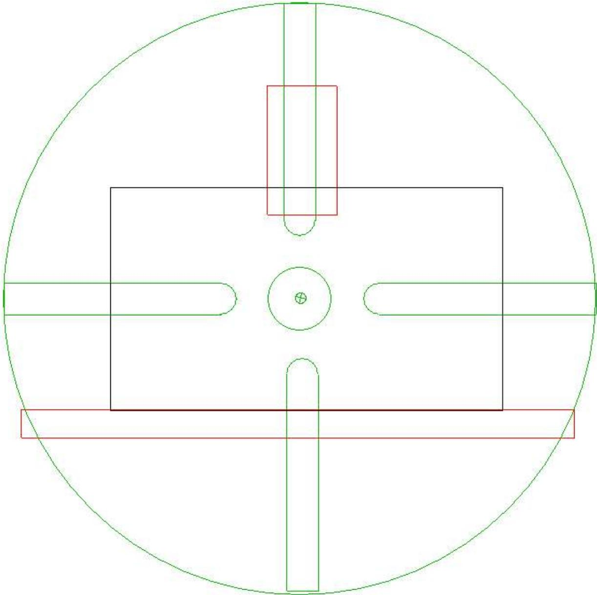
I don't want it to move yet so add a clamp at the 12:00 position. I also add a fence along the bottom<sup>3</sup>. Assume that the fence is clamped in place and aligned with the X axis. The center of rotation of the mill's spindle is marked with a small circle with a cross inside.
