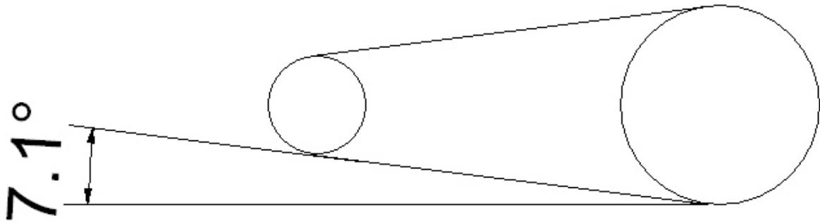
Using my CAD's measurement capabilities, I can easily find how much to rotate the figure so the bottom tangent will be horizontal. I then use my rotate tool to turn it counterclockwise by 7.1°.
