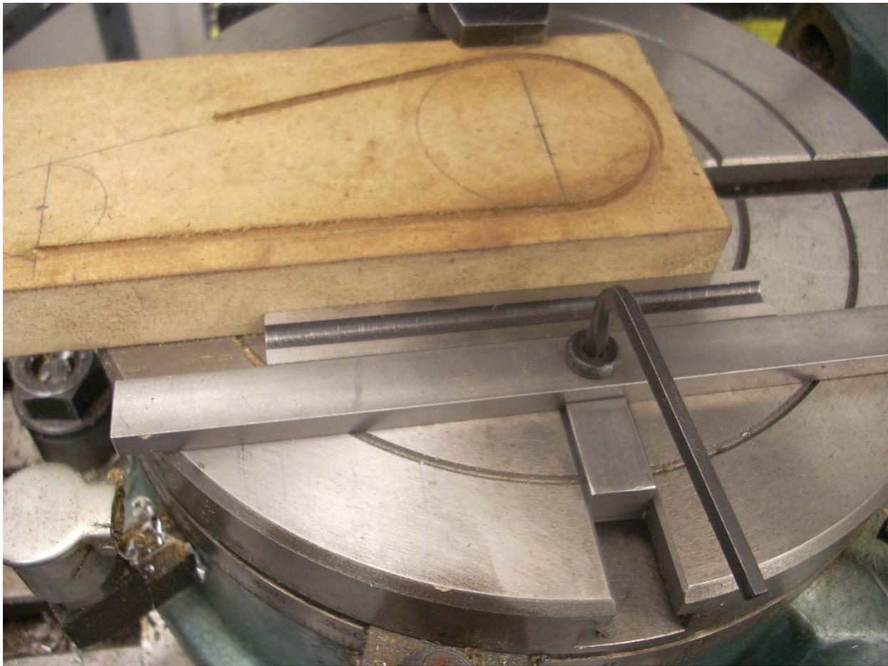
I have removed the front clamp in order to make room for my fence. I'm using a small parallel because the fence can't slide close enough to the MDF block. The block is used to align the fence before it is locked with the Allen wrench.
