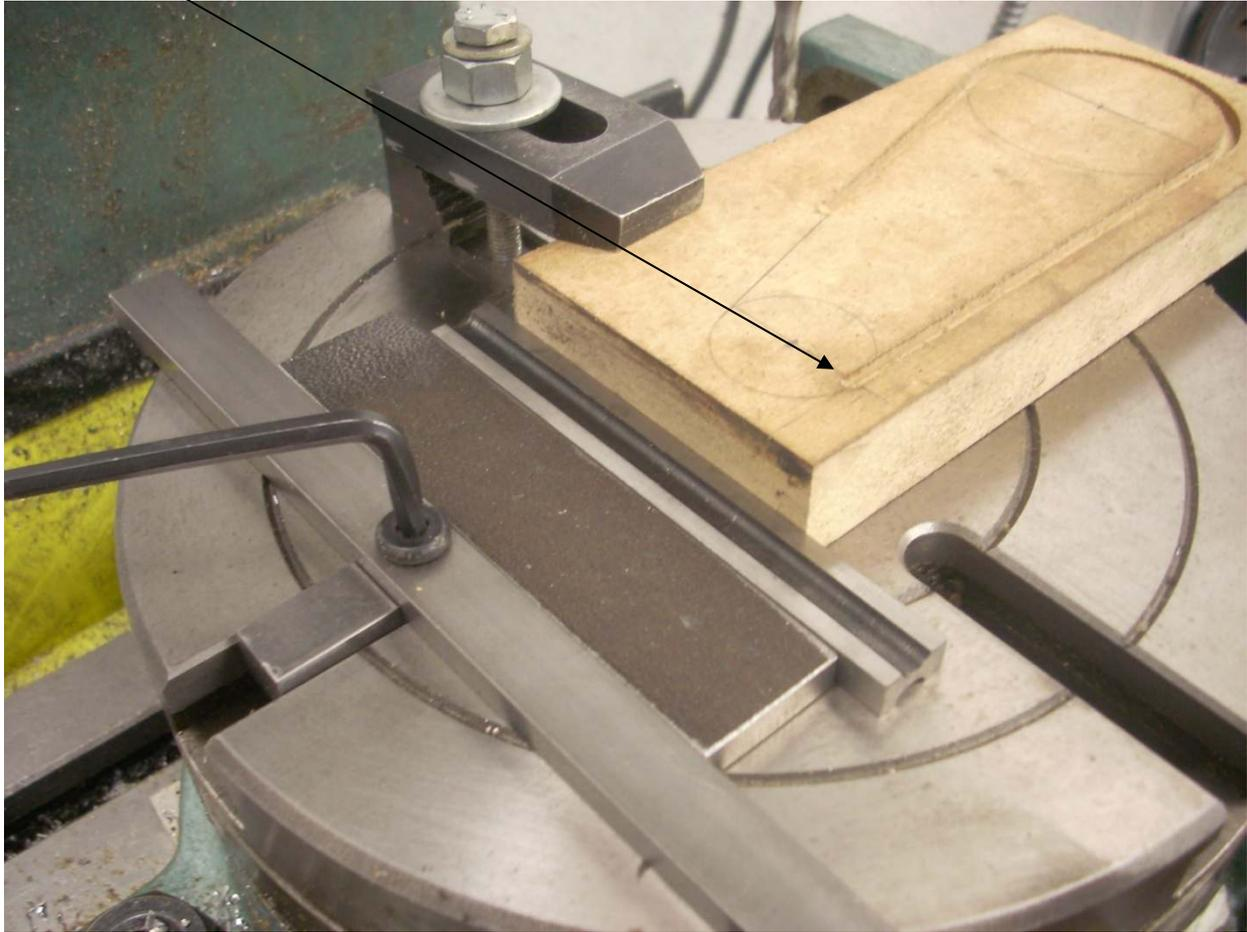
The process repeats for the Y axis. I had to use two parallels here. Not shown is the block being moved along the Y axis guided by the end mill.
