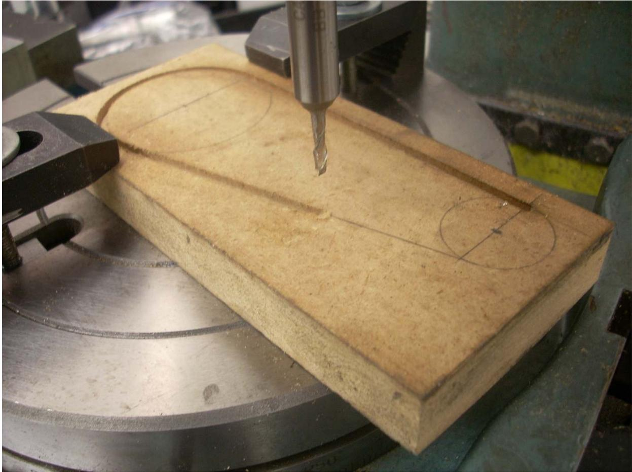
You may wonder why I stopped half way along the line. Well, I got caught in a lesson that keeps being repeated because I haven't learned it yet. I forgot to run the cutter over the full path before starting. My mill table is all the way to the left so the cut ends here. Time for plan "B".
