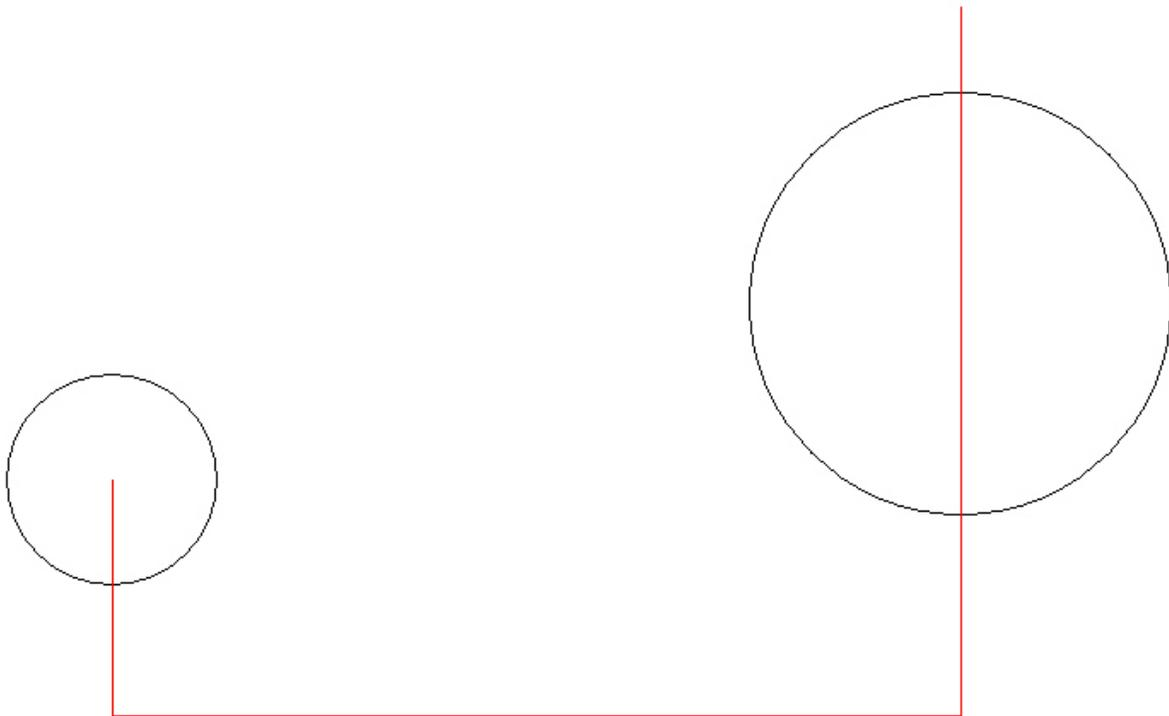
The small end has a radius of 0.500" and the large end has a radius of 1.000". They are separated horizontally by a center to center distance<sup>2</sup> of 4.000". I started by drawing a 1.000" circle on the left. A line was then drawn vertically from the center of the circle down a short distance. I then drew a 4.000" line horizontally.
