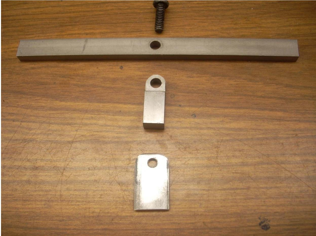
Not much to it. The rounded bar in the center gives a rough alignment of the fence to the T-slot but I still need to use my machinist square to get it right.
