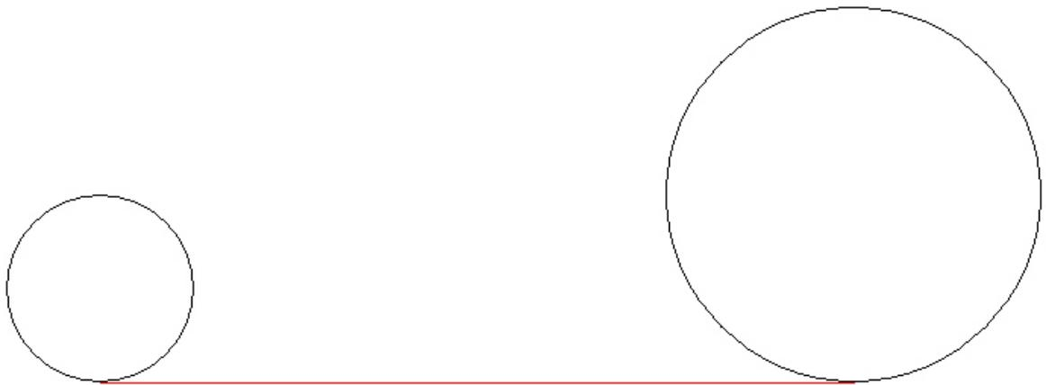
I then used the tangent tool to connect the tops of the two circles.
