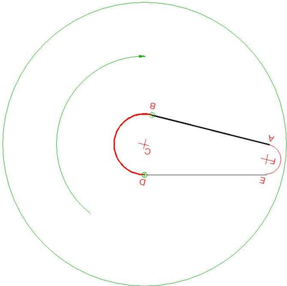
By cranking the RT  $194.2^\circ$ , we trace the arc and end up at point D. Note that the cutter went from point B to point D because the RT turned clockwise. It may seem strange but remember that the cutter really does not move, the part moves.
