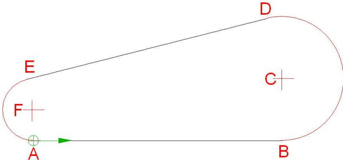
I want to move my cutter to point A. This entails moving the Y axis so the cutter is at point B, a distance equal to the radius of the large circle. I then move along the X axis until I get to point A.
