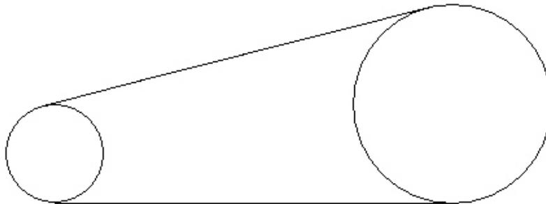
I now have each tangent 4.000" long and the center to center distance is 4.031". The lower tangent is parallel with the X axis.
