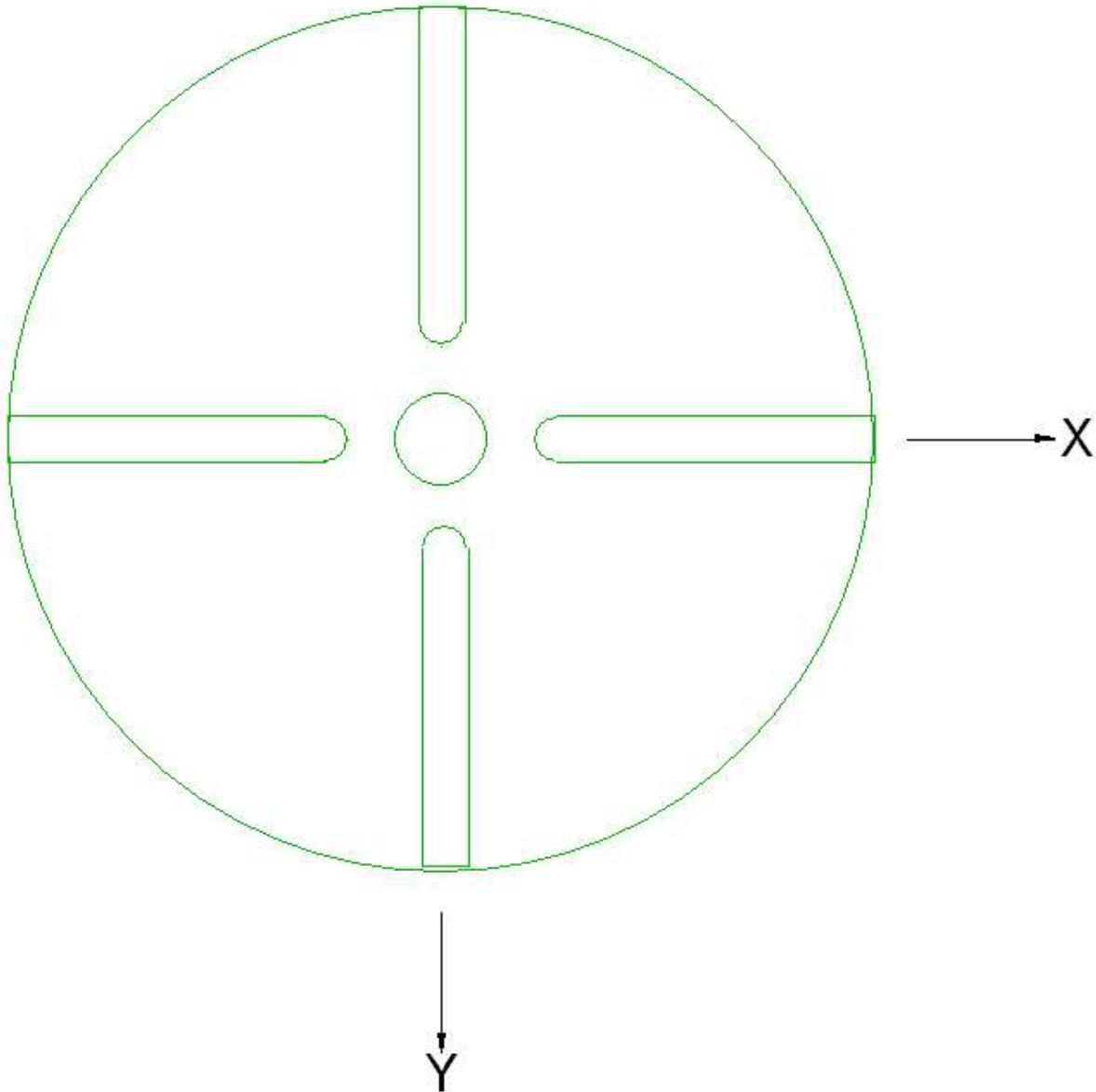
My RT is set at  $0^\circ$ . The center of rotation is aligned with the center of rotation of the mill's spindle. This puts my (0,0) point at the center of the RT. Note that I choose to define my positive X direction to the right and my positive Y direction to the front as the table is viewed from the top.
