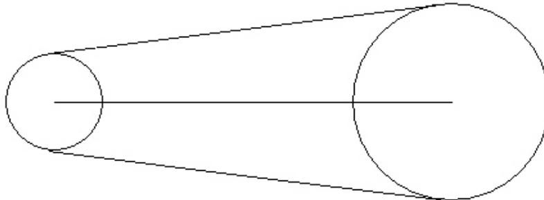
I then used my tangent line tool and drew in the top and bottom lines. I now have the same figure as shown on page 4. One more step will make it more usable: rotate the figure so one of the tangent lines is parallel to the X axis.
