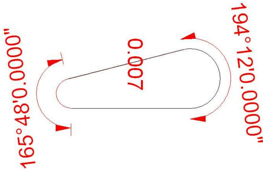
The exact error value was found by increasing the CAD display resolution to the maximum, inputting arcs equal to the truncated values, and then drawing two 4" lines at an angle of 14.2° to match the arc's truncated values. One line is black and the other is red. The red line was attached to the end of the small arc. The black line was attached to the end of the large arc.
