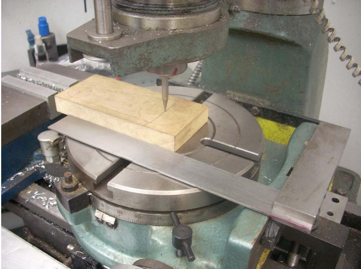
I'm using a spud mounted in a collet to hold the block of MDF while my machinist square aligns the edge. Recall that I want the center of the large arc to be aligned with my center of rotation. After clamping down the block, I mounted the end mill.
