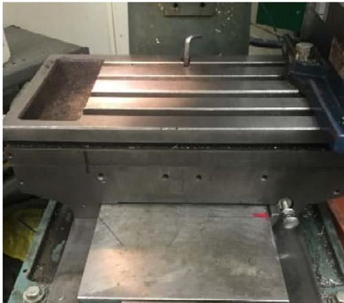
By drilling one hole, I am able to access the Y take up nut without disturbing the X axis. This hole enables me to feed an allen wrench through the table and into the top of the Y axis take up nut's Socket Head Cap Screw.
