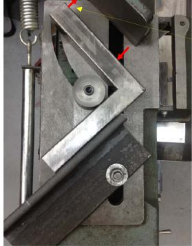
The end of the fixture will move towards the fixed jaw while closer to the 90° corner, the fixture moves away. This does not produce a usable clamping force.
