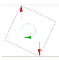
This might be clearer if you consider a square plate. Flanking the plate are two fixed walls shown as green lines. As I rotate the plate, the corners will move until they hit the walls. At this point, all of the turning force is
