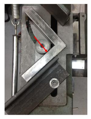
The first thing to understand is that when the cylinder presses on the fixture, the force will always be perpendicular to the surface of the bar and passing through the center. By using a cylinder, I get a smooth transition of this force vector as the fixture moves.
