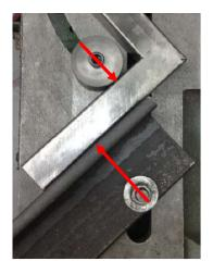
Remember that misalignment of force vectors? The larger this misalignment, the larger the twisting force. This actually helps us. If the vectors lined up, there is no tendency to rotate and no clamping force would exist between the fixture, workpiece, and fixed jaw.
