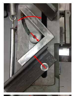
Looking at both vectors at the same time, we see that they do not line up. This causes the fixture to rotate clockwise as the movable jaw is tightened.
