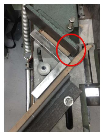
After the cut is made, the movable jaw is loosened slightly. By swapping the workpiece with the scrap, minimal movement of the movable jaw is needed.
