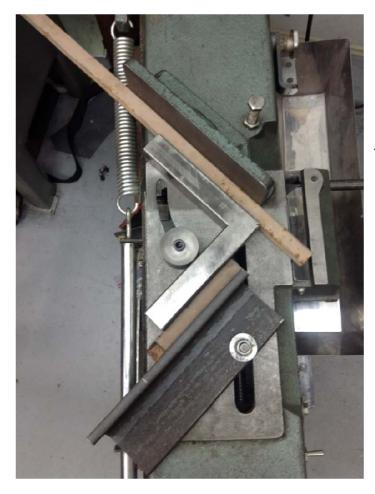
As shown here, I have first used my fingers to press the fixture against the workpiece, fixed jaw, pivot, and movable jaw. A piece of scrap is located between fixture and movable jaw. Its value will become evident soon.
