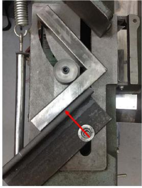
The force vector from the movable jaw turns out to be the same as for a cylinder. The vector passes through the pivot bolt. However, unlike the cylinder, there is a wide surface so friction to hold the workpiece is larger.
