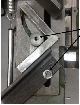
The nut is now under the base, the pivot is above it, and the bolt locks them together. The fixture rests on the pivot.
