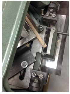
One solution is to build an attachment that permits both + and -  $45^{\circ}$ cuts with no change in saw set up or flipping of the workpiece. The picture on the left shows a - $45^{\circ}$  cut while the facing picture is + $45^{\circ}$ .
