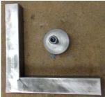
The attachment consists of two parts. One is a right angle fixture made of 16 gage 1" square tubing. The corner has been mitered, welded, and ground flat. The other part is a  $1\frac{1}{4}$ " diameter cylinder drilled to accept the hold down bolt.
