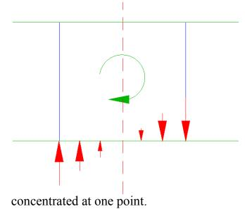
Consider our plate with a rotational force again in the center. This time the plate is sandwiched between the two walls, shown as green horizontal lines.
