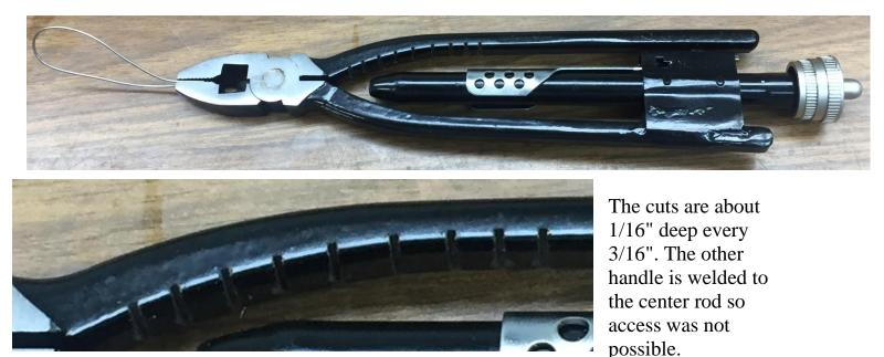
I was able to grab 0.041" stainless steel wire without undue effort. Today I used the tool many times to twist this wire as I secured rows of LED rope lights.
