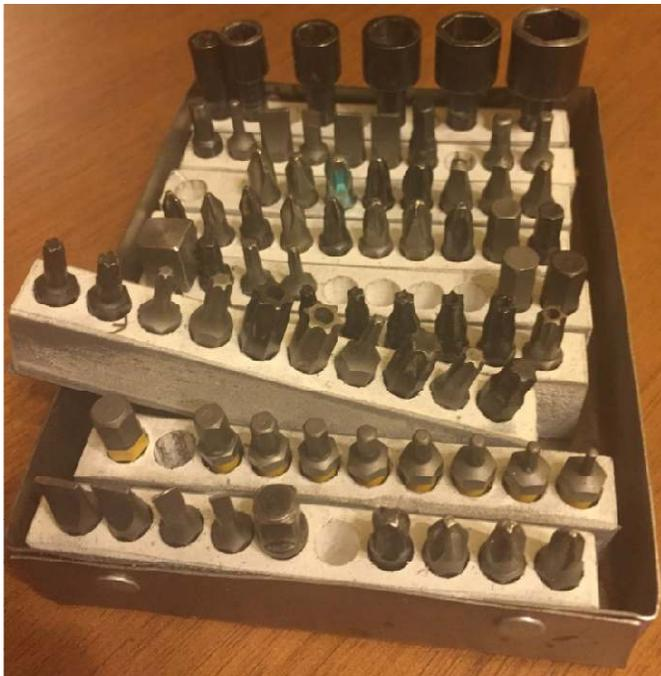
My solution was to make a set of  $\frac{1}{2}$ " wide bars  $3 \frac{1}{2}$ " long. Each bar holds 10 hex bits. It is easy to pull a bar out of the box and have full access to each bit.
