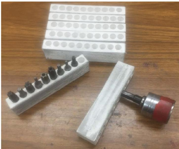
Next find the hex bit or adapter with the tightest fit. Press it into each hole to form the hex recess. You may need to move it in and out plus twist it slightly before it stops grabbing.
