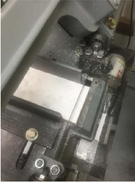
I started by sawing  $\frac{1}{2}$ " wide strips of the expanded PVC on my horizontal bandsaw. Laying the stock flat helps give a square cut.
