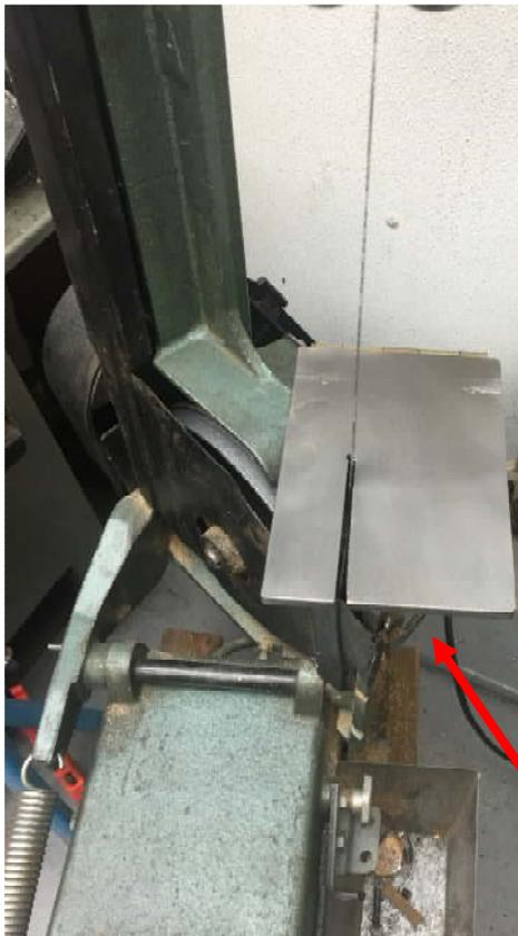
sawing have demonstrated that I simply will not bother. I was vertical sawing everything on that tiny plate screwed to the lower blade bearing support.
