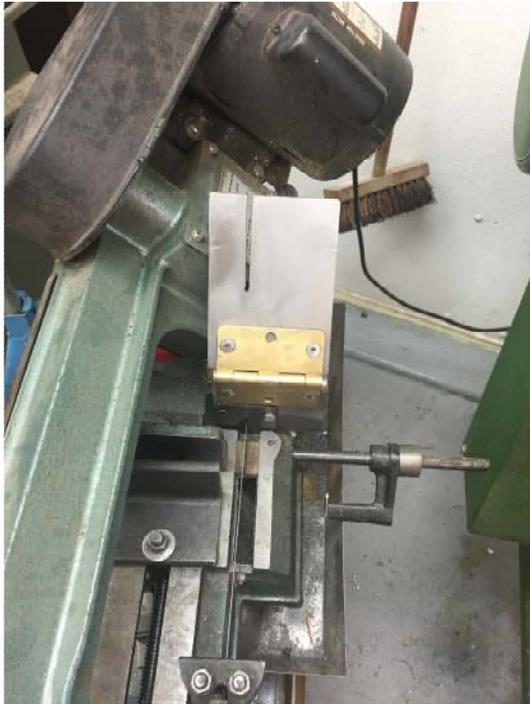
When the blade is in the horizontal position, the table folds back and does not interfere with the cut. It leans back about 45° so cannot flop forward due to vibration.
