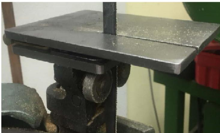
When the blade is vertical, the table folds down and contacts this bolt head. That bolt head is what keeps the table level. And since the table is then supported by essentially a line, the hinge, and a point, the bolt head, it can't rock and be unsteady. The downward force of cutting keeps the table seated.
