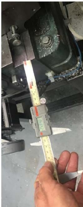
Did the same thing between the front of the base casting and the apron along the  $Y$  axis. It measured 2.5940 inches.
