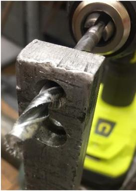
Poke the drill through your new drill guide with the countersunk side facing towards the point of the drill.
