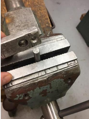
This drill guide works equally well on the end of a rod.
