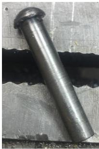
It is sometimes necessary for me to drill out a rivet. The drill tends to slide off the head until I cut a small divot. Then the job is easy. A trick is needed to get the drill centered.
