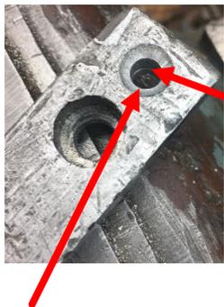
Take the drill you want to use on the rivet head and drill through the end of a piece of scrap metal. I'm using aluminum here. If the tool is going to see a lot of action, you could use steel or even press in a hardened drill guide. The drill guide hole must be smaller than the diameter of the dome.
