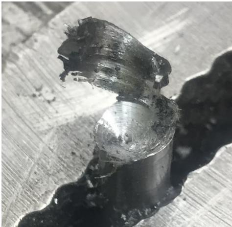
Here you see the top of the rivet almost cut off. I did have to adjust my drilling angle to stay centered but
