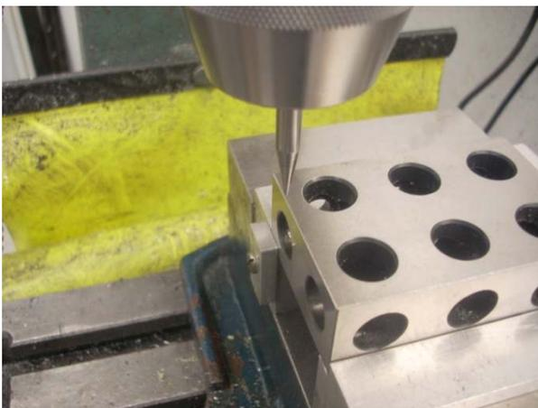
I have put a “spud” into my drill chuck as a means of locating surfaces. This is not particularly accurate but is easier to understand than if I used my Electronic Edge Finder. I'll get to the EEF later.
