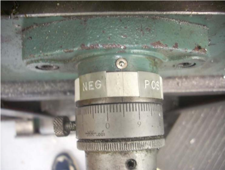
Oh yes, one more thing. I have labeled each of my axis hand cranks with a “POS” and “NEG” rotational direction in hopes of minimizing the number of times I move the cutter in the wrong direction and spoil my project. It has saved me a few times.
