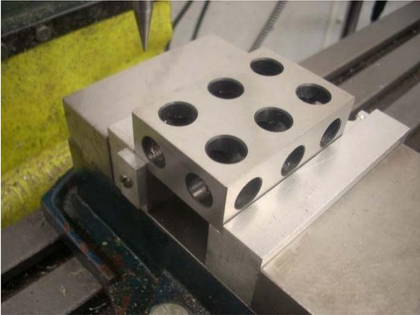
After cleaning off all mating surfaces, I have clamped a precision 1-2-3 block into my vise. This is for instructional purposes only. I have no intension of touching this hardened block with a cutter.
