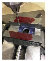
I put some Dykem on the tops of the jaws and scribed lines that aligned with the inside edges of the ways. It made it easy to line up the part so my drill bit would miss the ways.
