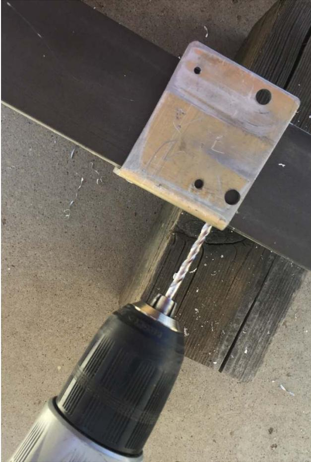
I line up the right edge of the drill guide with my tick mark. Then with the guide contacting both the top and side face, I start to drill the hole.
