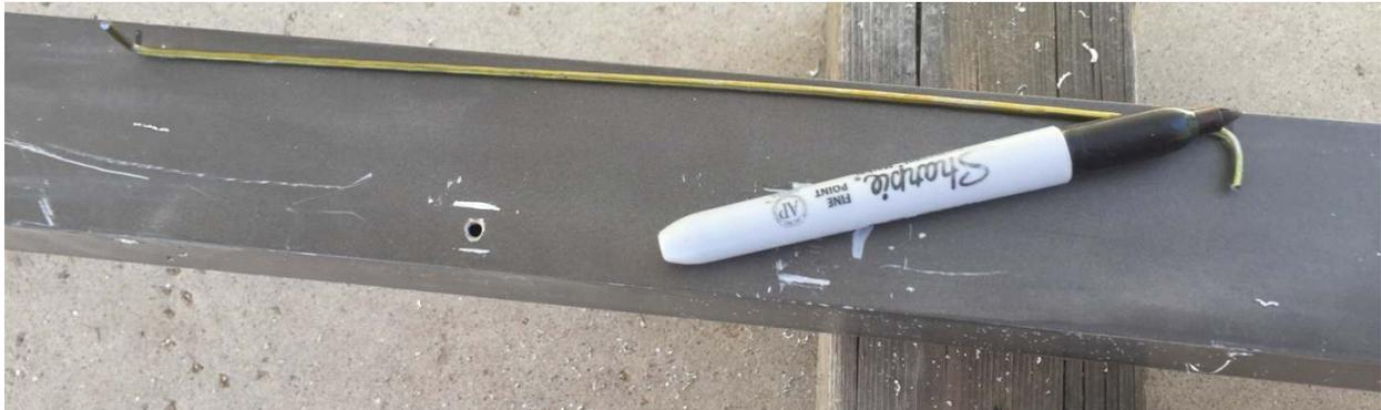
The first tool is a length of coat hanger. The ends are bent such that the corners are 8 inches apart. I mark the location of my first hole and then use this tool to mark the next hole. Moving down the tube, I can mark each locations in less 2 seconds. These holes were let me pass a length of stainless steel wire through in order to secure 4 strands of LED rope lights. The distance between holes is not that critical and it doesn't matter that there will be accumulated error.
