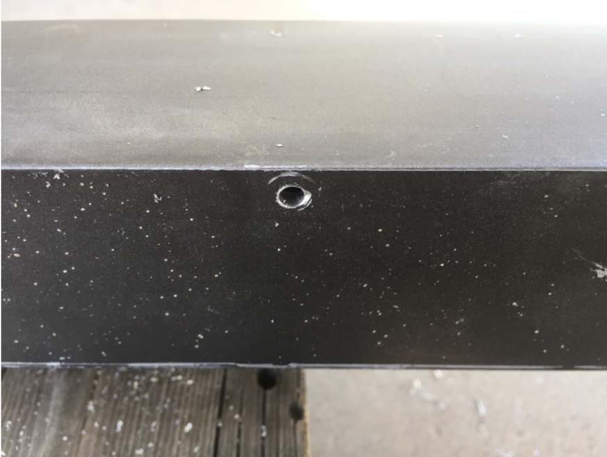
The finished hole is located just below the top face's inside surface.
