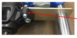
With the plate on the pillar and the large screw securely in place, use the plastic flange to guide a drill into the plate. Select a drill bit that is a close fit to the plastic hole. You only need to drill in enough to cut a cone. Then remove the plate and finish drilling the hole. This is much
