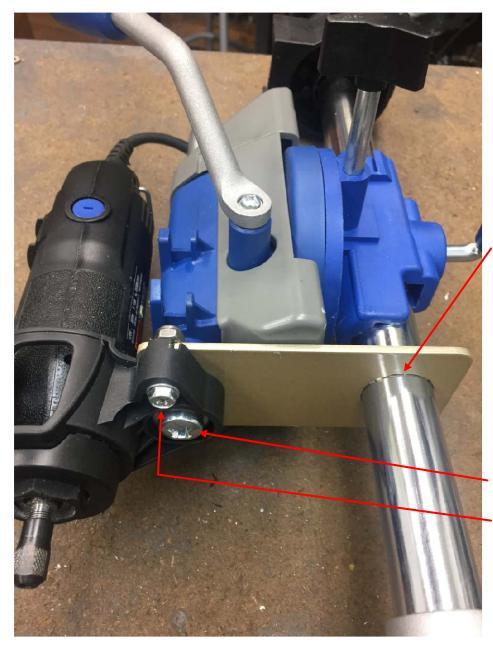
My solution was to increase the distance from the center of ram to the point that stops the rotation. This was done by fabricating a plate from  $1/8" \times 1 \frac{1}{2}"$ aluminum plate. One end was step drilled<sup>2</sup> out to 1". It is a sliding fit on the pillar.
