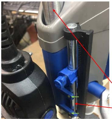
The Dremel drillpress is made mostly of steel and plastic. This is great for meeting a price point and, according to ratings I see on line, satisfies many users. But if you are trying to drill holes for a circuit board, it is a different matter. The side to side play (pivoting) of the spindle of the Dremel tool easily snaps off those tiny drill bits.
