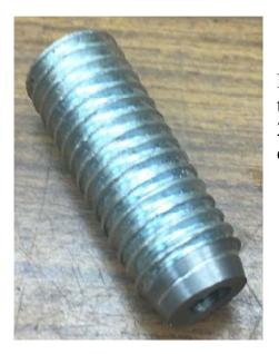
My answer was to use a 1-1/2" long piece of  $\frac{1}{2}$ "-13 threaded rod. A #7 hole was drilled through it and  $\frac{1}{4}$ -20 threads cut about  $\frac{1}{2}$ " in from one end. The other end was beveled for easy insertion.
