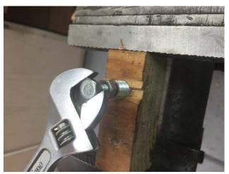
Using a wrench, I backed off the nut and then the bolt. The insert remained in the stud.
