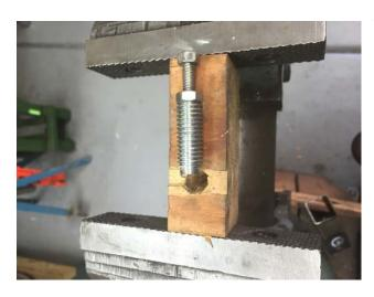
You can then turn the bolt and back the fastener out of the hole.
