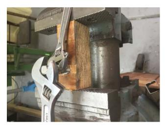
To remove the insert, screw the bolt with nut back into the fastener. Take care not to bottom out the bolt in the threaded hole.
