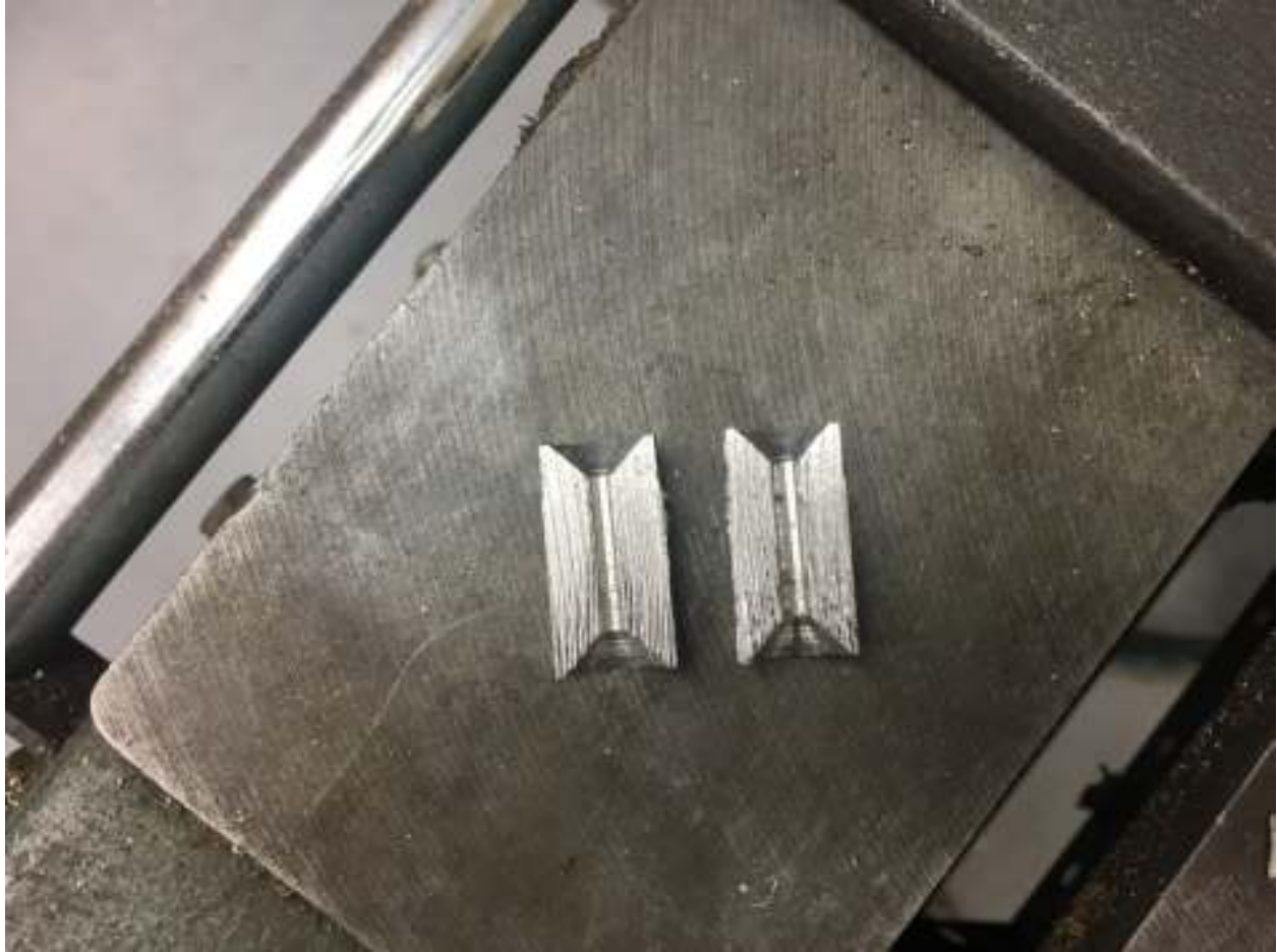
The parts look identical which means the cut was about centered.
