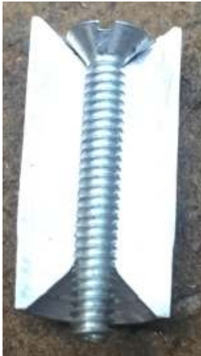
And finally, sand and/or file the rough cut faces. Then I had one gage for myself and another for a friend.
