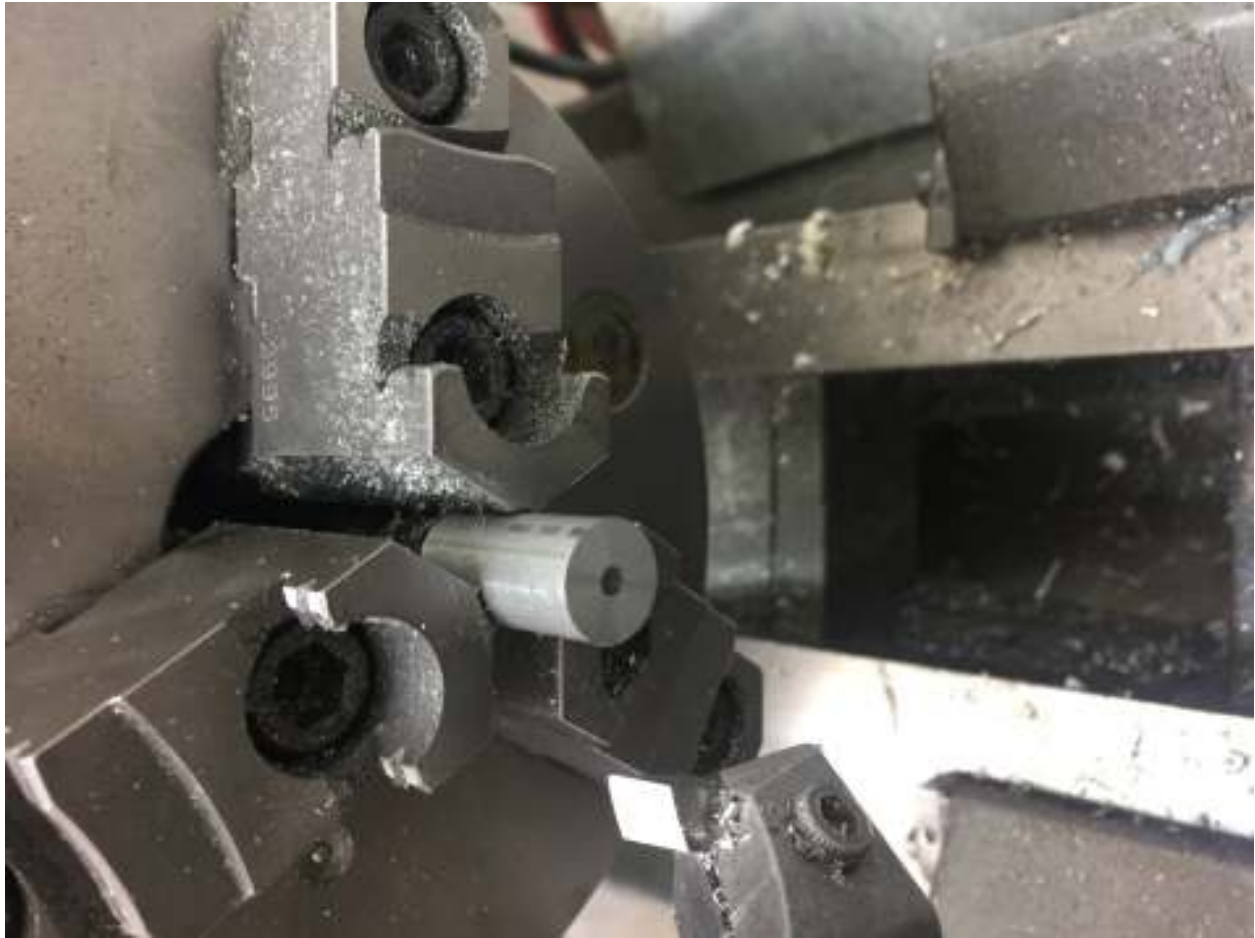
Using the left hand cutter, I faced the second end.
