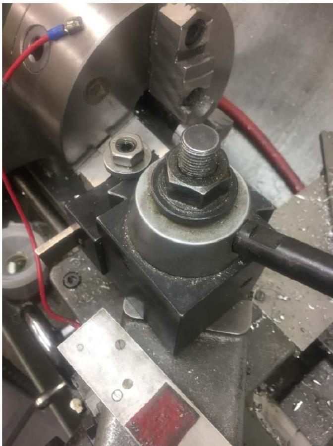
I measured TIR by using my parting tool as a probe. My Electronic Edge Finder<sup>3</sup> told me when the tool contacted the dowel pin. I took readings at 0°, 120°, and 240°. The crossfeed dial told me movement. Then I checked at 60°, 180°, and 300° to verify I had found maximum and minimum.
