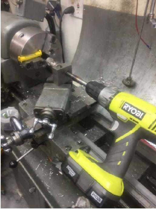
The breakthrough in making the 3 perimeter holes at the same distance from the center was to use my compound mounted drill chuck. I used a line level to set the angle.
