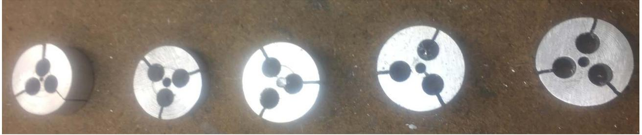
I have been able to get a Total Indicated Runout (TIR) of less than a thou with this collet but it took a bit of doing. Here are most of my attempts. After each one, I measured the TIR, determined the root cause of the poor performance, and then figured out how to avoid the problem on my next attempt.
