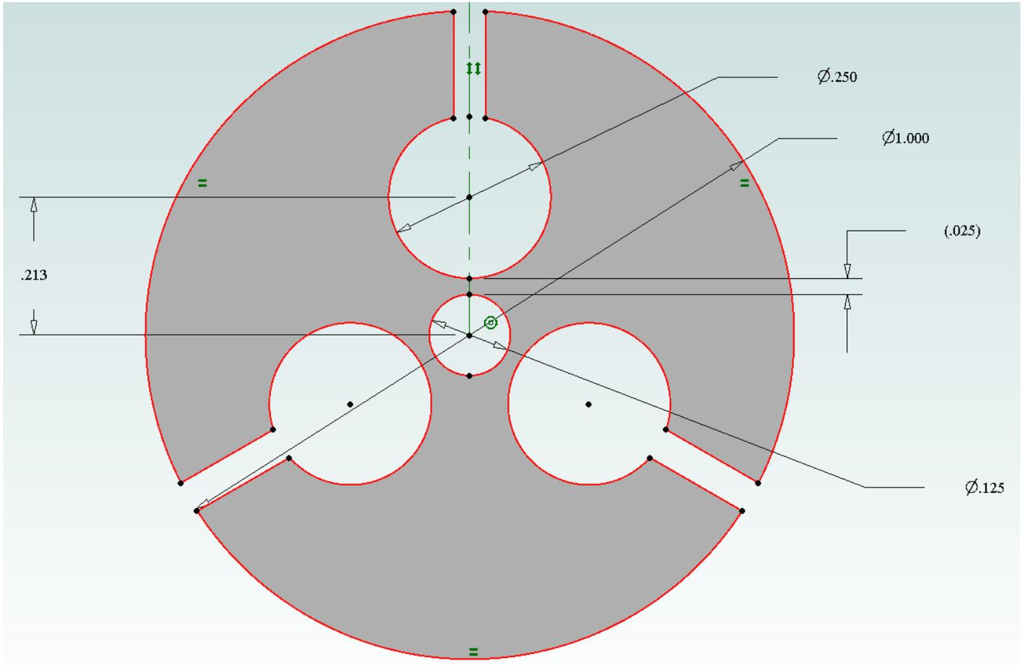
Here is my test crush collet. I used a 1/8" center hole so I could fit it with a 1/8" dowel pin in order to accurately measure TIR. I chose a wall thickness of 0.025" between the nominal position of the center hole and perimeter holes.
