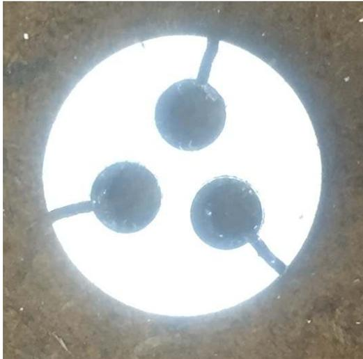
Next I removed the part and drilled through using a 1/4" drill on the drill press. The 3 cuts were made on my bandsaw. It is essential that the saw not slip and cut the far side of any hole. I spoiled one part that way. This caused excessive TIR.
