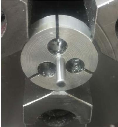
My 1/8" dowel pin smoothly slid into the hole. Then when I tightened down on the chuck, the pin was solidly locked in place.
