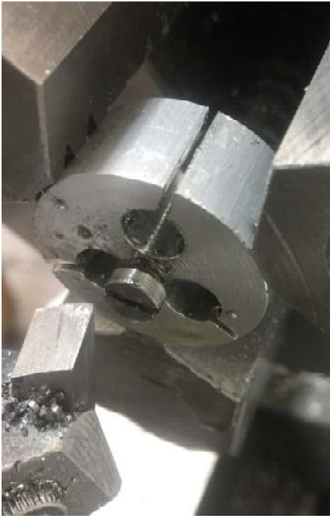
Although my test collets have a smooth hole in them, the real value is when the hole is tapped. It then becomes possible to hold threaded stock like small brass screws without causing damage. Here I have machined the head of an 8-32 screw. It started out with a round head. I saw no unscrewing while machining.
