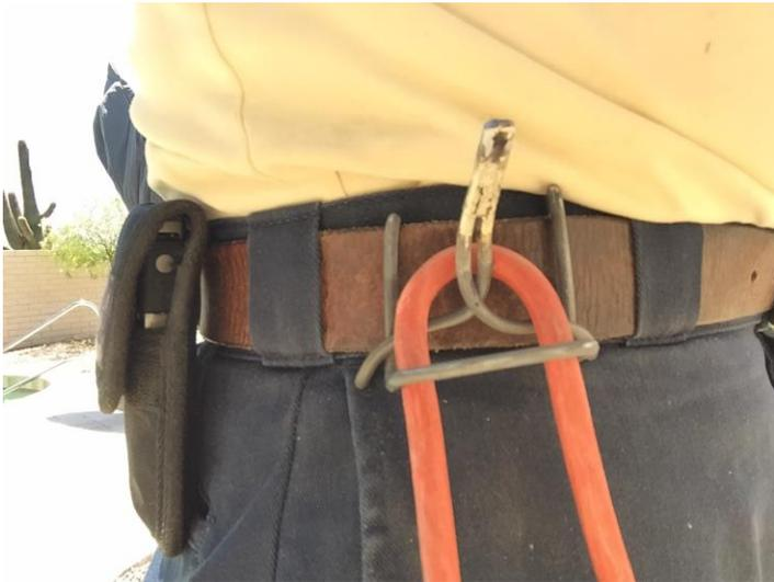
Then I got thinking about the cable relief on my edger. It forced too tight a bend in the cable but the idea was good. I have taken that basic idea, increased the loop radius, and now have a useful, if not geeky, solution.
