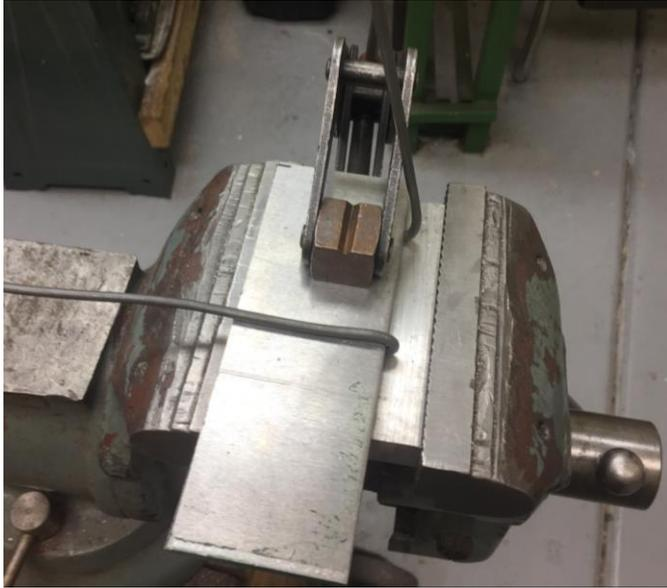
To finish the bends, I clamped down a 3/16 inch by 2 inch bar. Then I used my hammer to flatten it down. After bending one wire, I moved the clamp and bent the other wire.
