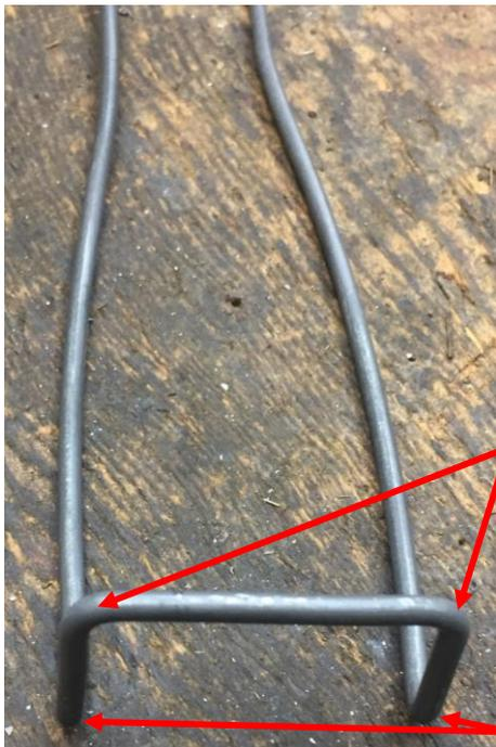
I started with 3 feet of 1/8" CRS wire. Finding the center, I marked a line 1 inch on each side. Using my bench vise and a large ball peened hammer,
