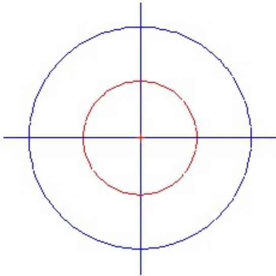
If you placed a DTI on the red circle in the ideal case, the reading would be constant as the circle turned. When I get this result in my less than ideal world, it usually means the DTI is broken, hitting a stop, or not touching the circle.
