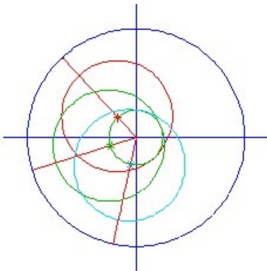
Here is where it gets a bit messy. As I turn the blue circle with the red circle resting on it, note how the red circle turns. The original location of the red circle is shown with its red center point. Below it is this same circle but with the blue circle turned a bit counterclockwise. I changed the color to green. Below it is again the same circle but move a little further and in turquoise. As I turn the blue circle, the center of
