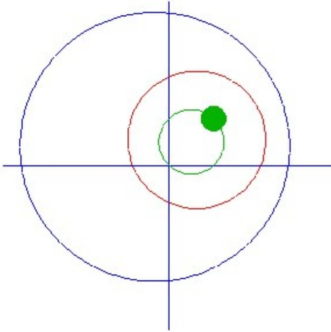
As I rotate the body of the EEF represented by the red circle, the pin will trace out the path marked by the green circle. Note that there is a point on the green circle that lines up with the center of rotation. By turning the body of the EEF we can place its pin's center at the center of rotation and achieve zero TIR. We would then have a misaligned spindle holding a misaligned EEF with its pin perfectly aligned. I guess you could say that in this instance,
