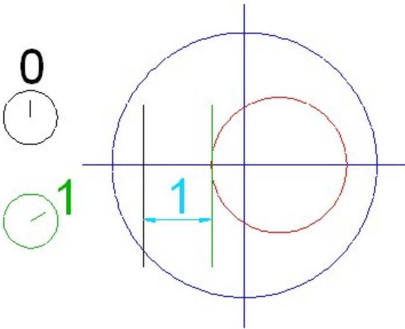
Now rotate the blue circle 180 degrees. The red circle will again have its center on the same line as the blue circle's center and the DTI's spot. The DTI will now read a minimum.
