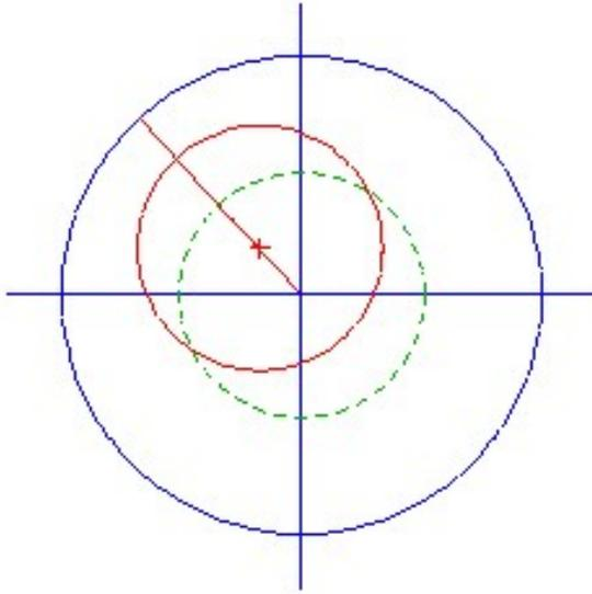
Look what happens if the red circle's center is not aligned with the center of the blue circle. The dashed green circle is its previous, ideal location and the red circle is the new location. The center of the red circle is marked with a red X. I can always draw a line from the center of the blue circle, through the center of the red circle, and out to the blue circle. This line will always be a radius.
