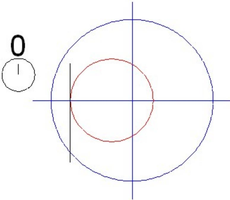
Anyway, say the red circle is not centered. I can rotate the blue circle until the DTI reads a maximum. This must be the point where the center of the blue circle is on the same line as the center of the red circle. Say I set the DTI to read 0.
