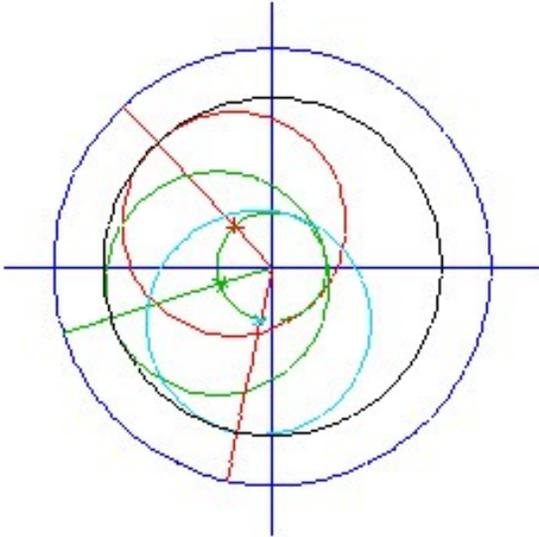
Time for a diversion to the practical. Say the blue line represents the spindle of a vertical mill as viewed by looking up. The red circle represents an end mill. A *really* bad collet holds the end mill so it turns way off center.
